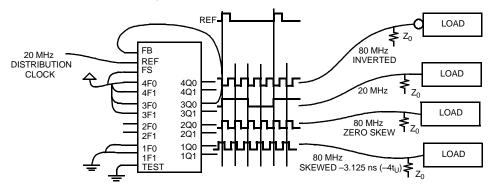
Figure 9. Board-to-Board Clock Distribution
