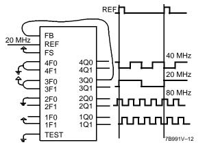
Figure 6 shows the LVPSCB configured as a clock multiplier. The 3Q0 output is programmed to divide by four and is sent back to FB. This causes the PLL to increase its frequency until the 3Q0 and 3Q1 outputs are locked at 20 MHz, while the 1Qx and 2Qx outputs run at 80 MHz. The 4Q0 and 4Q1 outputs are programmed to divide by two that results in a 40 MHz waveform at these outputs. Note that the 20- and 40-MHz clocks fall
