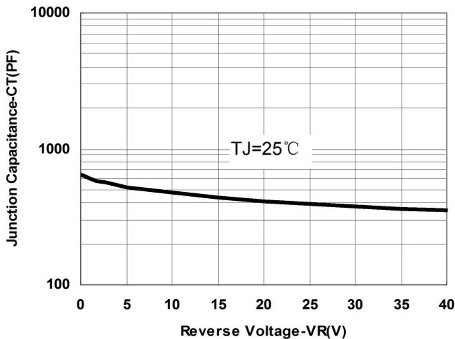
Fig.1-Typical Junction Capacitance
