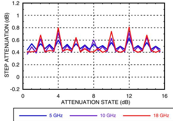
**Step Attenuation vs. Attenuation State**
