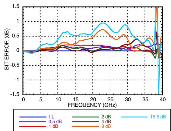
**0.5 dB LSB GaAs MMIC 5-BIT DIGITAL ATTENUATOR, 0.1 - 33 GHz**
