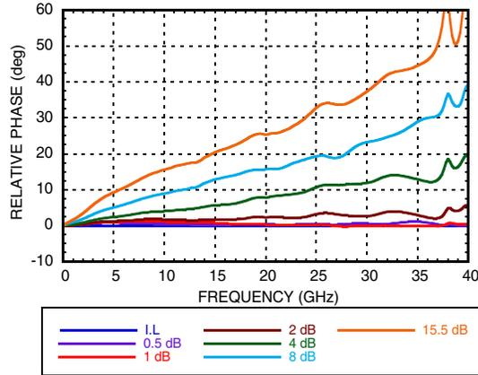
**Step Attenuation vs. Attenuation State**
