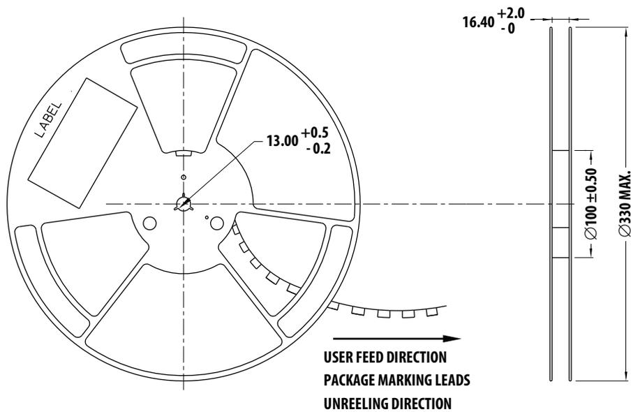
NOTE: All dimensions in millimeters (mm).
