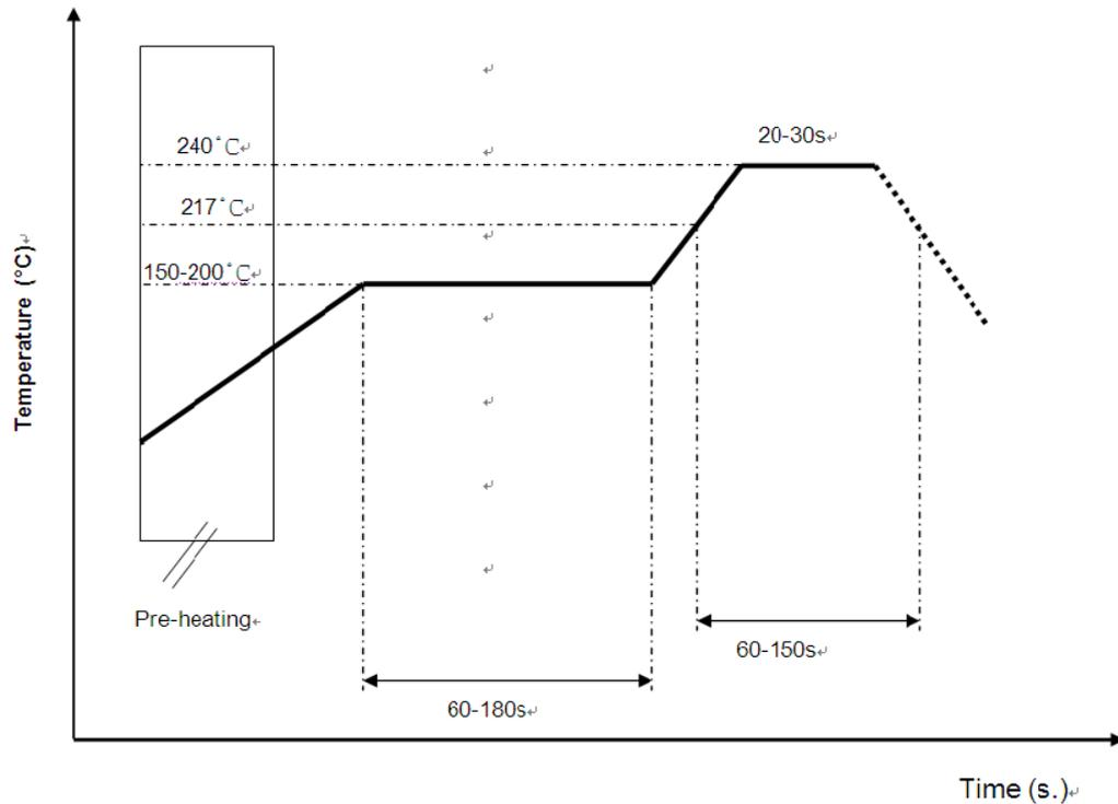
\*Recommended solder paste alloy: SAC305 (Sn96.5 /Ag3 /Cu0.5) Lead Free solder paste.
