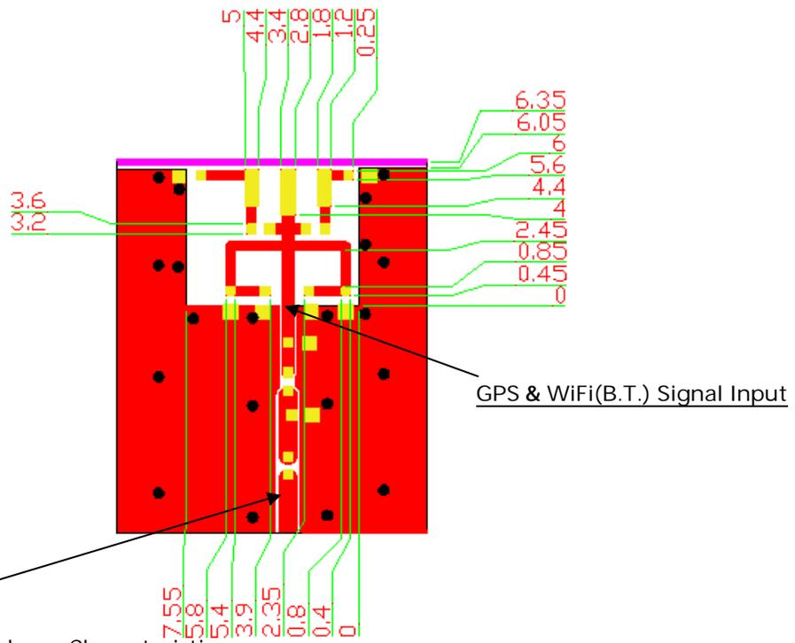
Transmission Line with 50Ω Impedance Characteristic
