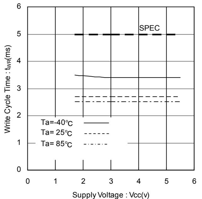
Figure 27. Write Cycle Time vs Supply Voltage
