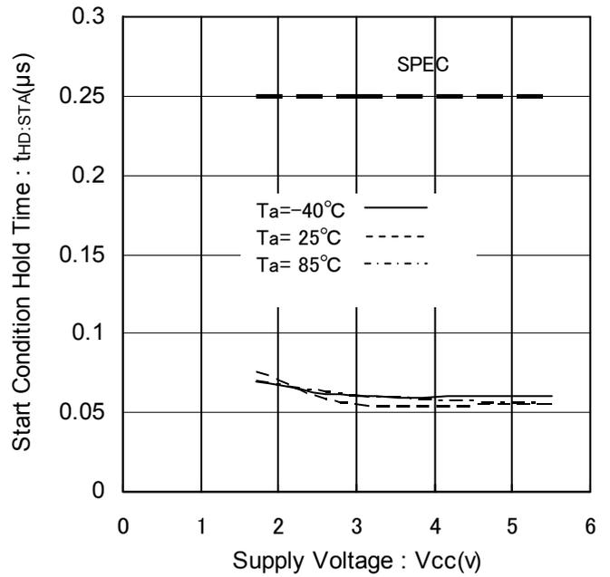
Figure 17. Start Condition Hold Time vs Supply Voltage
