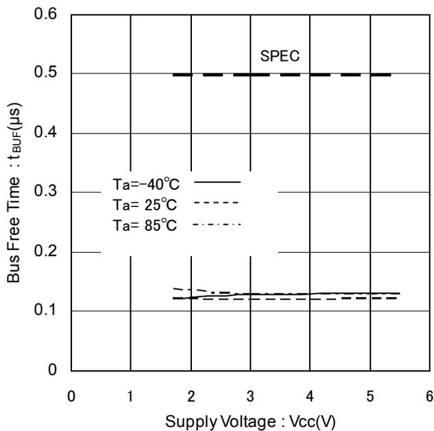
Figure 26. Bus Free Time vs Supply Voltage
