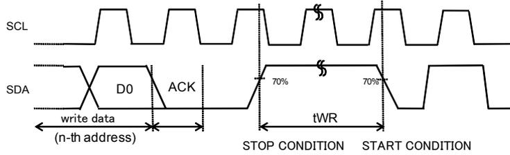
Figure 2-(c). Write Cycle Timing
