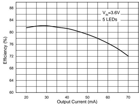
**Performance Characteristics** (continued) (The WLED forward voltage ( $V_F$ ) is 3.45V at  $I_F = 20\text{mA}$ , unless otherwise noted.)
