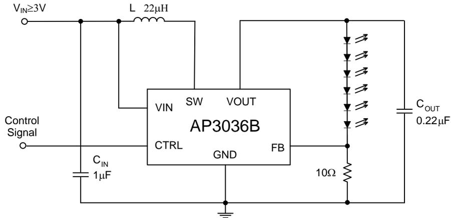
Note: 4. C: X5R or X7R type dielectric, L: SUMIDA CDRH5D28R-220NC or equivalent. And, this circuit can work in full temperature.
