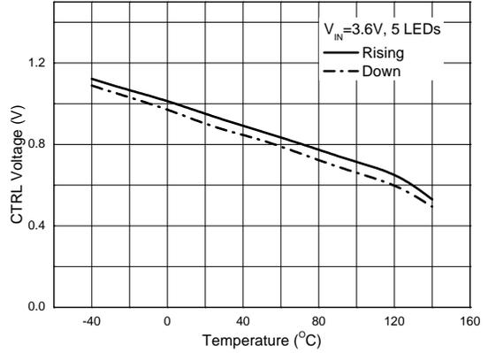
**OVP Voltage vs. Temperature**
