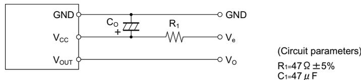
In setting  $R_1$  and  $C_1$ , use suitable values after considering under the real condition
