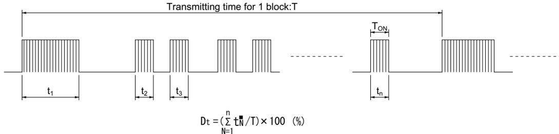
In case the signal format of total duty and/or ON/OFF signal time doesn't meet the conditions noted above, there is a case that reception distance much reduces or output dose not appear.
