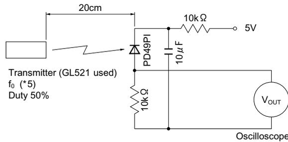
In the above figure, the transmitter should be set so that the output  $V_{OUT}$  (P-P) can be 40mV. However, the PD49PI to be used here should be of the short-circuit current  $I_{SC}=2.6 \mu A$  at  $E_v = 100$  lx. ( $E_v$  is an illuminance by CIE standard light source A (tungsten lamp).)
