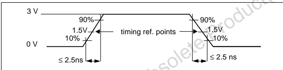
Figure 8 Input waveforms
