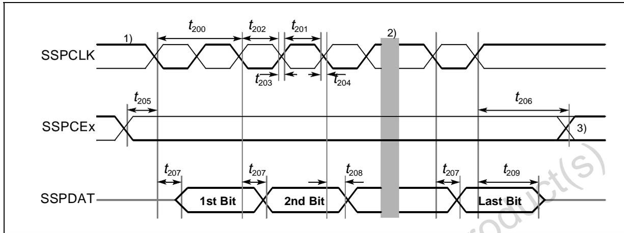
Figure 26 SSP write timing
