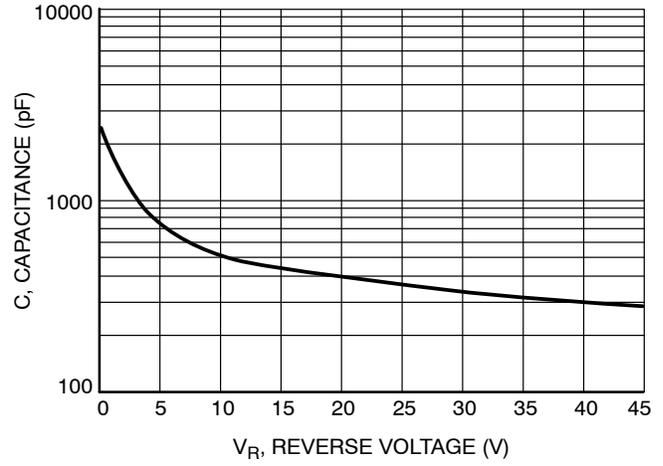
Figure 7. Typical Capacitance
