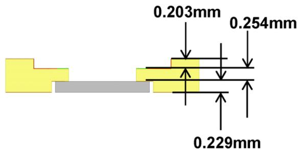
Fig. 3. CQFN 24-Pin Package Drawing (All Dimensions in mm)
