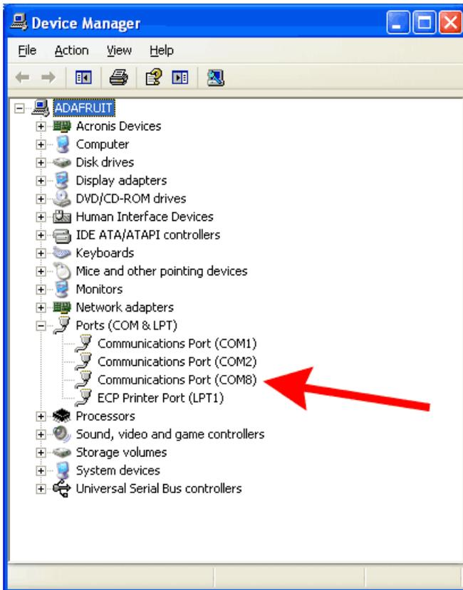
For mac/linux, once you have plugged in the cable, run **dmesg** to see what the name of the port is, probably something like **/dev/cu.usbmodem-XXXX** or similar. You can also type **ls /dev/cu.\*** into a **Terminal** window and see what items appear/disappear when the cable is connected and unplugged.
