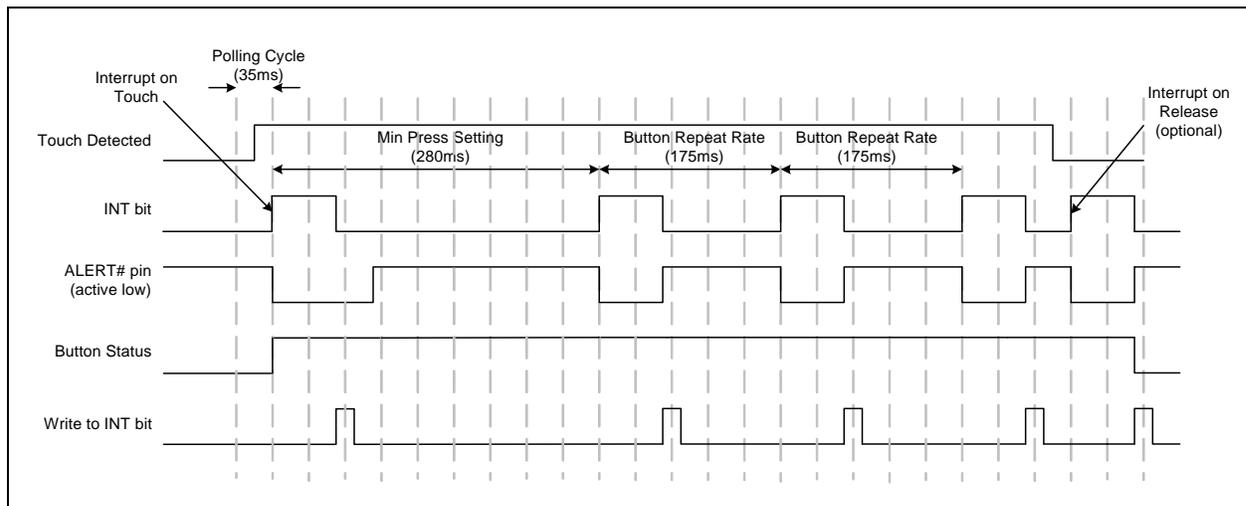
**FIGURE 5-3:** Sensor Interrupt Behavior - No Repeat Rate Enabled
