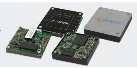
Advanced Energy's Artesyn AVE450/500 series half-brick isolated DC-DC converter provides a single regulated low noise output, 28 Vdc that can deliver up to 16 amps (AVE450B-48S28) or 50V that can deliver up to 10 amps (AVE500-48S50). It has a wide 2:1 input range of 36 to 75 Vdc and is designed primarily for use with standard 48 V telecommunications equipment supplies. The converter's main application area is in low power and remote radio head (RRH) telecommunications applications.
