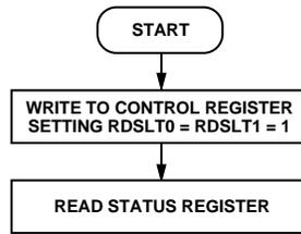
Figure 6. Flowchart for Reading the Status Register
