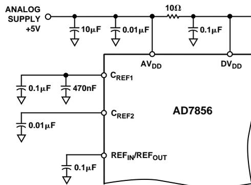
Figure 16. Relevant Connections When Using Internal Reference
