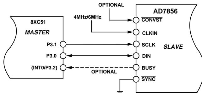
Figure 37. 8XC51/PIC16C42 Interface
