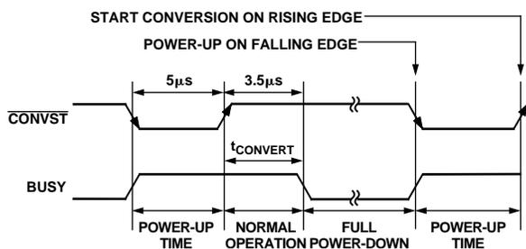
Figure 22. Power-Up Timing When Using  $\overline{\text{CONVST}}$  Pin
