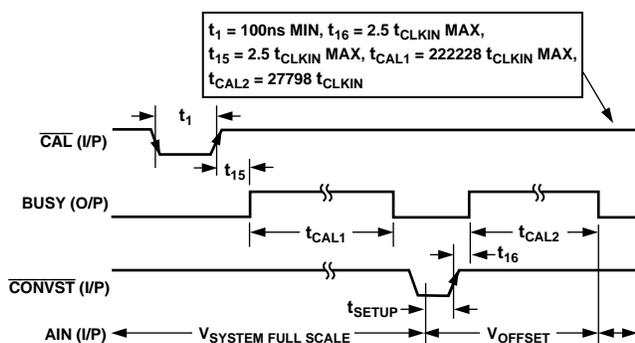
Figure 29. Timing Diagram for Full System Calibration
