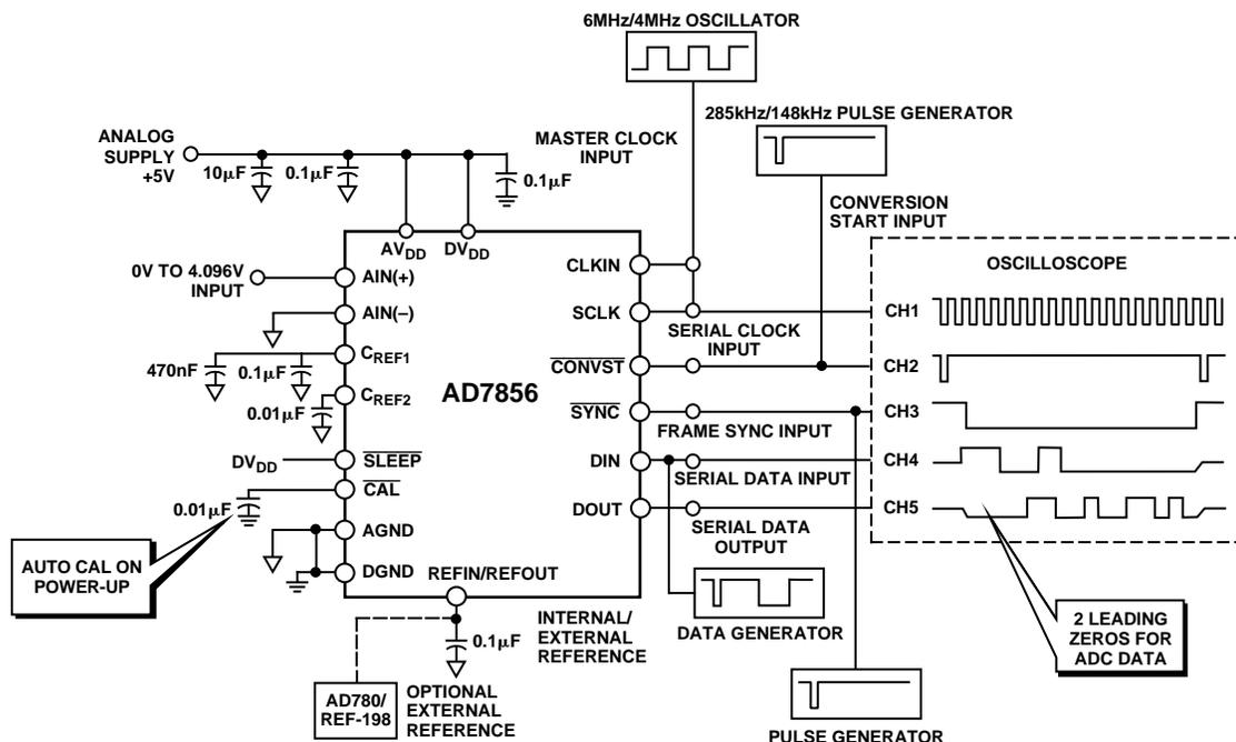
Figure 10. Typical Circuit
