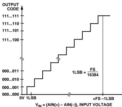
Figure 15. Transfer Characteristic
