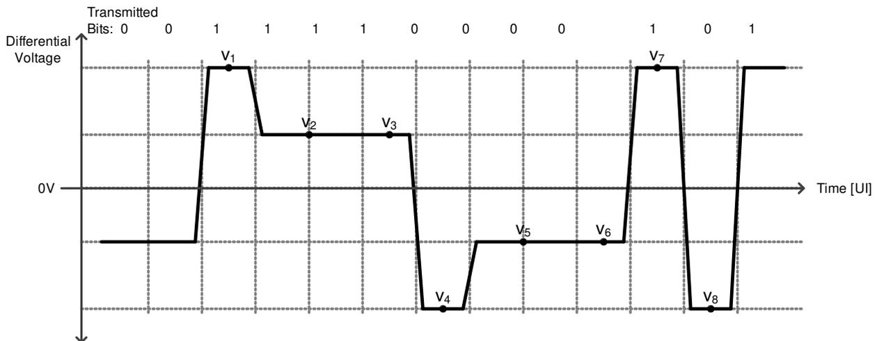
Figure 8. Conceptual FIR Waveform With Postcursor Only
