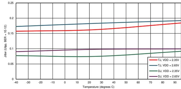
Figure 4. Typical Output Jitter vs Temperature at 25.78125 Gbps
