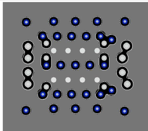
Figure 27. VDD Layer (Pin A1 is Top-Left)
