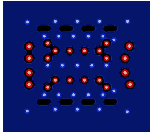
Figure 25. Layer 1 GND (Pin A1 is Top-Left)
