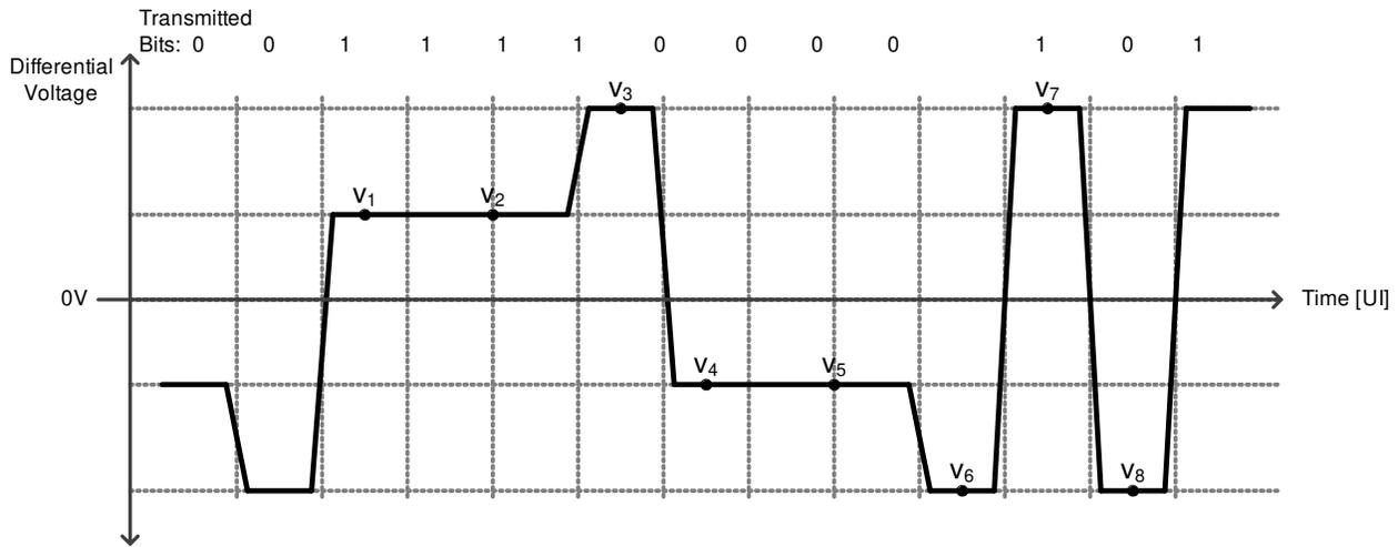
Figure 9. Conceptual FIR Waveform With Precursor Only
