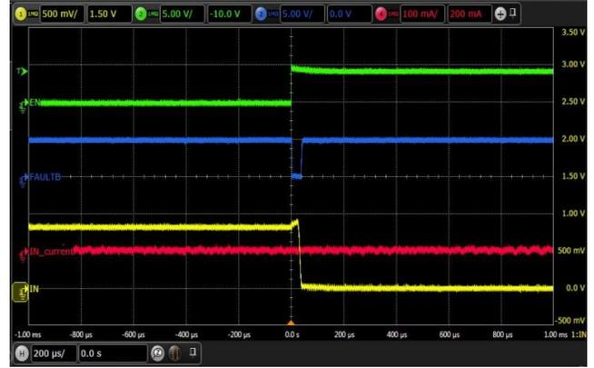
$V_{CC} = EN = 5\text{V}$ , IN\_Current = 0A to 10A (IN Initial = 0V)
