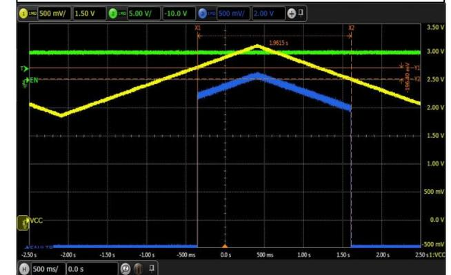
$V_{CC} = EN = 5\text{V}$ , IN = 0V Hard Short to 12V
