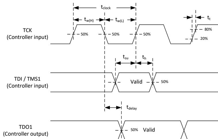
**Figure 6-19. Timing Diagram for JTAG Boundary Scan**
