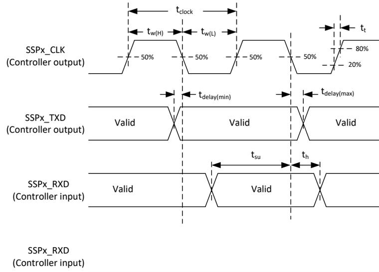
**Figure 6-18. Timing Diagram for SSP Master (Modes 0/3)**
