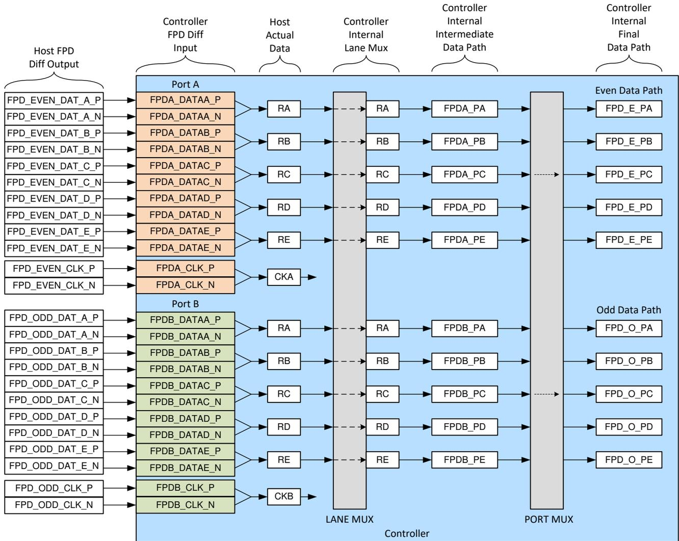
**Figure 7-2. Example of Typical FPD-Link Port Lane Mapping**
