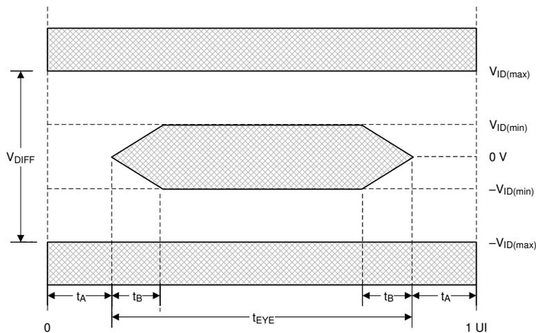
Figure 6-12. V-by-One Timing
