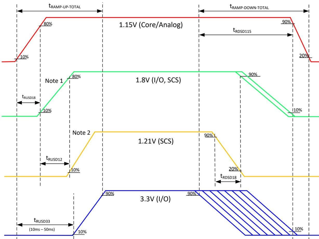
Note 1: No power up or power down timing dependency between 1.8V and 3.3V
