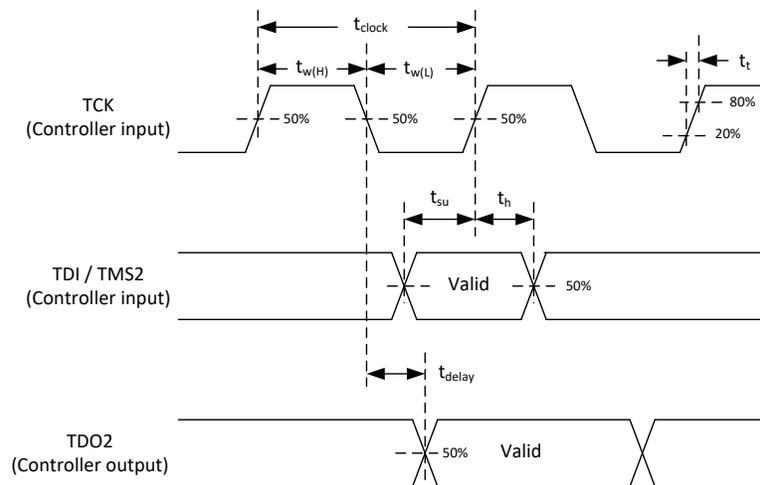
**Figure 6-20. Timing Diagram for JTAG ARM Multi-Ice**
