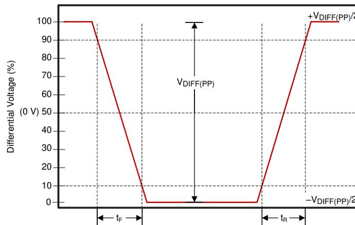
V<sub>CM</sub> is removed when signals are viewed differentially
