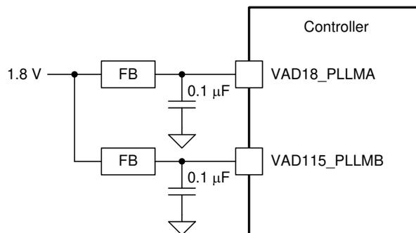
**Figure 10-8. 1.8-V PLL Power Supply Filter Topology**
