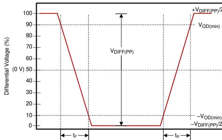
$V_{CM}$  is removed when signals are viewed differentially
