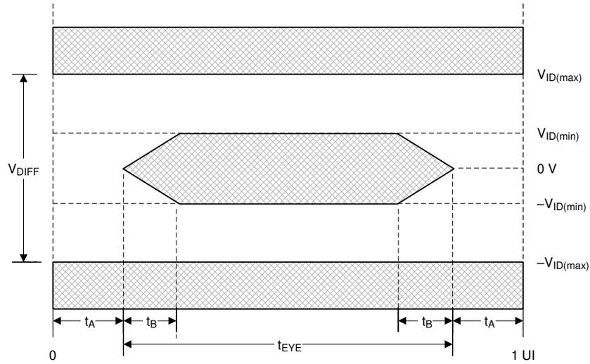
Figure 6-14. FPD-Link Timing
