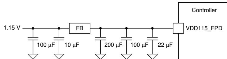
**Figure 10-3. VAD115\_FPD (FPD-Link) Recommended Filter**
