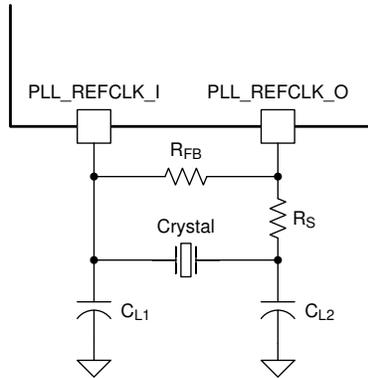
$C_L$  = Crystal load capacitance
