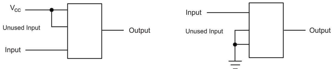
Figure 35. Layout Diagram
