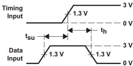
Figure 25. Voltage Waveforms Setup and Hold Times
