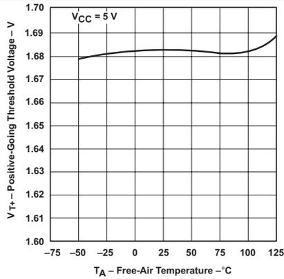
Figure 1. Positive-Going Threshold Voltage vs Free-Air Temperature
