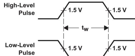
Figure 17. Voltage Waveforms Pulse Durations
