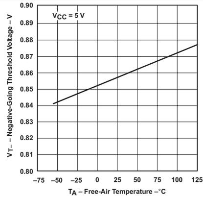
Figure 2. Negative-Going Threshold Voltage vs Free-Air Temperature
