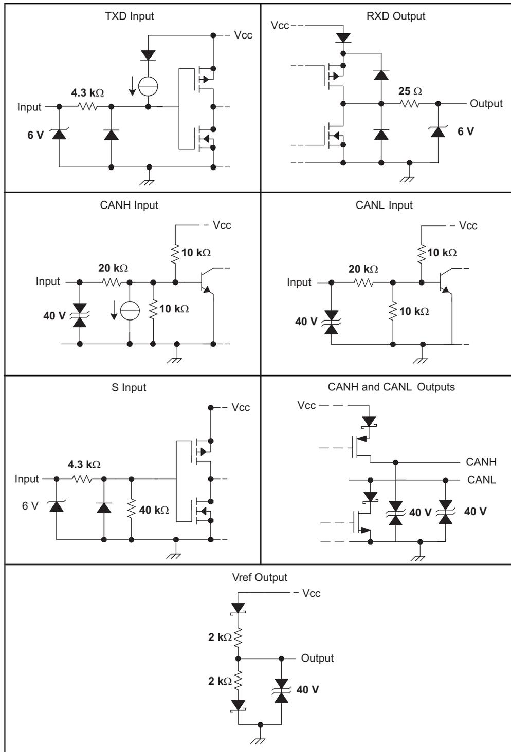
Figure 22. Equivalent Input and Output Schematic Diagrams
