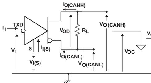
Figure 11. Driver Voltage, Current, and Test Definition
