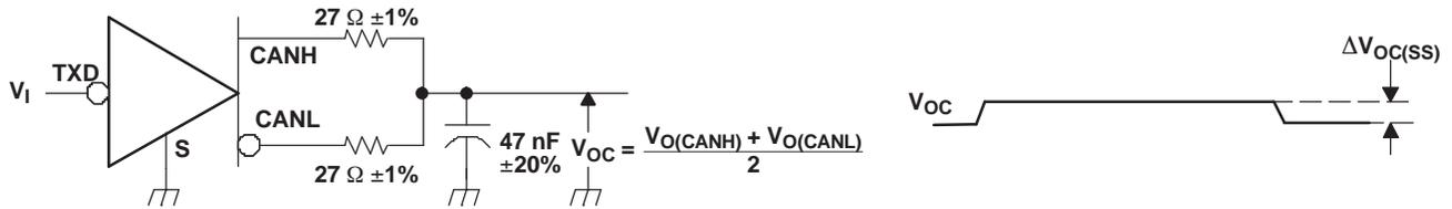
NOTE: All  $V_I$  input pulses are from 0V to  $V_{CC}$  and supplied by a generator having the following characteristics:  $t_r$  or  $t_f \leq 6$  ns. Pulse Repetition Rate (PRR) = 125 kHz, 50% duty cycle.
