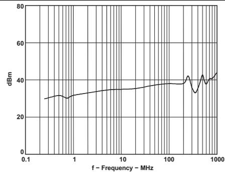
Figure 10. Direct Power Injection (DPI) Response vs Frequency
