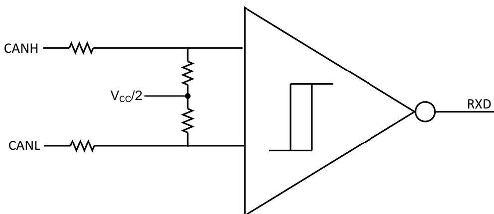
Figure 24. Simplified Recessive Common Mode Bias and Receiver
