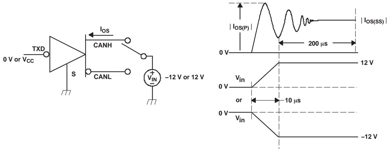
Figure 21. Driver Short-Circuit Current Test and Waveform
