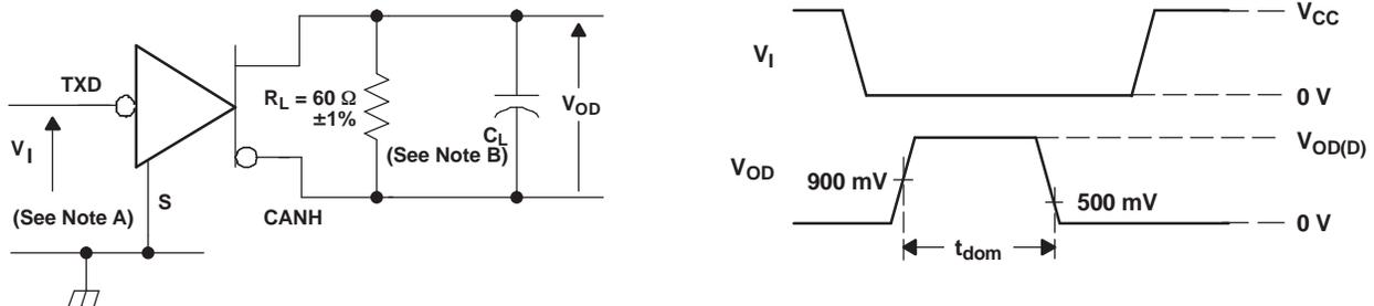
A. All  $V_I$  input pulses are from 0 V to  $V_{CC}$  and supplied by a generator having the following characteristics:  $t_r$  or  $t_f \leq 6$  ns. Pulse Repetition Rate (PRR) = 500 Hz, 50% duty cycle.
