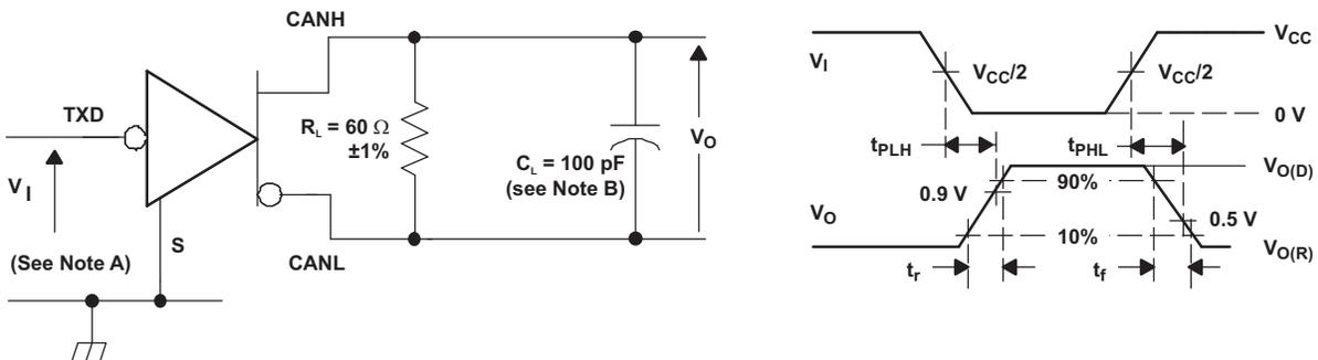
Figure 14. Driver Test Circuit and Voltage Waveforms
