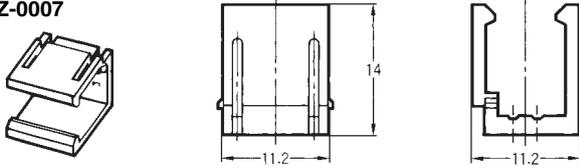
After a Plug and Socket are mated with each other, they can be locked with the XC5Z-0007 Clamping Bracket in order to improve the vibration and shock resistance of the Connector.
