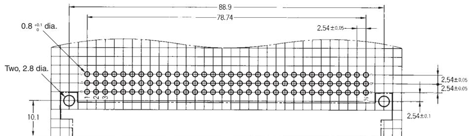
Note: The 64-contact plug does not have the center row (b in the above diagrams).
