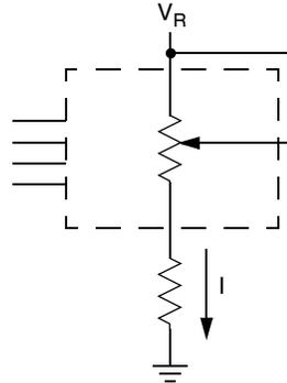
Two terminal Variable Resistor;
