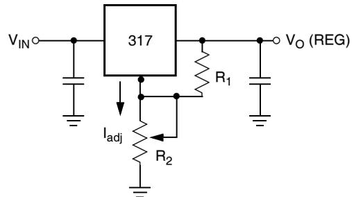
$$V_O (\text{REG}) = 1.25V (1 + R_2/R_1) + I_{\text{adj}} R_2$$
