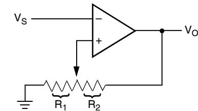
$$V_{UL} = \{R_1/(R_1 + R_2)\} V_O(\text{max})$$
