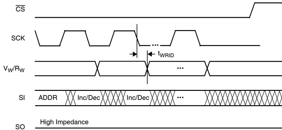
**Write Protect and Device Address Pins Timing**
