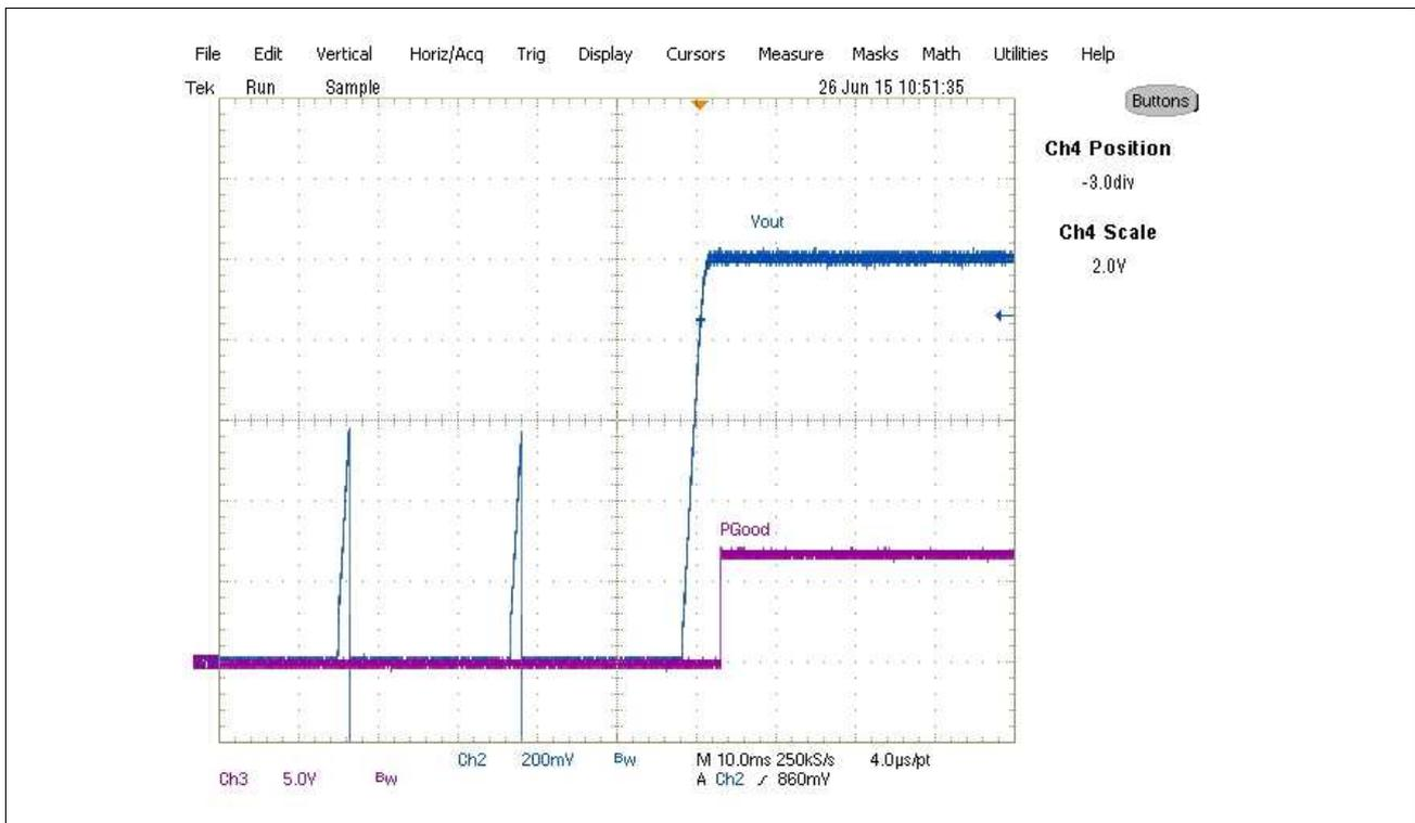
Figure 7-11 Short circuit (hiccup) recovery (Ch<sub>2</sub>:Vout, Ch<sub>3</sub>: PGood)
