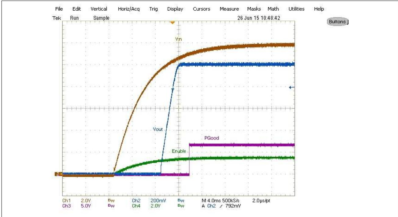
Figure 7-6 Startup at 20A Load (Ch<sub>1</sub>: $V_{in}$ , Ch<sub>2</sub>: $V_{out}$ , Ch<sub>3</sub>:  $PGood$ , Ch<sub>4</sub>: $Enable$ )
