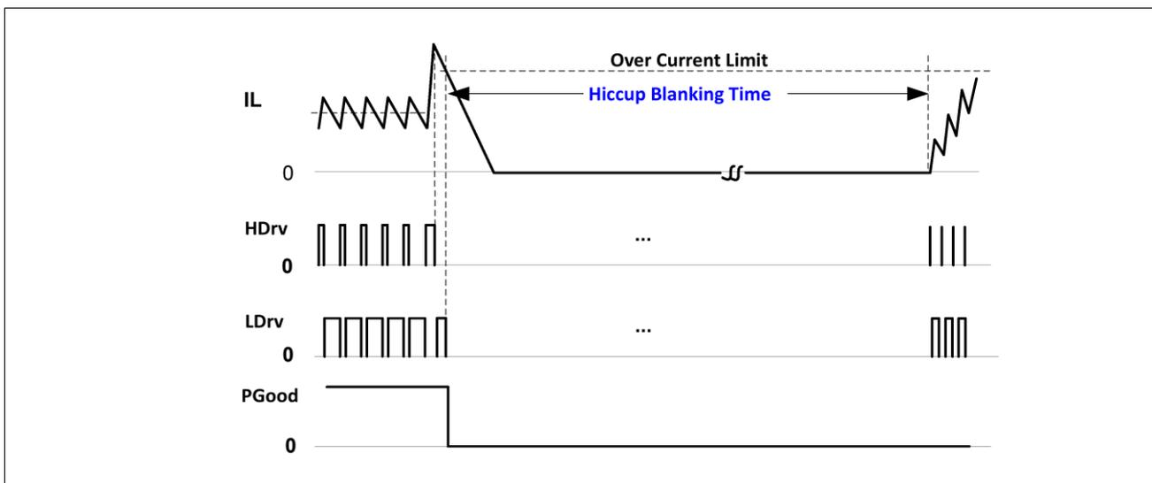
**Figure 6-7** Timing Diagram for Current Limit Hiccup
