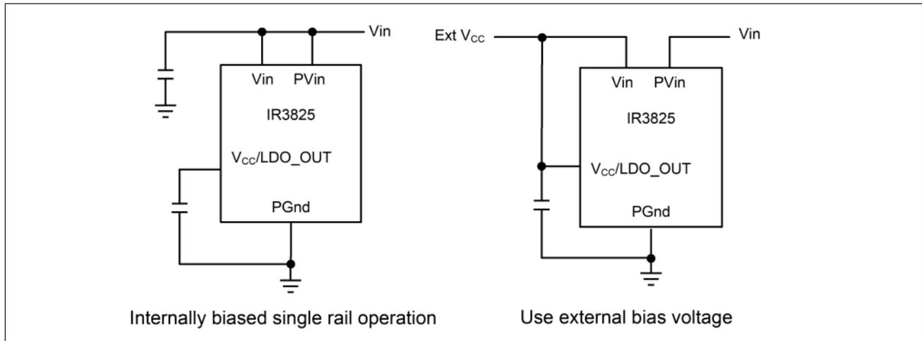
Figure 6-9 Internal LDO or External V<sub>CC</sub> Configurations
