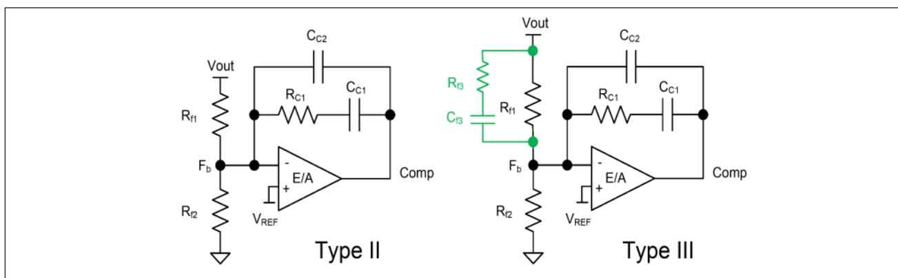
Figure 6-1 Loop Compensators
