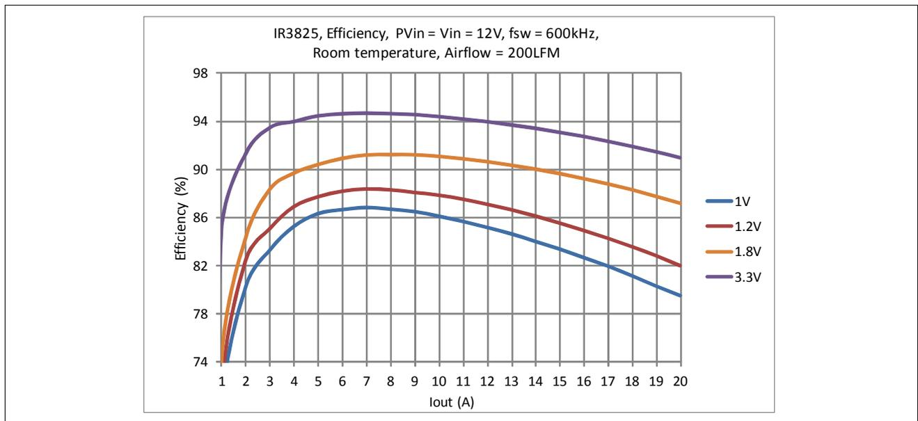
**Figure 5-1 IR3825 Efficiency Curves -  $P_{V_{in}} = V_{in} = 12V$ ,  $V_{CC} = \text{Internal LDO}$**
