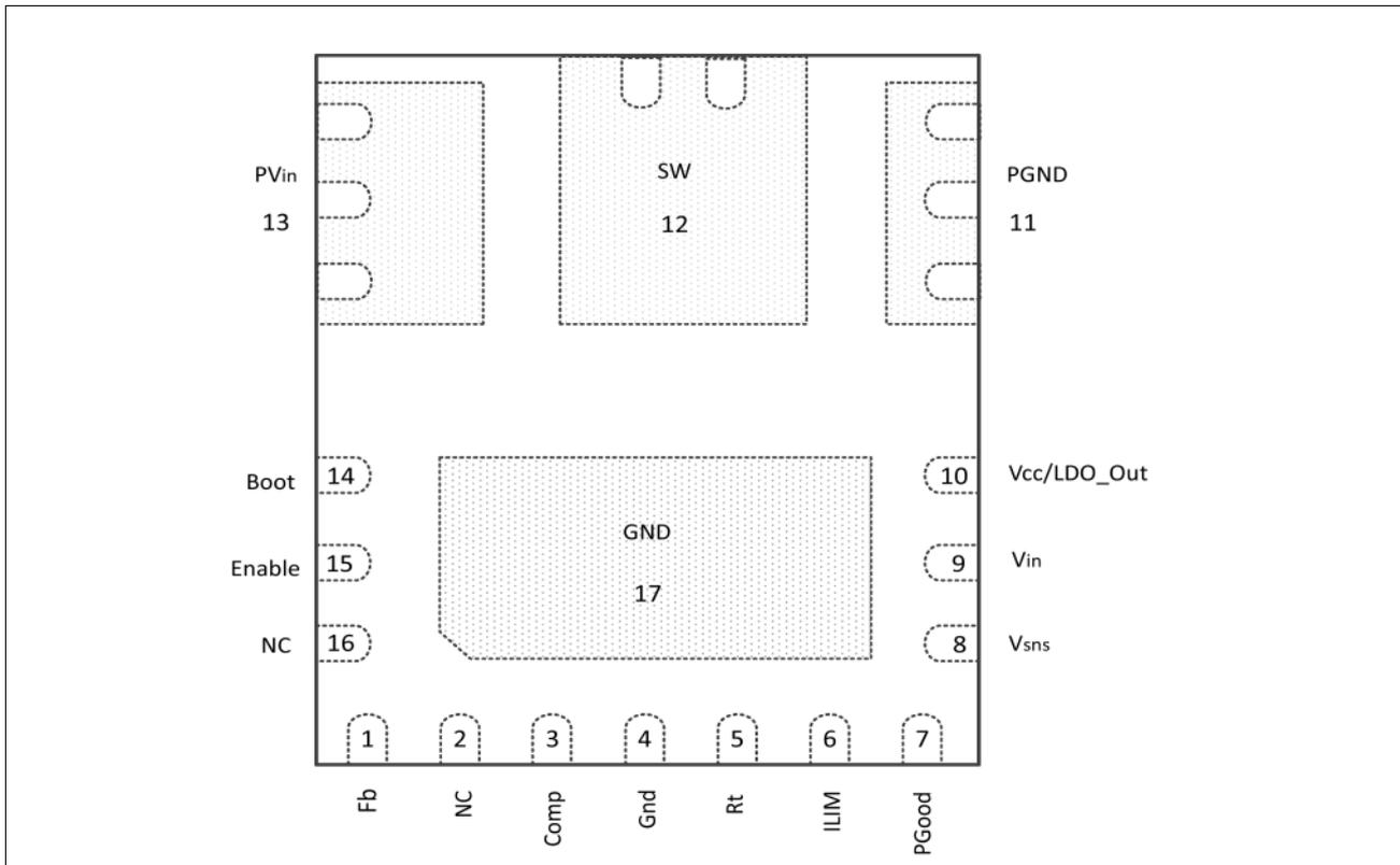
Figure 4-1 Pinout Diagram: PQFN 5 mm x 6 mm (Top View)
