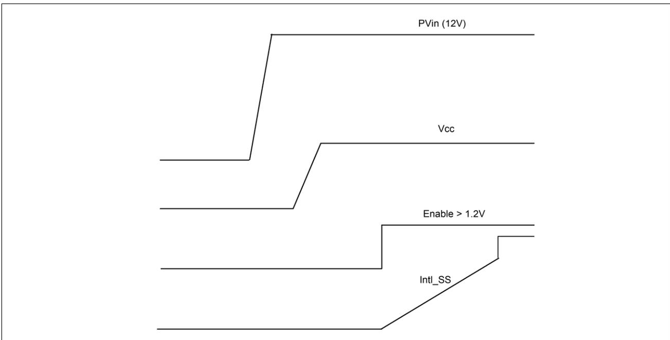
**Figure 6-3 Normal start-up with a logic input for Enable signal**
