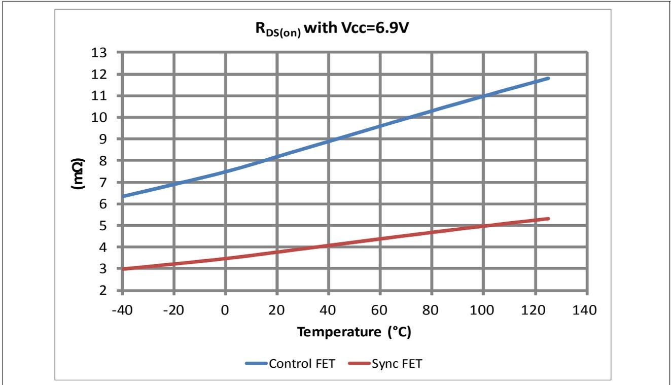
Figure 5-5  $R_{DS(on)}$  with  $V_{CC} = 6.9V$  Over Temperature
