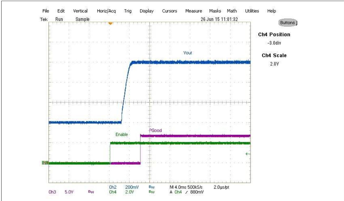
Figure 7-8 Start up with pre bias, 0A Load (Ch<sub>2</sub>:Vout, Ch<sub>3</sub>: PGood, Ch<sub>4</sub>:Enable)
