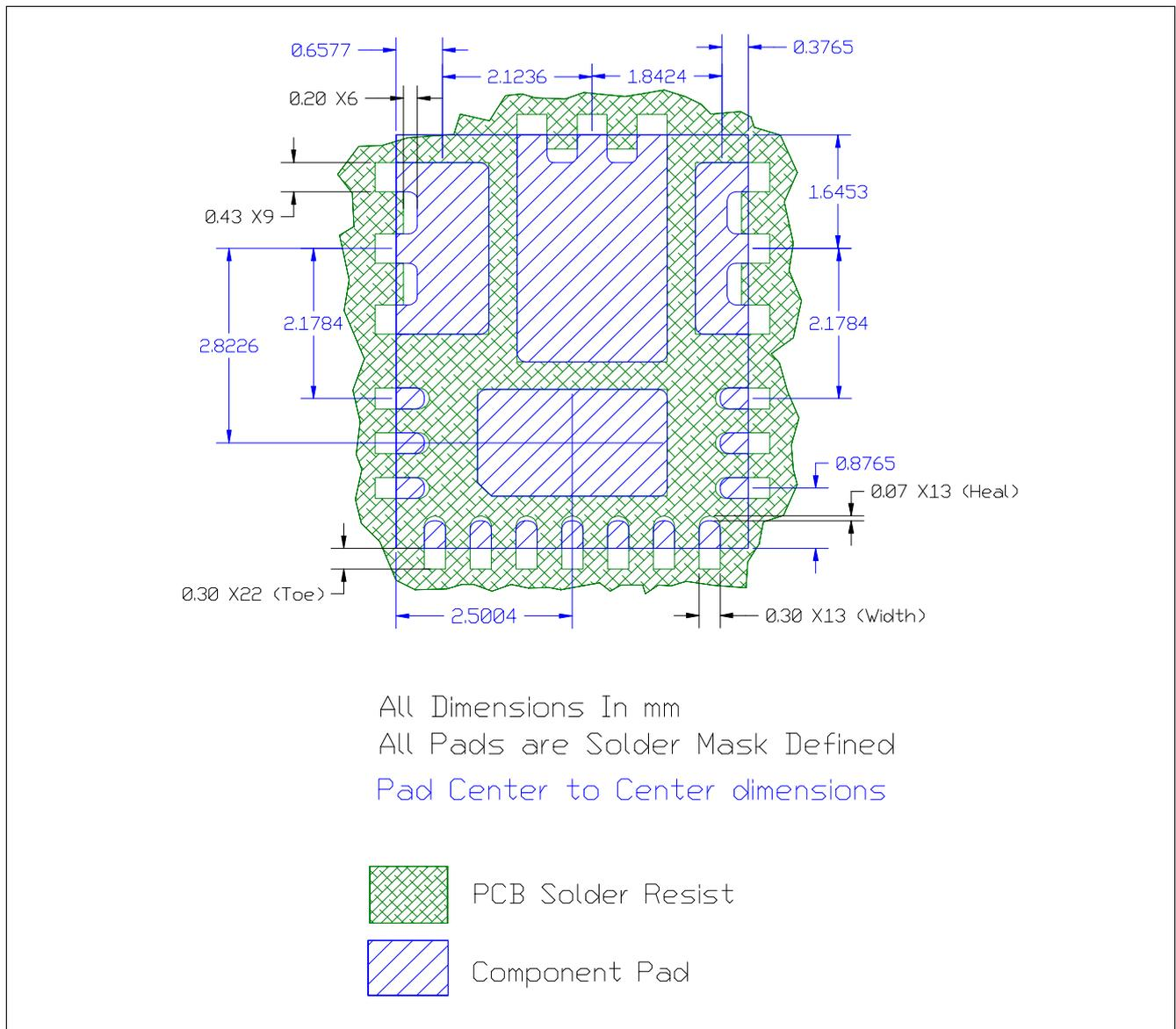
Figure 8-6 Solder Resist
