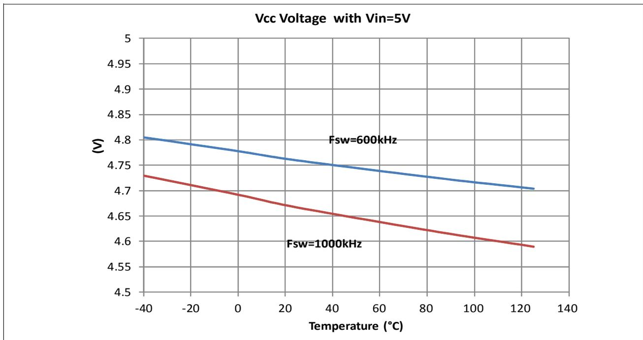
Figure 6-10 LDO Voltage with Vin = 5V
