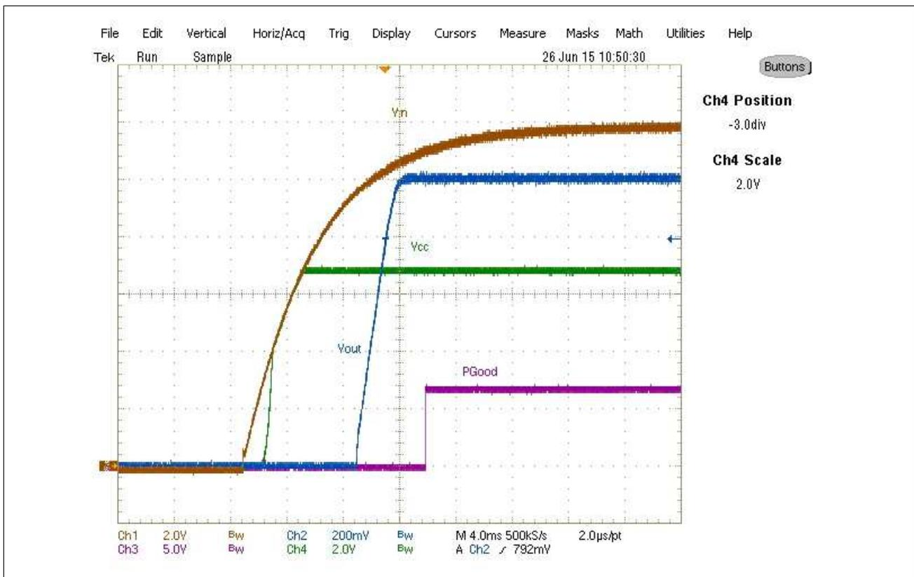
Figure 7-7 Startup at 20A Load (Ch<sub>1</sub>: $V_{in}$ , Ch<sub>2</sub>: $V_{out}$ , Ch<sub>3</sub>:  $PGood$ , Ch<sub>4</sub>: $V_{CC}$ )
