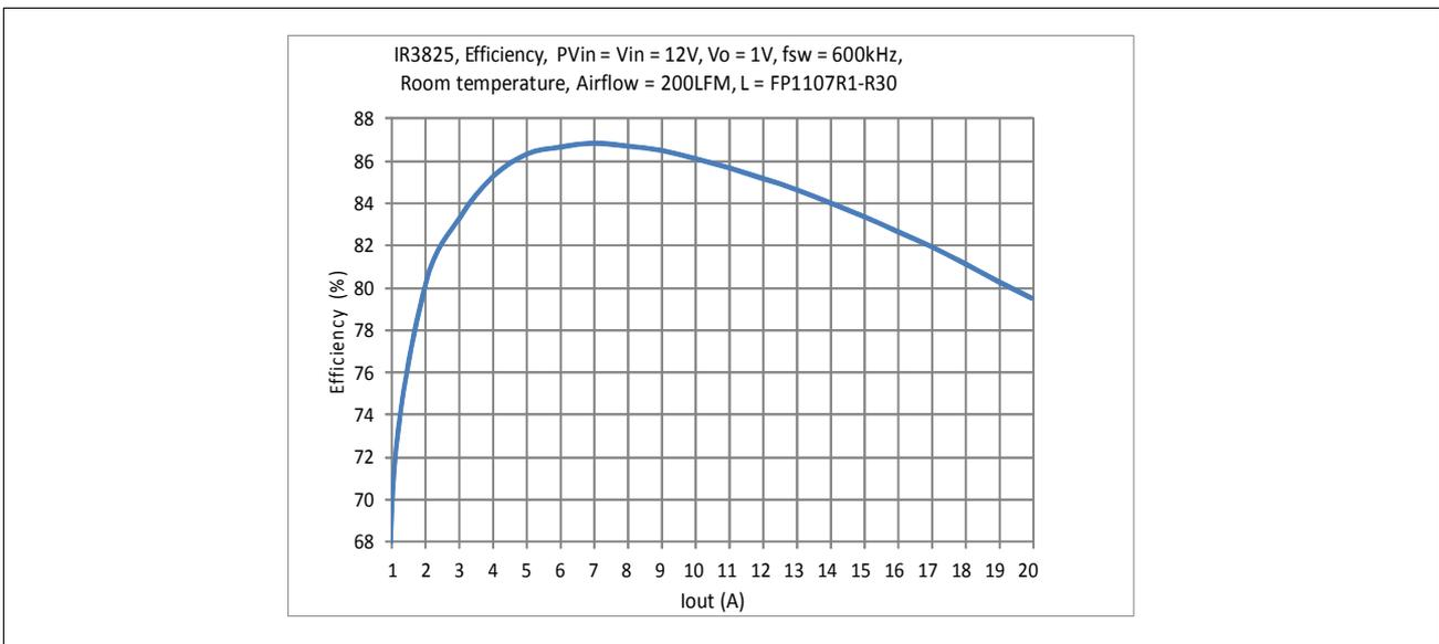
Figure 2-2 IR3825 Efficiency
