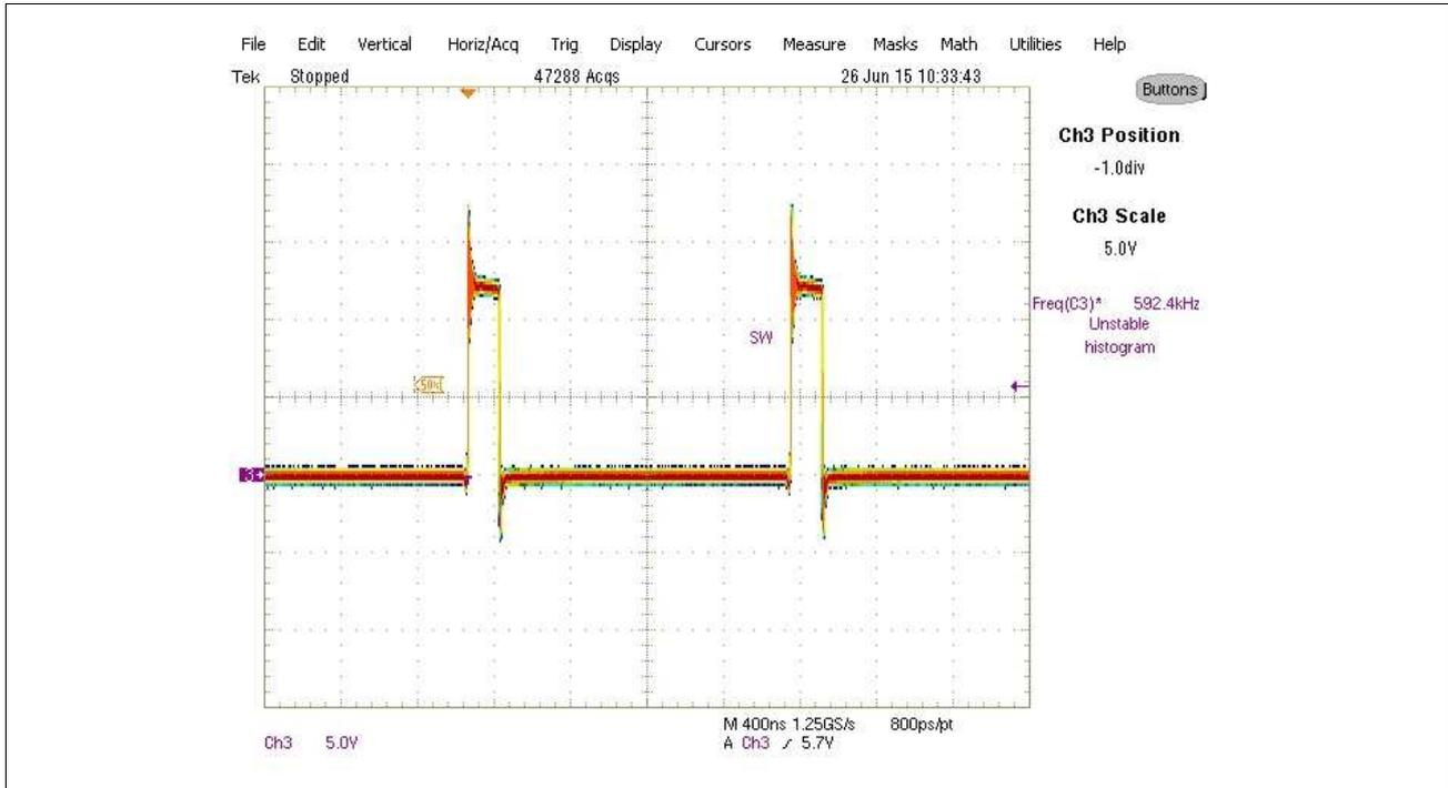
Figure 7-10 Inductor node at 20A load (Ch<sub>3</sub>: Switch Node)
