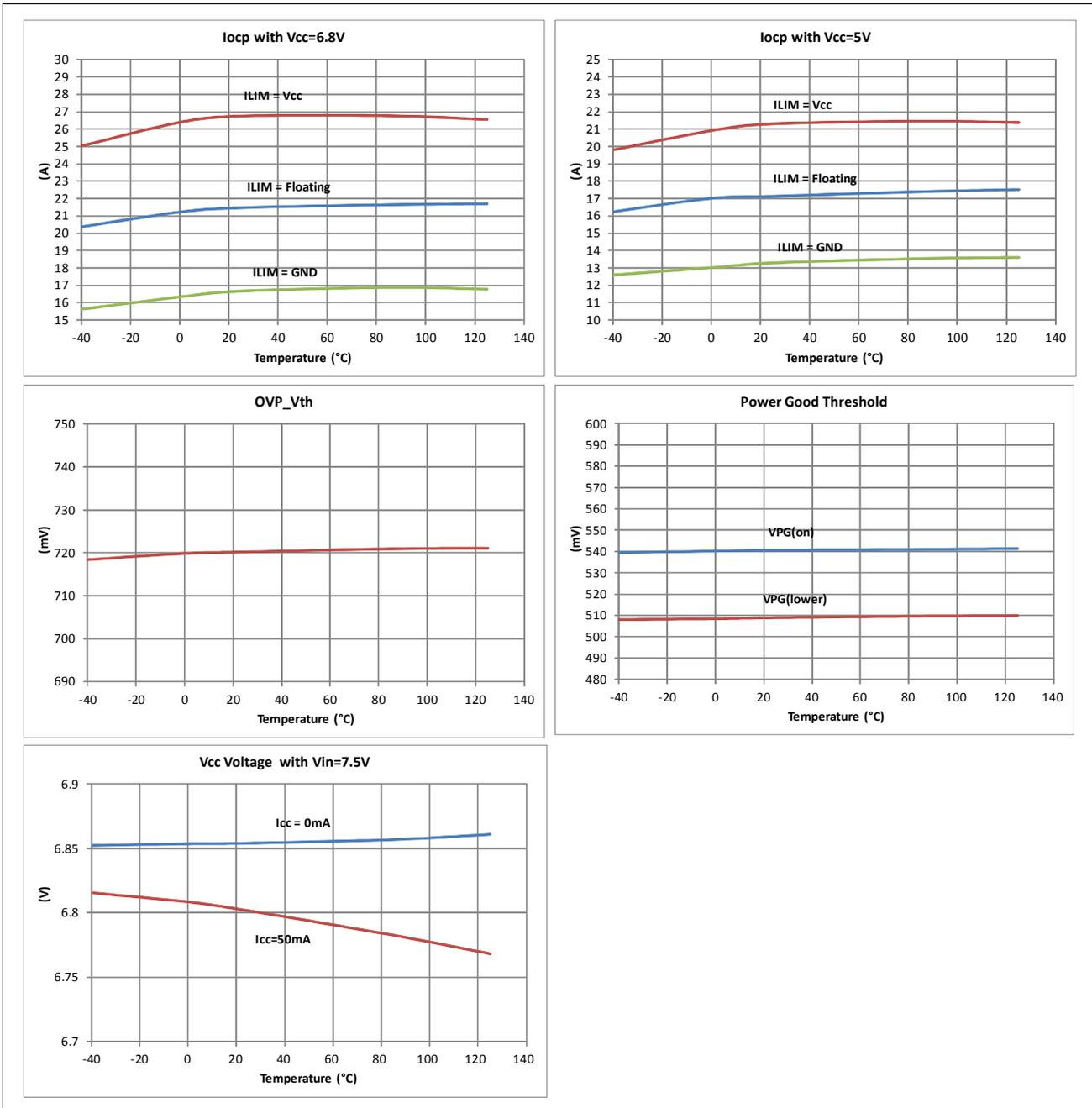
Figure 5-8 Typical Operation Characteristics (Set 2 of 2)
