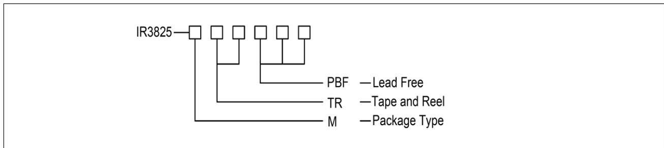
Figure 1-1 IR3825 Part Number Configuration Code
