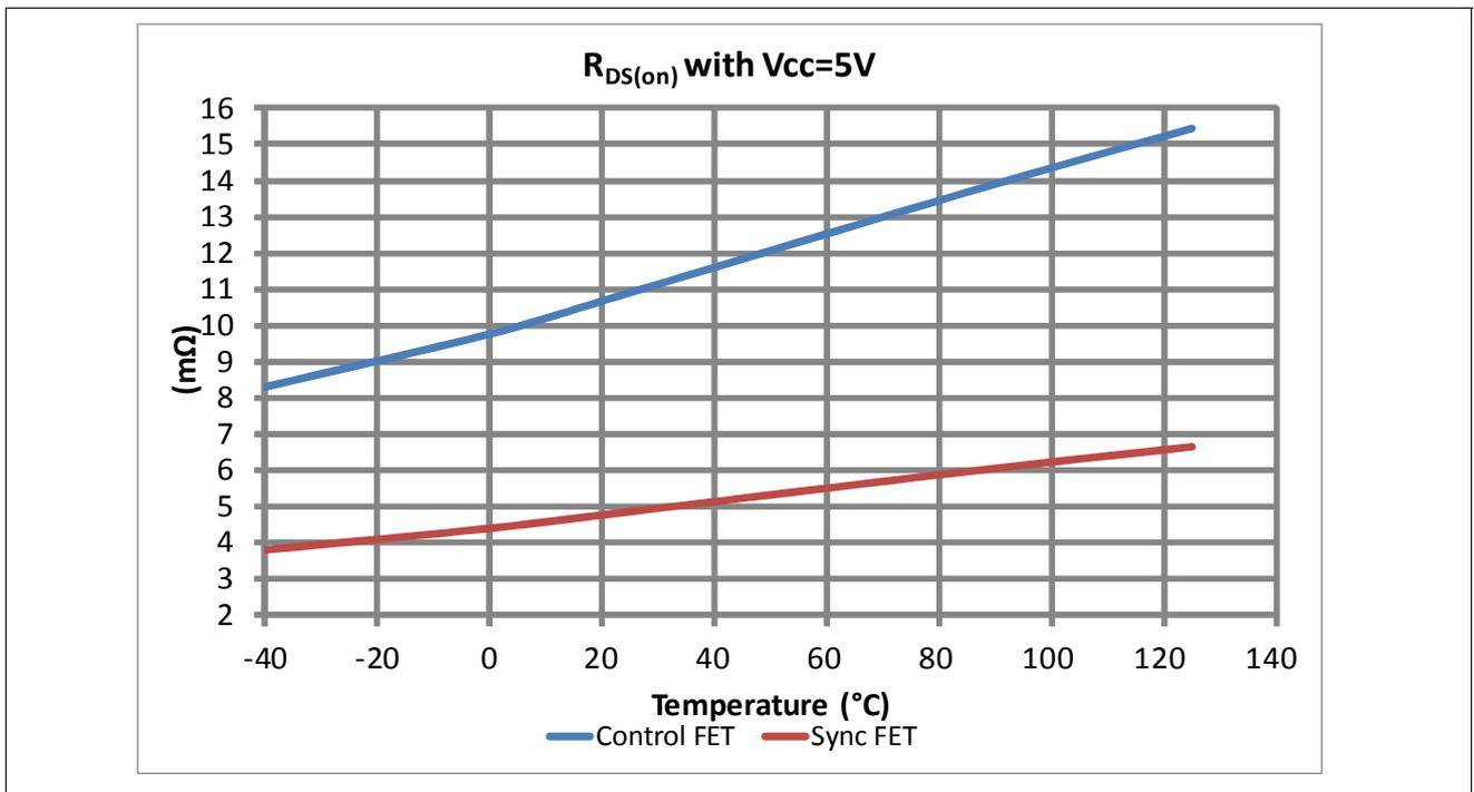
Figure 5-6  $R_{DS(on)}$  with  $V_{CC} = 5.0V$  Over Temperature
