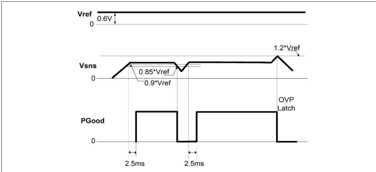
**Figure 6-11 Vsns vs. PGood Relationship Timing Diagram**
