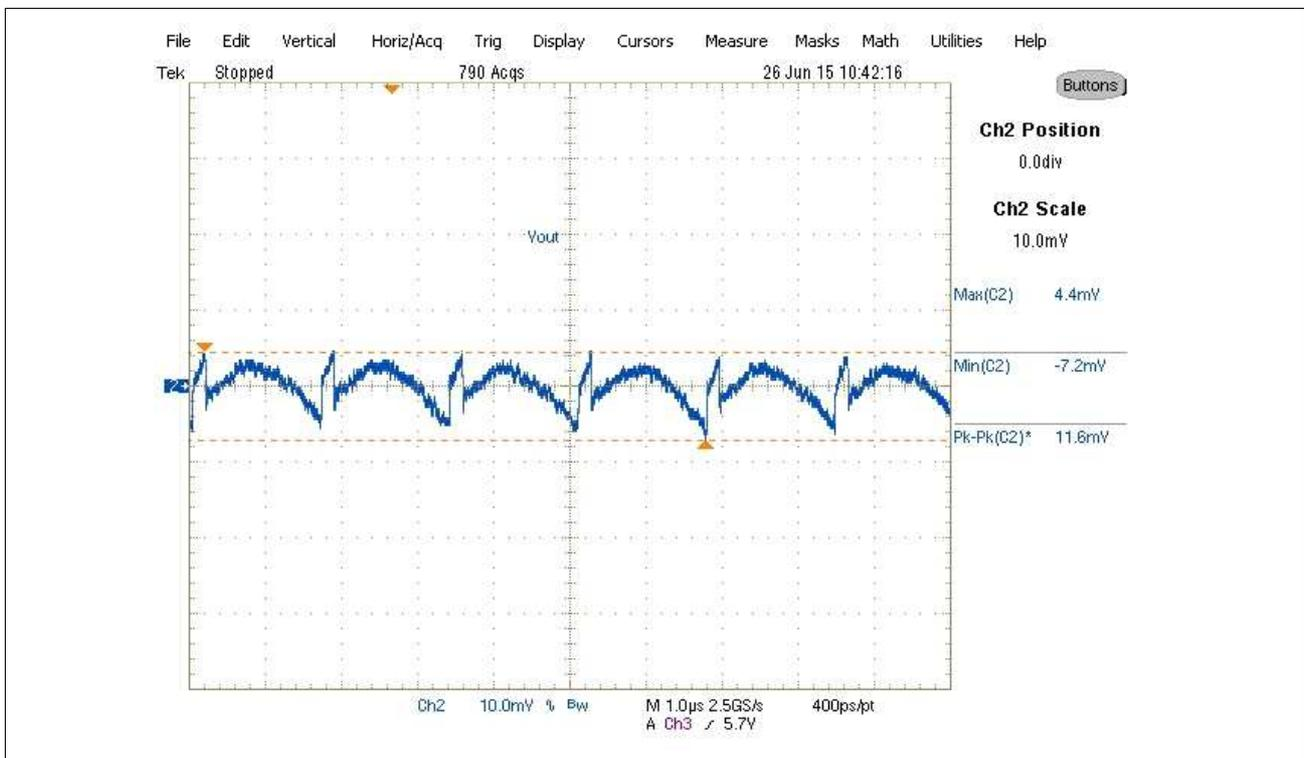
Figure 7-9 Output voltage ripple, 20A load (Ch<sub>2</sub>:Vout)
