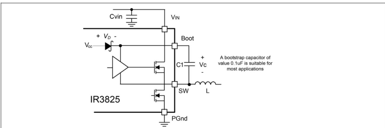
Figure 7-3 Bootstrap Circuit to Generate  $V_c$  Voltage.
