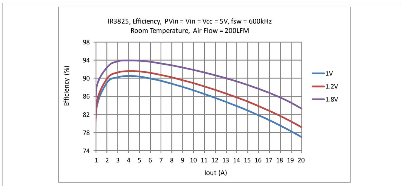
**Figure 5-3 IR3825: Efficiency Curves -  $P_{V_{in}} = V_{in} = V_{CC} = 5V$**
