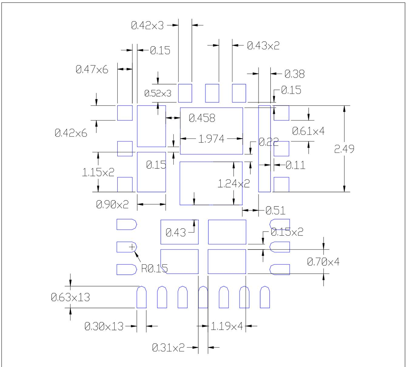
Figure 8-7 Stencil pad spacing (all dimensions in mm)
