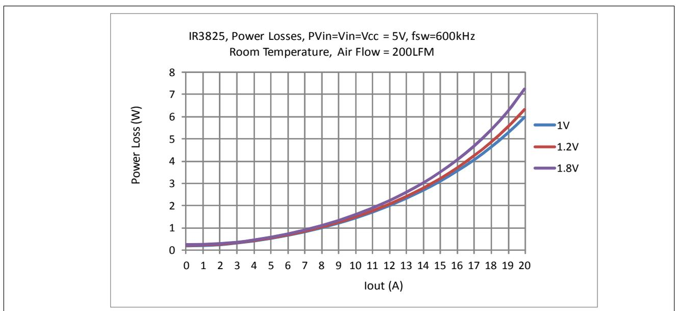
**Figure 5-4 IR3825: Power Loss Curves-  $P_{V_{in}} = V_{in} = V_{CC} = 5V$**
