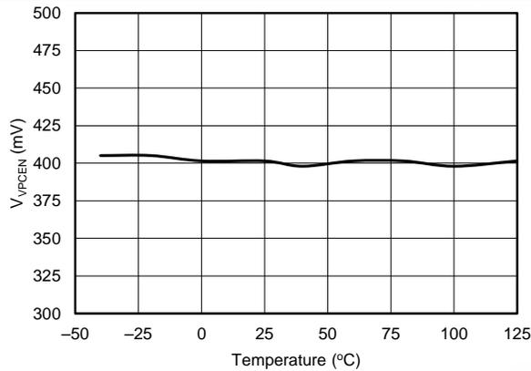
Figure 3. VPC Enable Threshold vs Temperature
