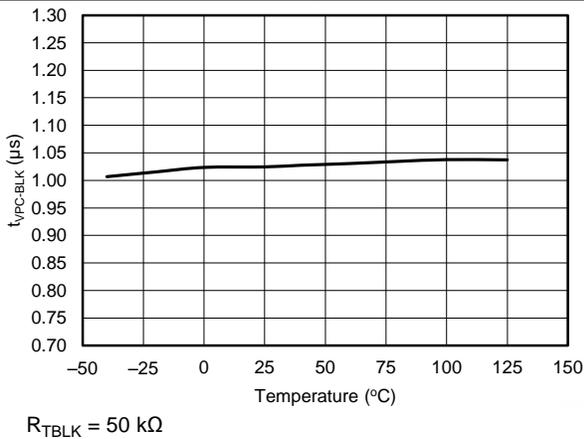
**Figure 9. VPC Blanking Time vs Temperature (maximum setting)**
