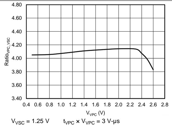
Figure 6. VPC-to-VSC Ramp Gain Ratio vs VPC Voltage
