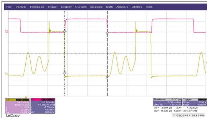
C2(RED): DRV signal to synchronous rectifier Q1
