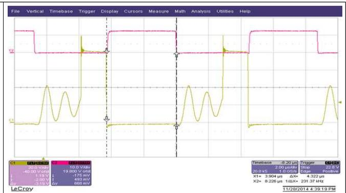
C2(RED): DRV signal to synchronous rectifier Q1
