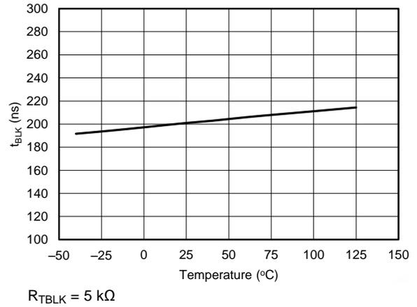
**Figure 8. VPC Blanking Time vs Temperature (minimum setting)**
