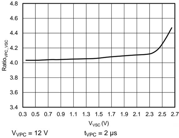
**Figure 7. VPC-to-VSC Ramp-Gain Ratio vs VSC Voltage**
