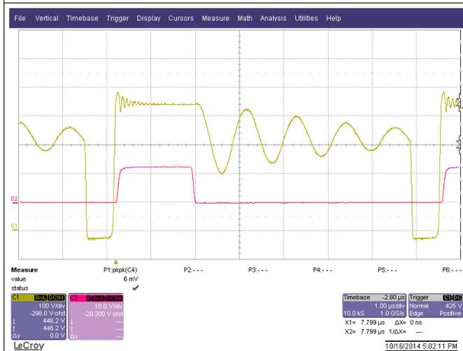
C2(RED): DRV signal to synchronous rectifier Q1
