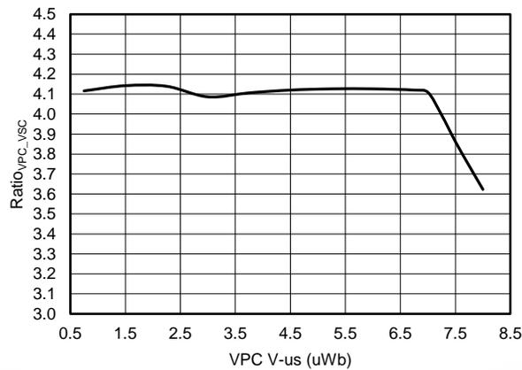
**Figure 16. Ratio<sub>VPC\_VSC</sub> vs VPC V- $\mu$ s**
