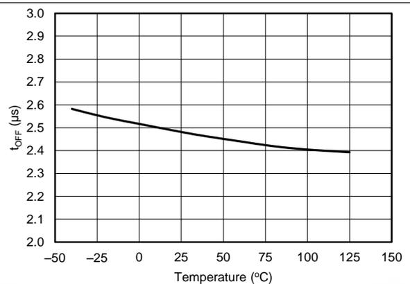
**Figure 12. DRV Minimum Off Time vs Temperature**
