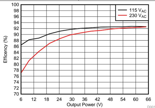
Figure 29. Efficiency vs Output Power
