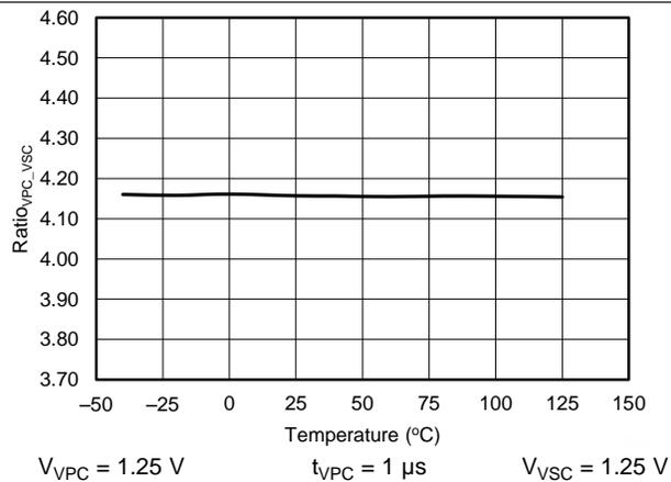
Figure 5. VPC-to-VSC Ramp Gain Ratio vs Temperature
