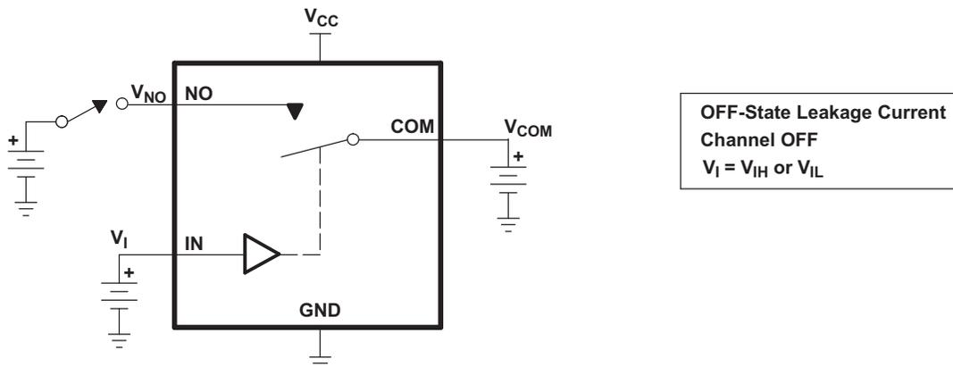
Figure 16. OFF-State Leakage Current ( $I_{COM(OFF)}$ ,  $I_{NO(OFF)}$ ,  $I_{COM(PWROFF)}$ ,  $I_{NOC(PWRFF)}$ )
