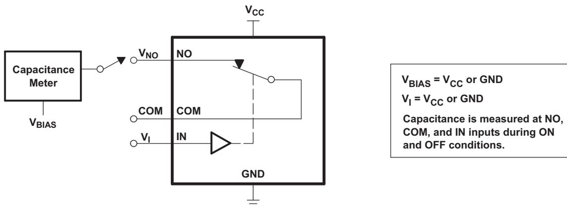
Figure 18. Capacitance ( $C_I$ ,  $C_{COM(OFF)}$ ,  $C_{COM(ON)}$ ,  $C_{NO(OFF)}$ ,  $C_{NO(ON)}$ )
