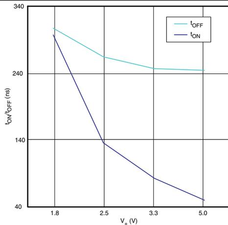
Figure 6.  $t_{ON}/t_{OFF}$  vs Supply Voltage
