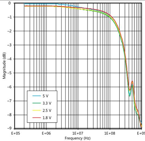
Figure 9. Insertion Loss
