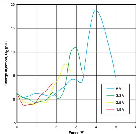
Figure 12. Charge Injection (Q<sub>C</sub>) vs Bias Voltage
