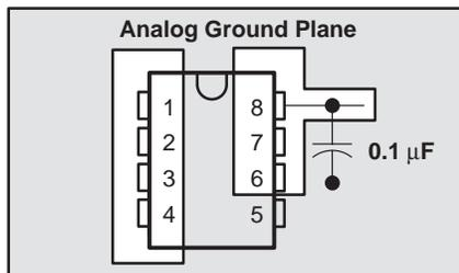
Figure 20. Power-Supply Bypassing
