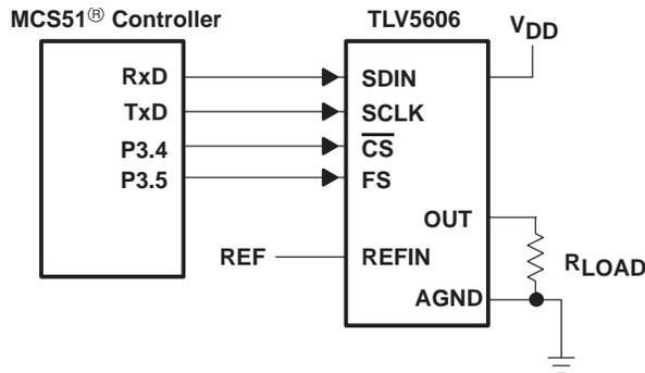
**Figure 18. TLV5606 to MCS51<sup>®</sup> Controller Interface**
