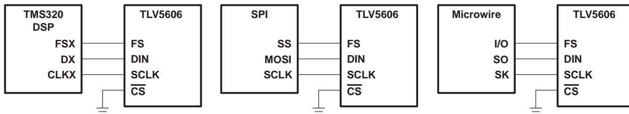
Figure 16. Three-Wire Interface
