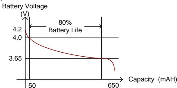
Figure 2. Li-ion Battery Energy Capacity Versus Battery Voltage.
