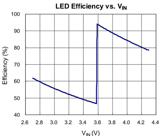
Figure 3. Efficiency of RT9363. ( $I_{LED} = 60\text{mA}$ ,  $V_F = 3.45\text{V}$ )
