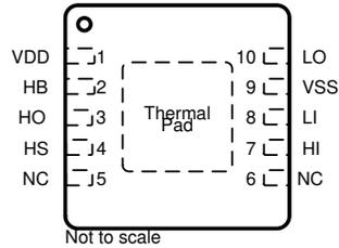
**Figure 5-3. DPR Package 10-Pin SON Top View**
