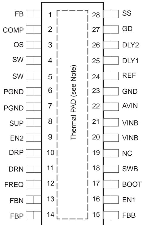
NOTE: The thermally enhanced PowerPAD™ is connected to PGND.
