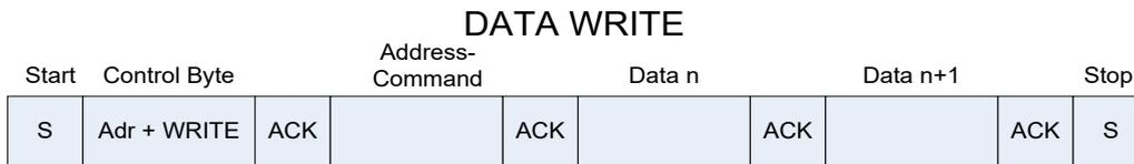
**Figure 7.4: I<sup>2</sup>C Write.**
