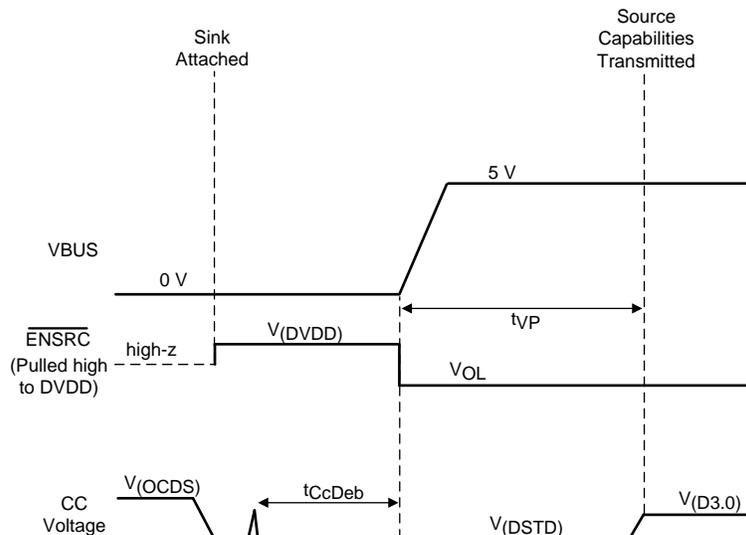
Figure 3. Timing Illustration for t<sub>CcDeb</sub> and t<sub>VP</sub>, Under Persistent Fault Condition
