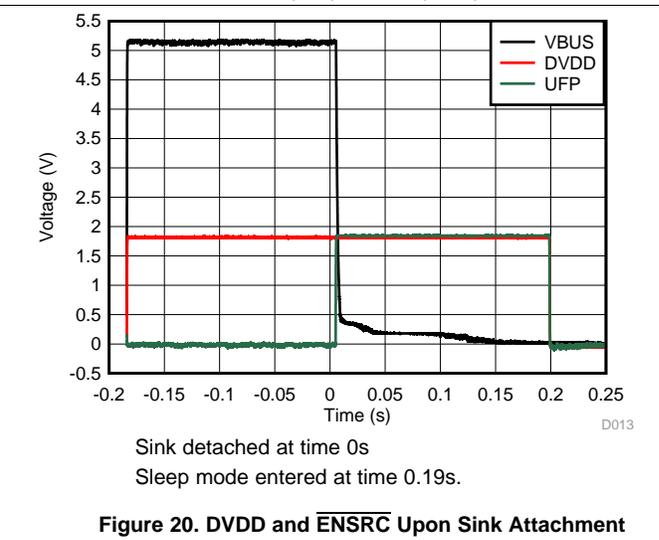
Figure 20. DVDD and  $\overline{ENSRC}$  Upon Sink Attachment
