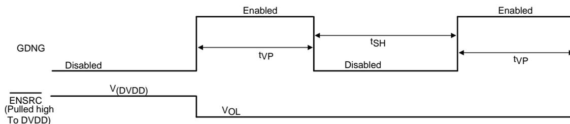
Figure 4. Timing Illustration for t<sub>SH</sub> and t<sub>VP</sub>, with VBUS Shorted to Ground
