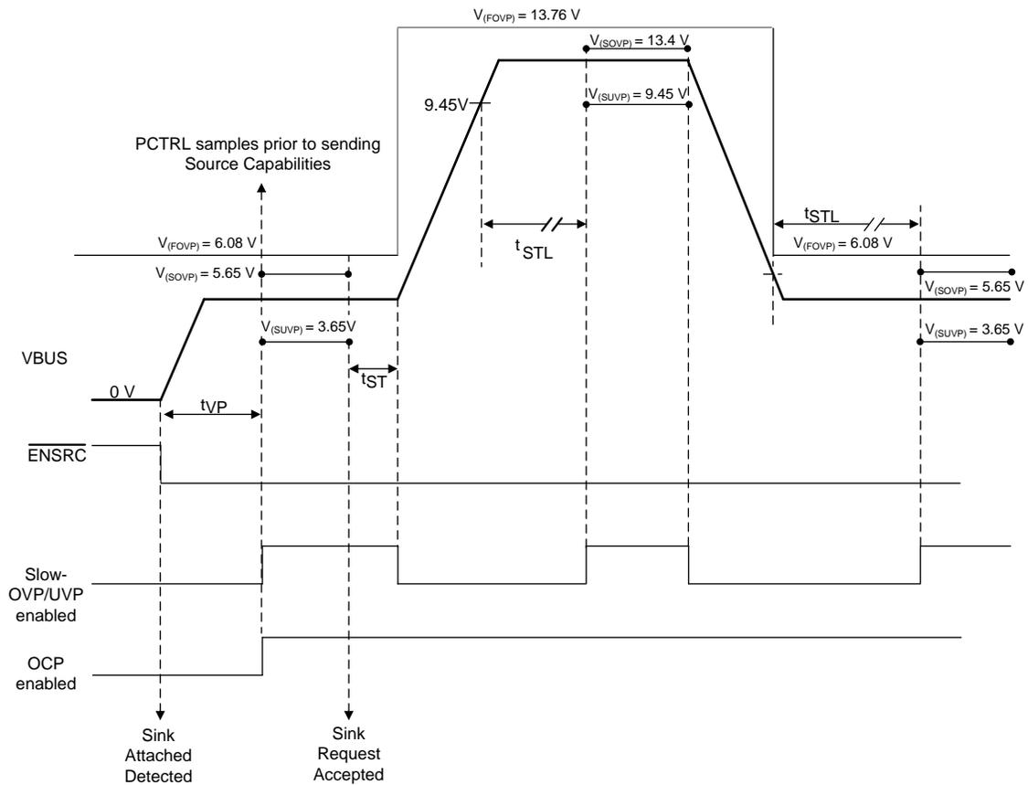
Figure 1. Timing Illustration for  $t_{VP}$ ,  $t_{ST}$  and  $t_{STL}$ , After Sink Attachment Negotiation to 12 V Then Back to 5 V.  $V_{(SOVP)}$  and  $V_{(SUVP)}$  are Disabled Around Voltage Transitions.
