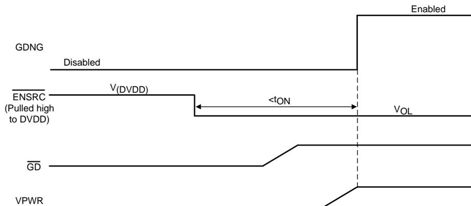
Figure 5. Timing Illustration for t<sub>ON</sub>
