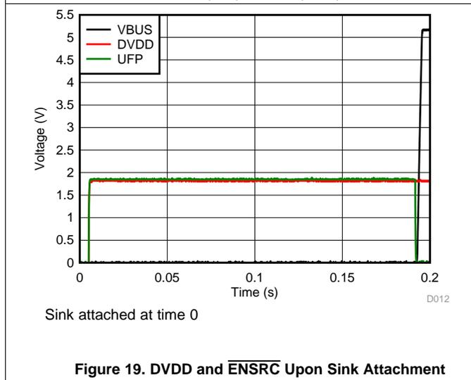
Figure 19. DVDD and  $\overline{ENSRC}$  Upon Sink Attachment
