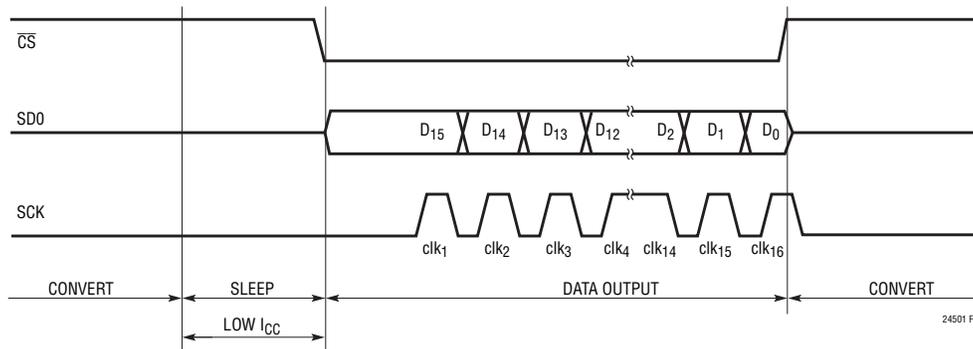
Figure 7. Idle-Low (CPOL = 0) Clock.  $\overline{CS}$  Triggers a New Conversion
