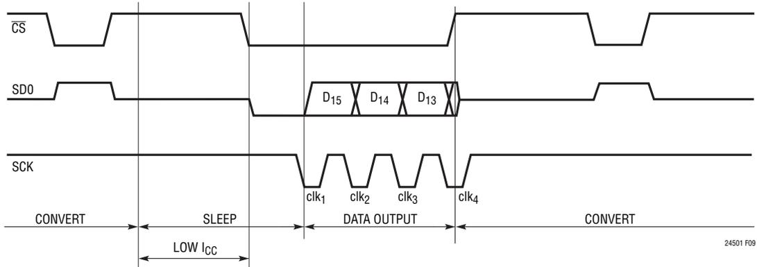
**Figure 9. Idle-High (CPOL = 1) Clock and Aborted I/O Example**
