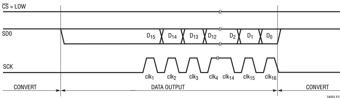
Figure 13. 2-Wire, Idle-Low ( $CPOL = 0$ ) Serial Clock Operation Example
