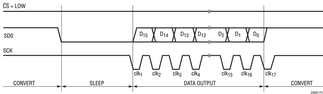
Figure 12. 2-Wire, Idle-High ( $CPOL = 1$ ) Serial Clock, Operation Example
