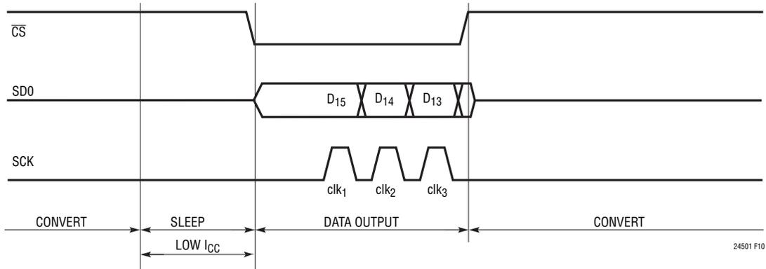
**Figure 10. Idle-Low (CPOL = 0) Clock and Aborted I/O Example**
