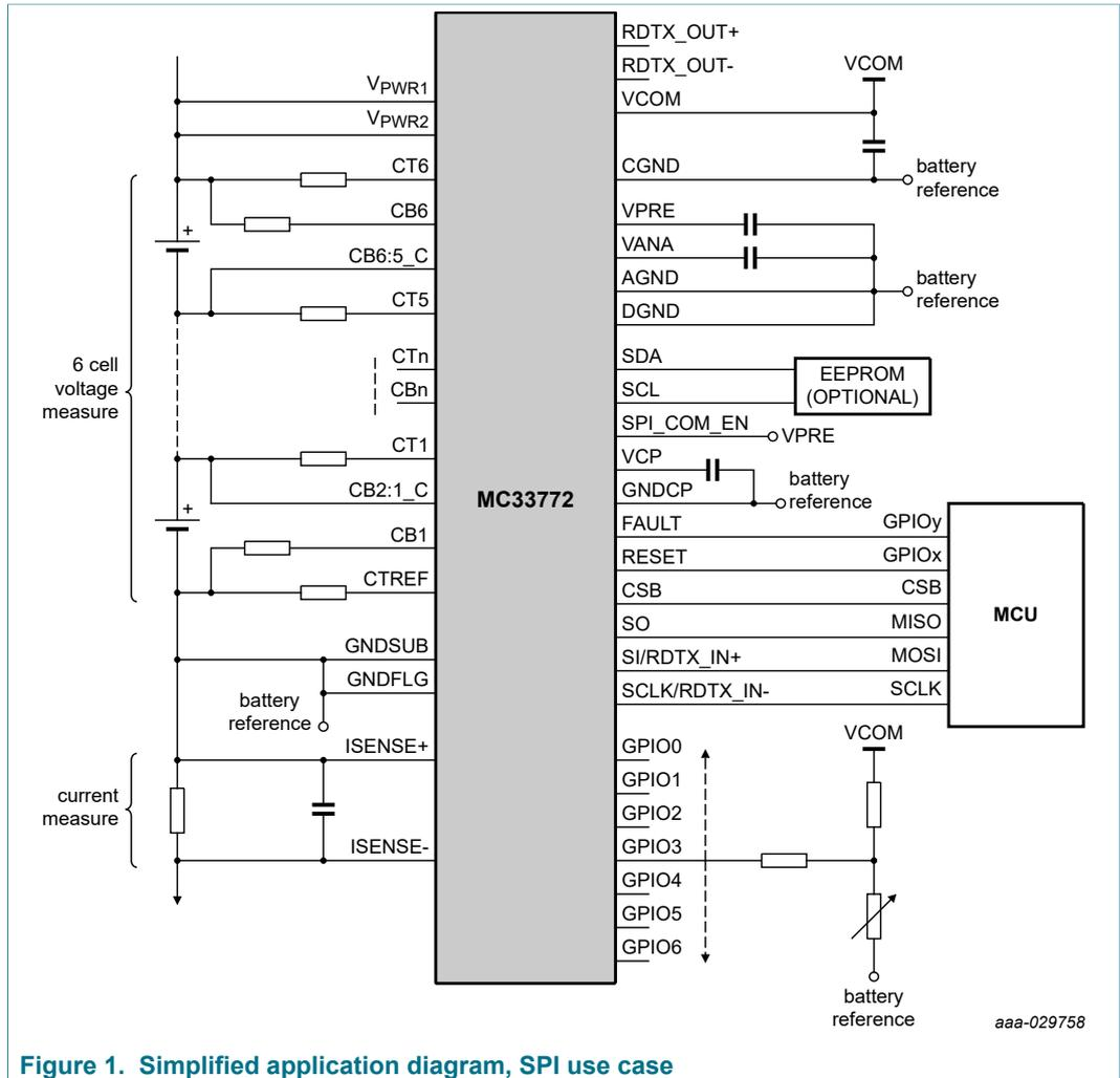
**Figure 1. Simplified application diagram, SPI use case**
