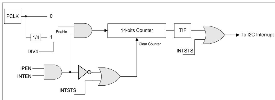
Figure 6-79 I<sup>2</sup>C Time-out Block Diagram
