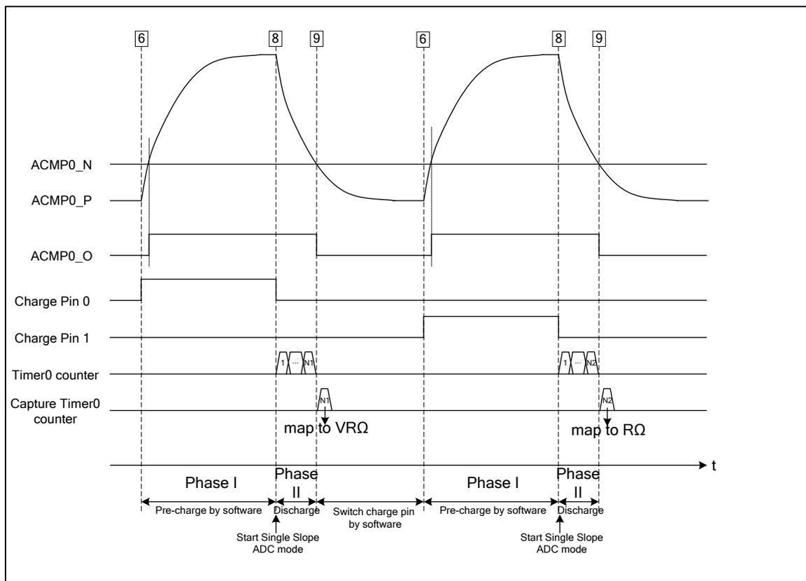
Figure 6-135 ACMP0 Single Slope ADC Mode Timing
