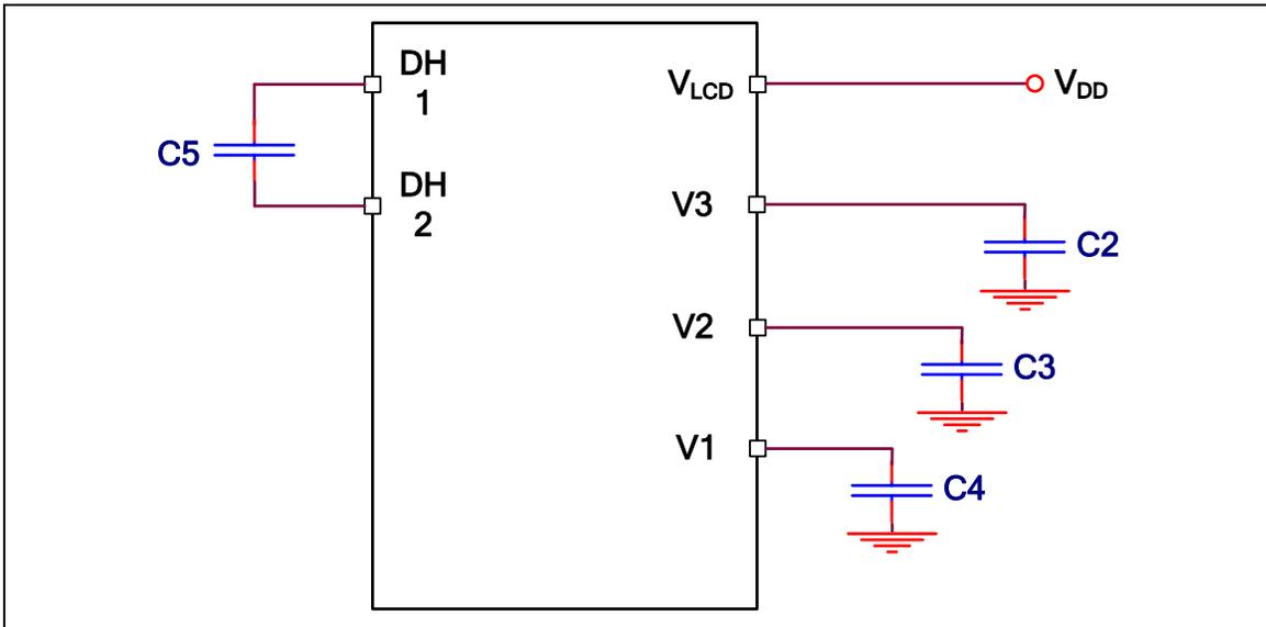
Figure 6-65 1/2 Bias (External Capacitor Ladder)
