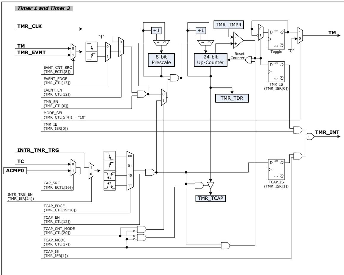
Figure 6-29 Timer 1 and Timer 3 Controller Block Diagram
