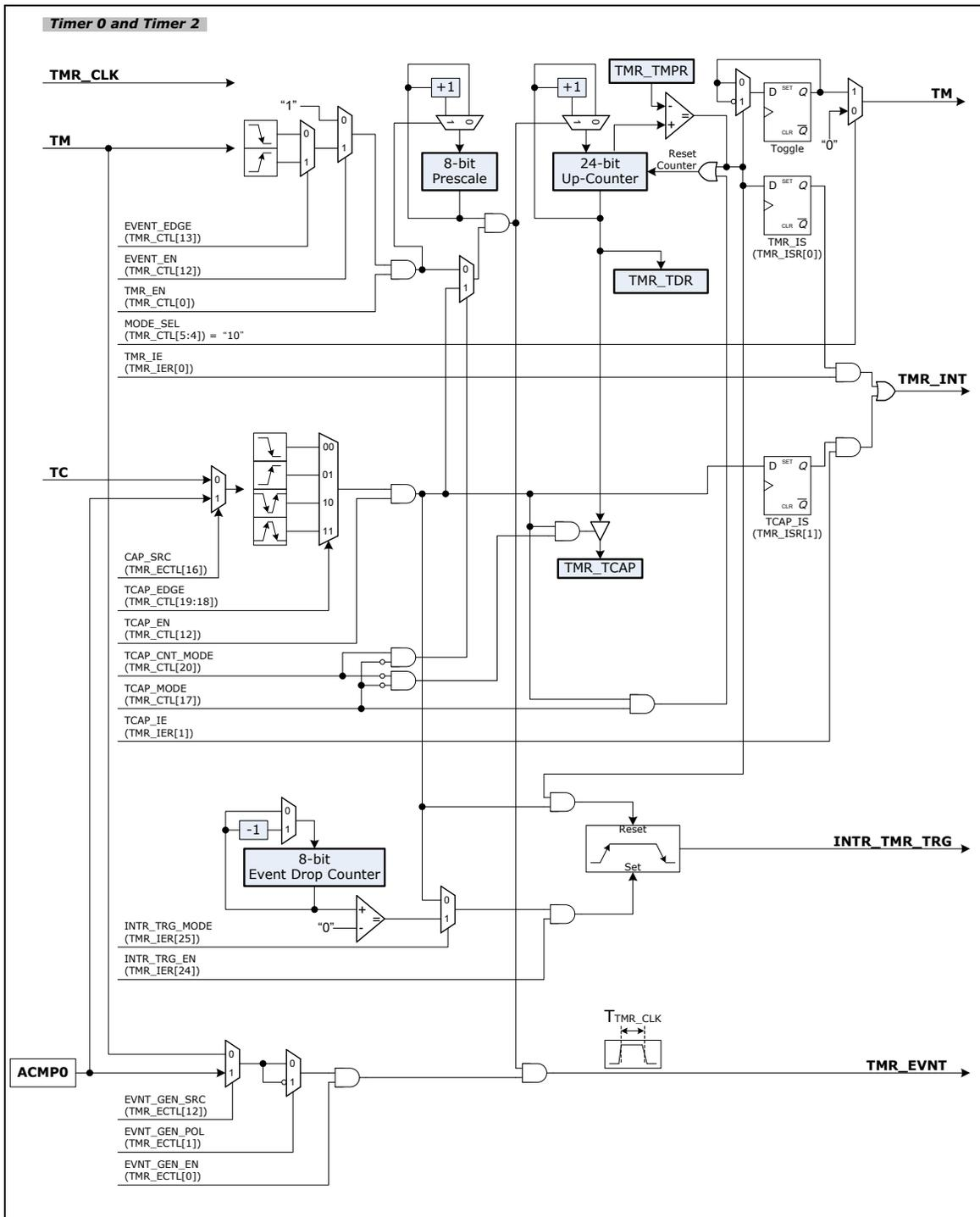
Figure 6-28 Timer 0 and Timer 2 Controller Block Diagram
