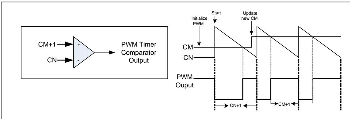
Figure 6-37 Legend of Internal Comparator Output of PWM-Timer
