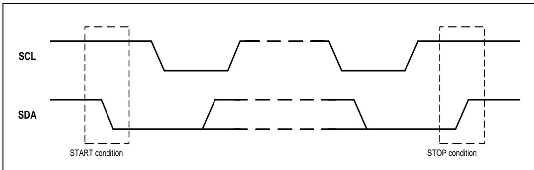
Figure 6-76 I<sup>2</sup>C START and STOP Conditions
