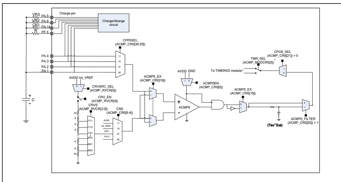
Figure 6-134 ACMP Single Slope ADC Mode Reference Circuit
