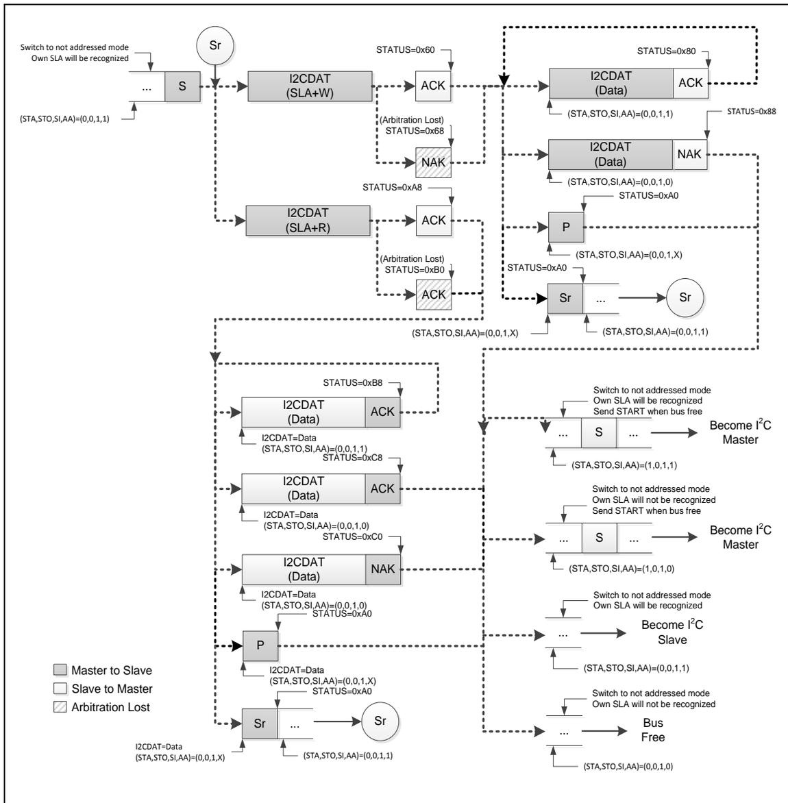
Figure 6-84 Slave Mode Control Flow
