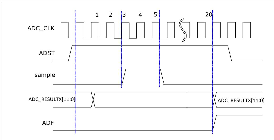
Figure 6-119 ADC Single Mode Conversion Timing Diagram
