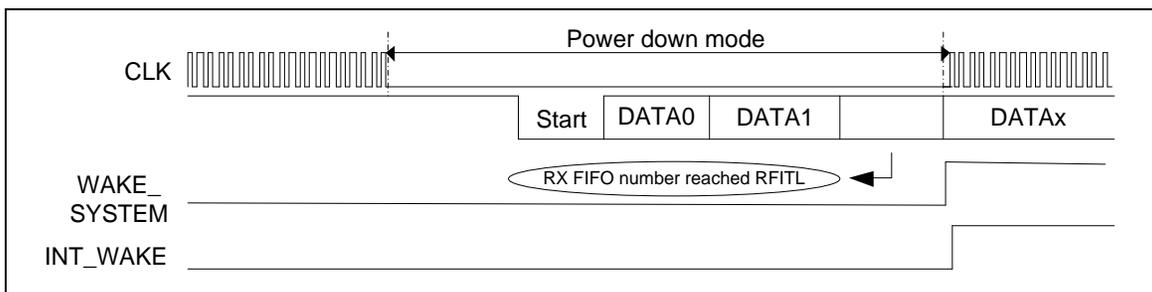
Figure 6-59 UART Receive DATA FIFO Reach RFITL Wake-Up
