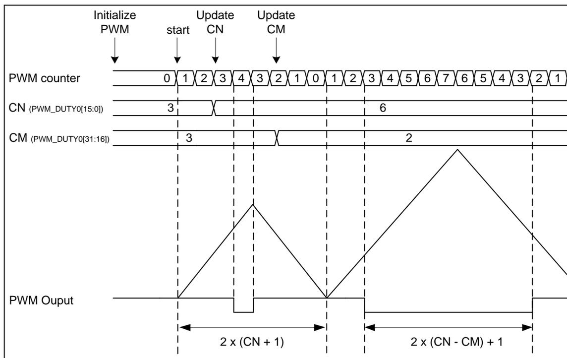
Figure 6-39 PWM-Timer Operation in Center-aligned Mode
