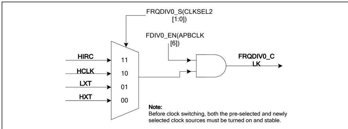
Figure 6-9 Clock Source of Frequency Divider0
