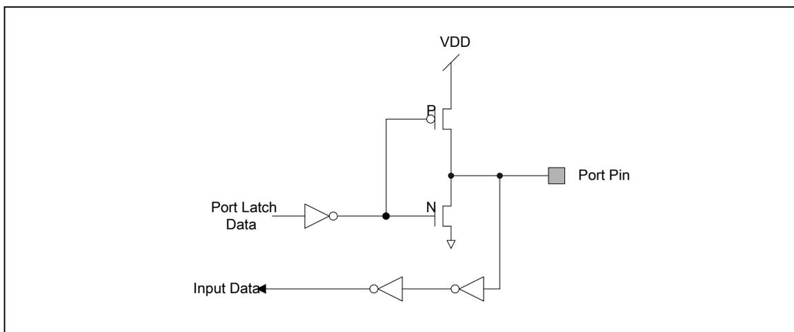
Figure 6-23 Push-Pull Output
