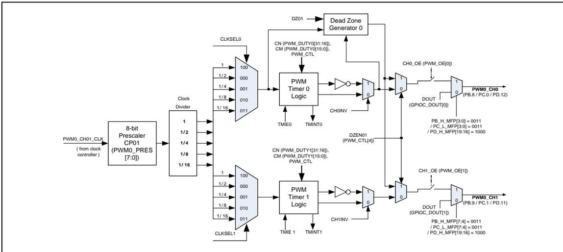
Figure 6-34 PWM Generator for Channel 0, 1
