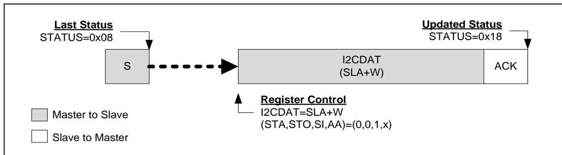
Figure 6-81 Control I2C Bus according to Current I<sup>2</sup>C Status
