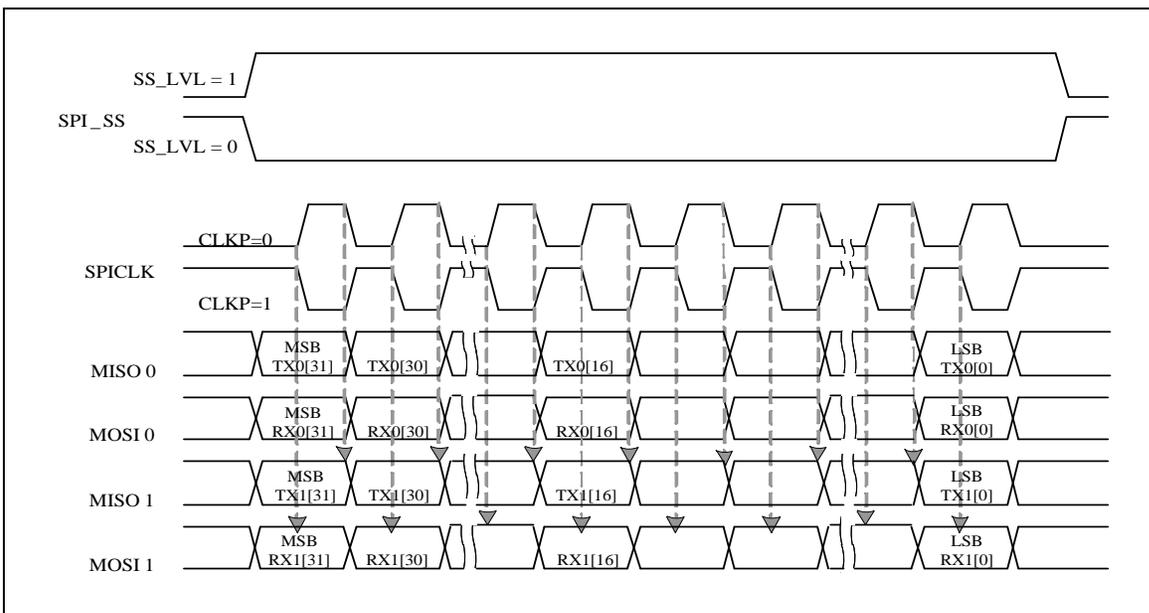
Figure 6-96 SPI 2-bit Transfer Mode Timing Diagram
