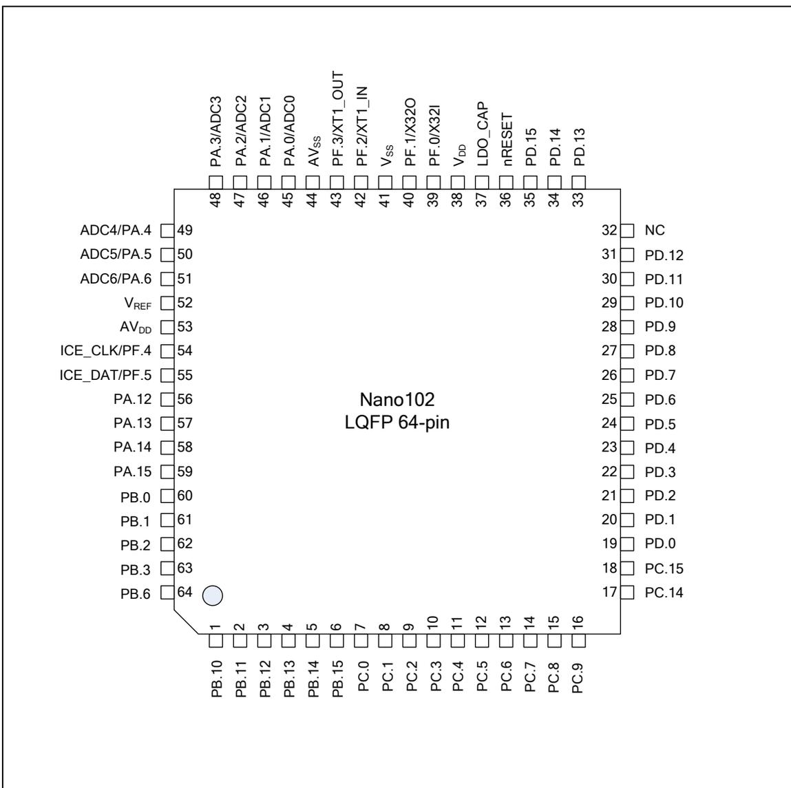
Figure 4- 2 NuMicro™ Nano102 LQFP 64-pin Diagram
