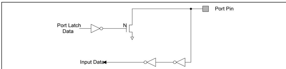
Figure 6-24 Open-Drain Output
