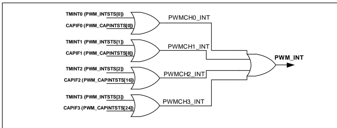
Figure 6-44 PWM-Timer Interrupt
