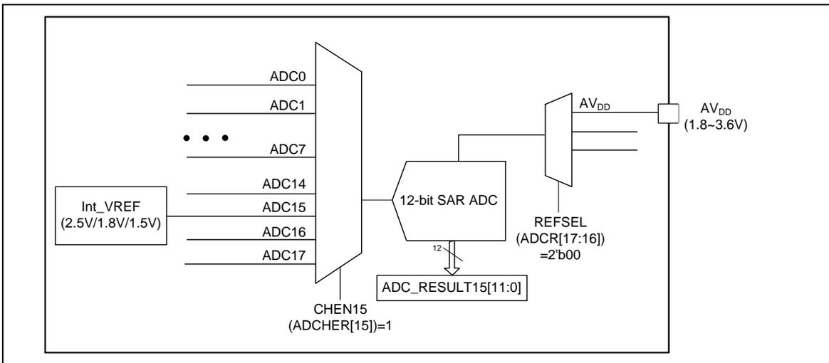
Figure 6-130 Int\_VREF for Measuring AVDD Application Block Diagram
