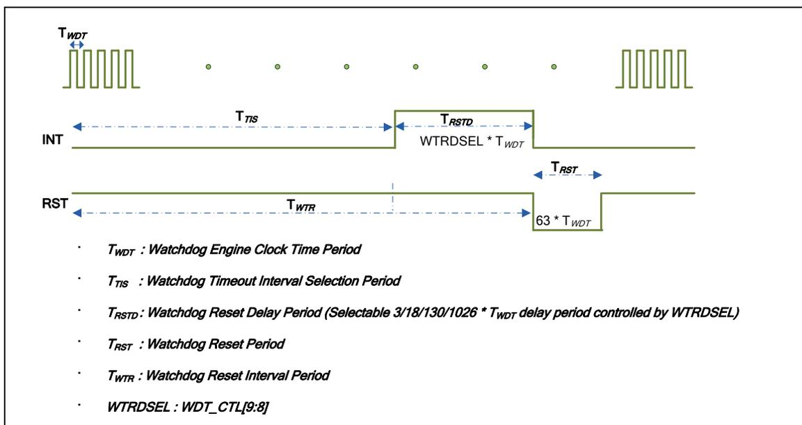
Figure 6-48 Watchdog Timing of Interrupt and Reset Signal
