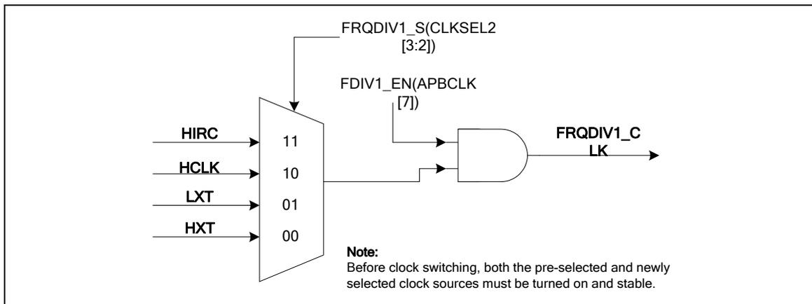
Figure 6-10 Clock Source of Frequency Divider1
