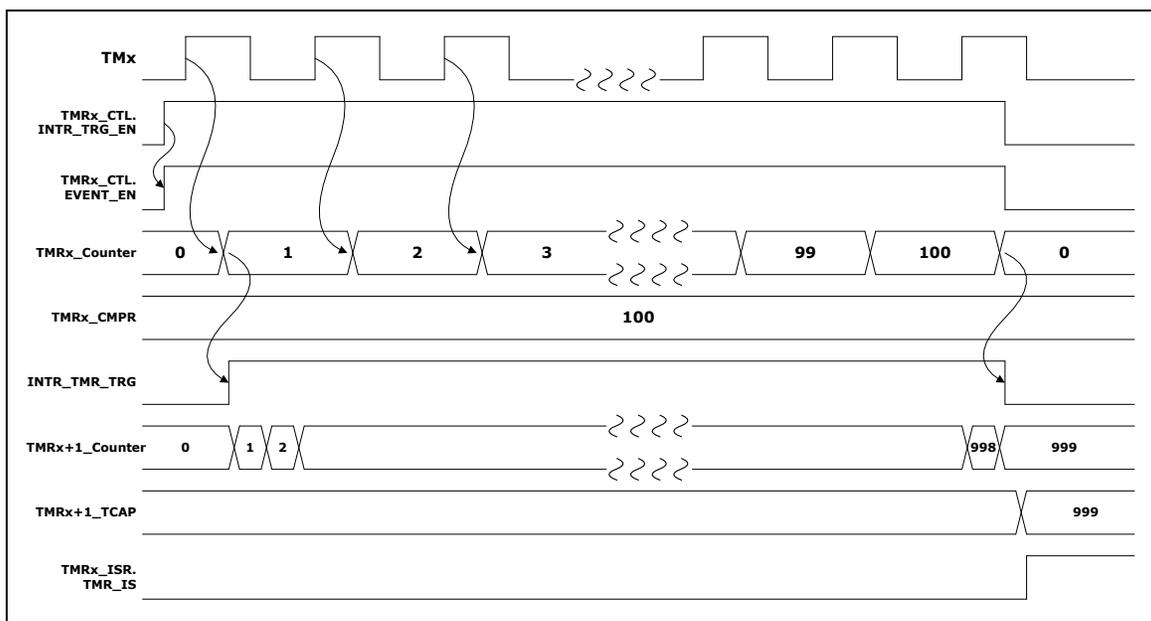
Figure 6-32 Inter-Timer Trigger Mode
