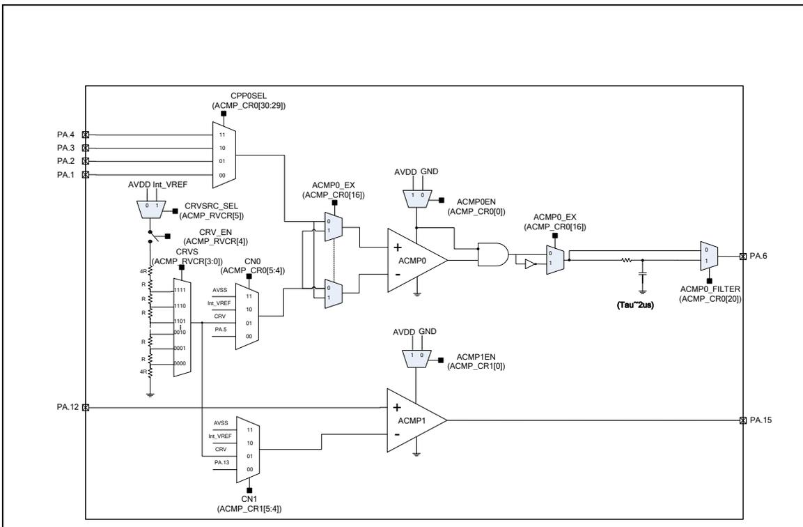
Figure 6-133 Normal Comparator Mode Block Diagram
