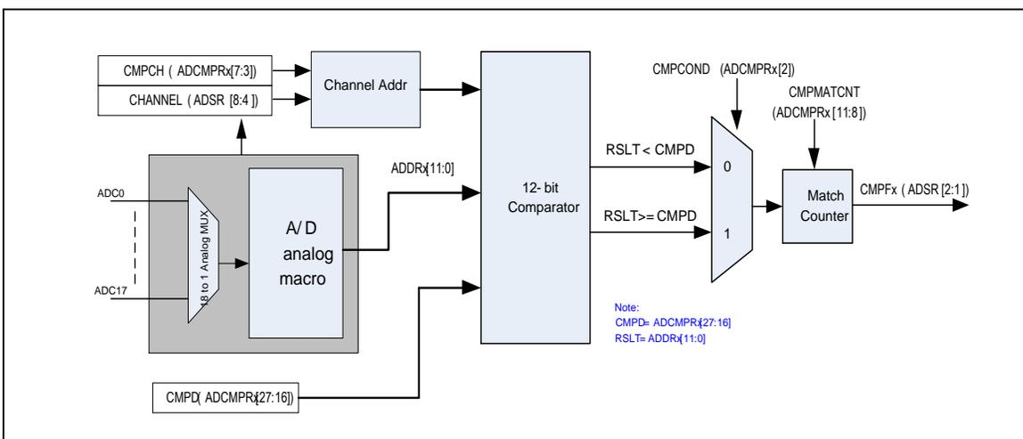
Figure 6-122 ADC Conversion Result Monitor Logic Diagram
