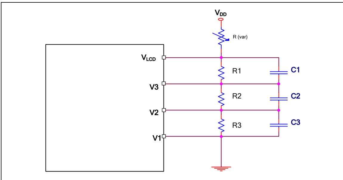
Figure 6-111 1/3 Bias (Resistor Ladder with Capacitor)
