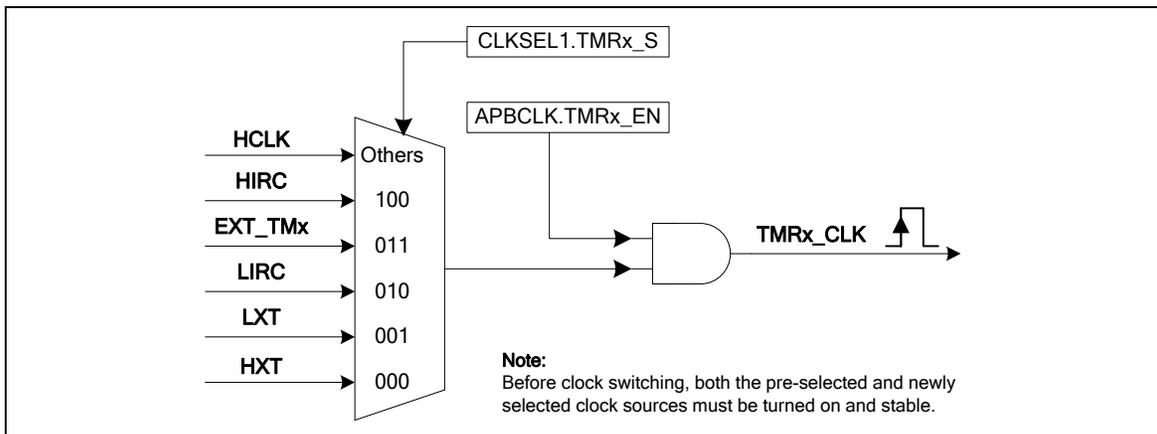
Figure 6-30 Timer Clock Controller Diagram
