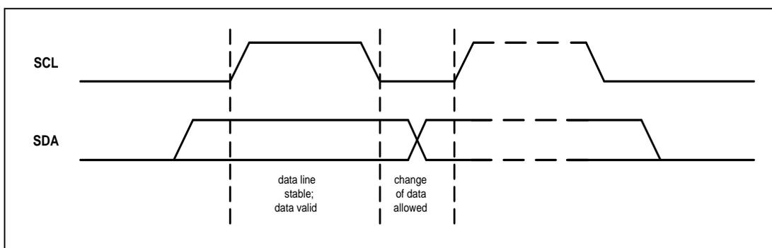
Figure 6-77 Bit Transfer on I<sup>2</sup>C Bus
