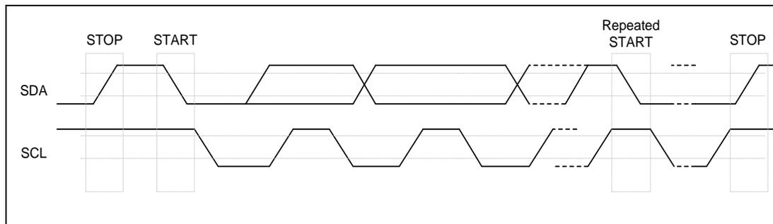
Figure 6-74 I<sup>2</sup>C Bus Timing
