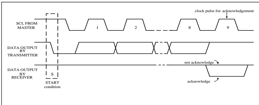
Figure 6-78 Acknowledge on I<sup>2</sup>C Bus
