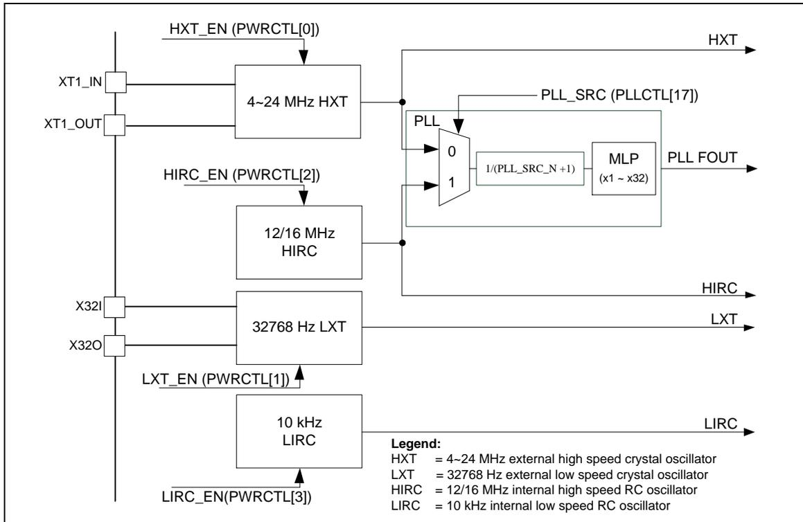
Figure 6-6 Clock Controller Block Diagram (1/3)
