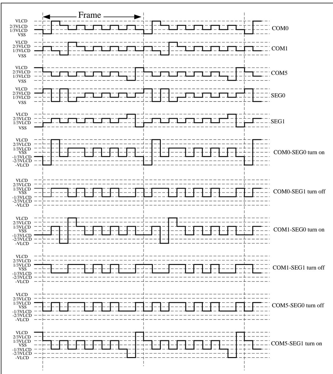
Figure 6-108 COM-SEG Signal Waveform by 1/6 Duty with 1/3 Bias
