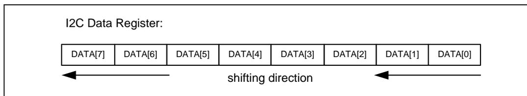
Figure 6-80 I<sup>2</sup>C Data Shifting Direction
