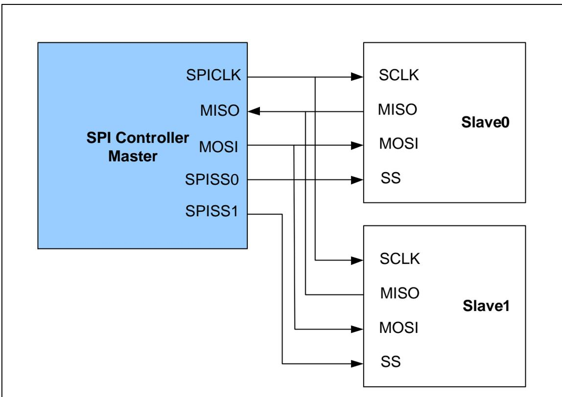
Figure 6-89 SPI Master Mode Application Block Diagram
