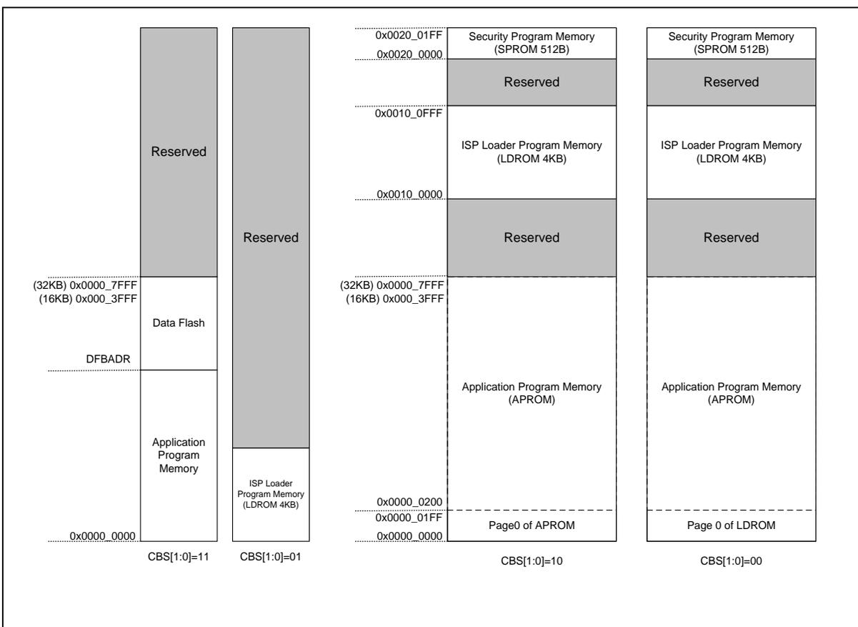
Figure 6-17 Flash Memory Mapping of CBS in CONFIG0
