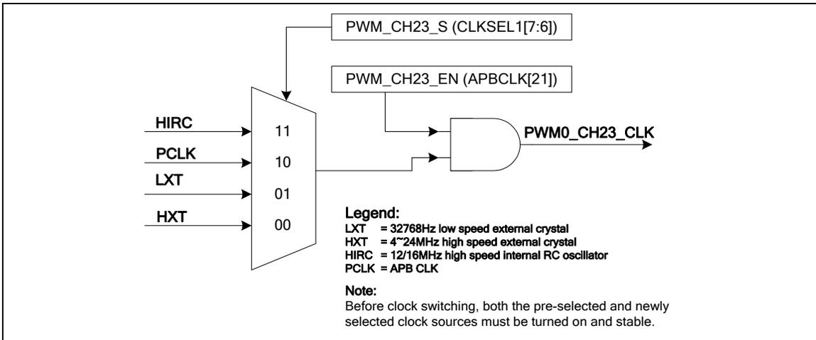
Figure 6-35 PWM Clock for Channel 2, 3
