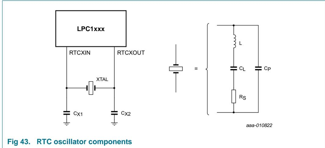
**Fig 43. RTC oscillator components**
