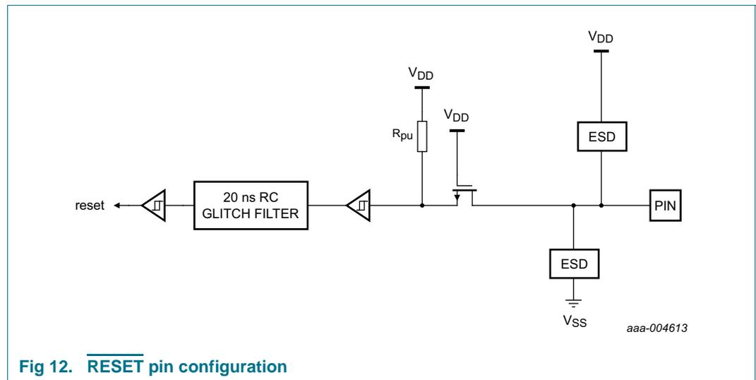
Fig 12.  $\overline{\text{RESET}}$  pin configuration
