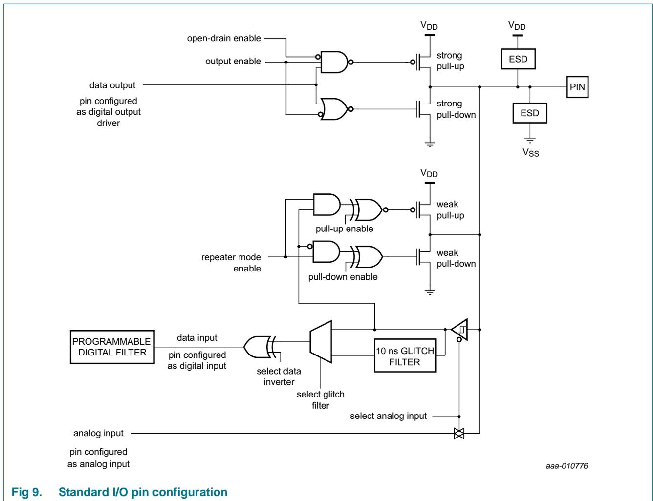
Fig 9. Standard I/O pin configuration
