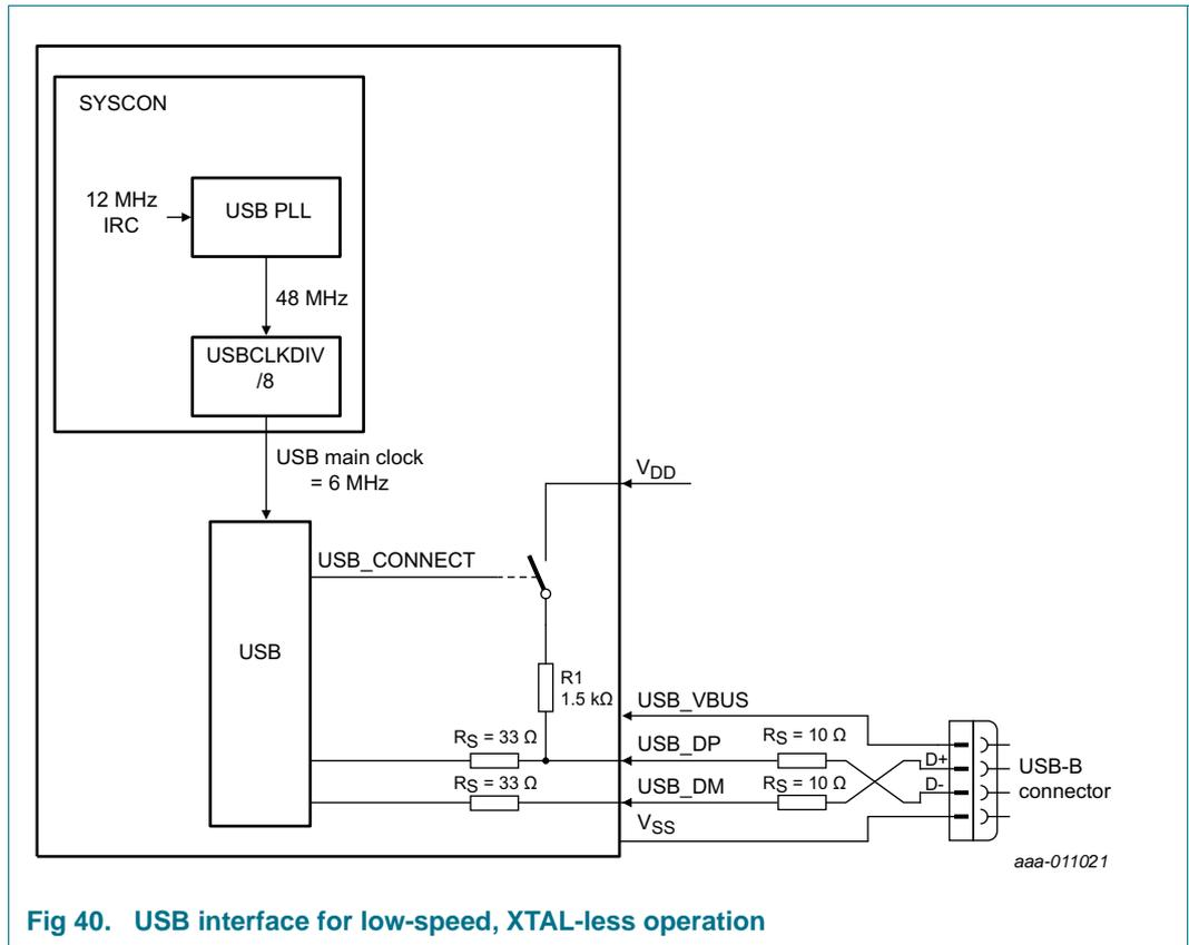
Fig 40. USB interface for low-speed, XTAL-less operation
