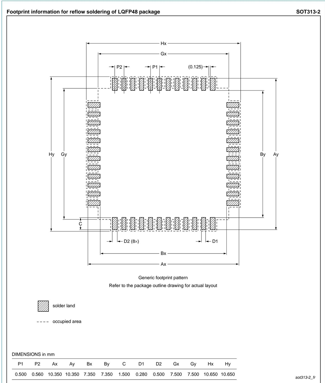
Fig 48. Reflow soldering for the LQFP48 package
