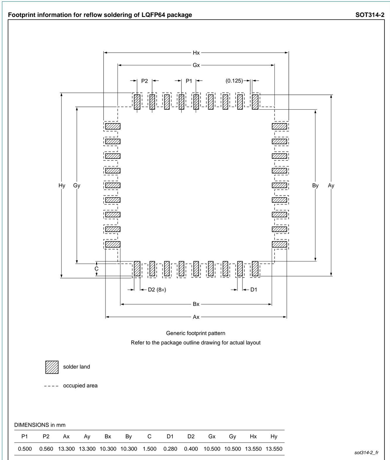
**Fig 49. Reflow soldering for the LQFP64 package**
