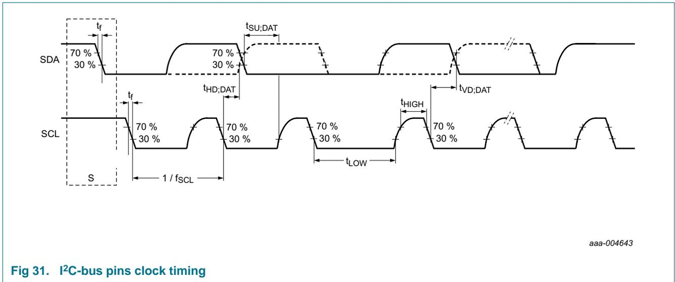
Fig 31. I<sup>2</sup>C-bus pins clock timing
