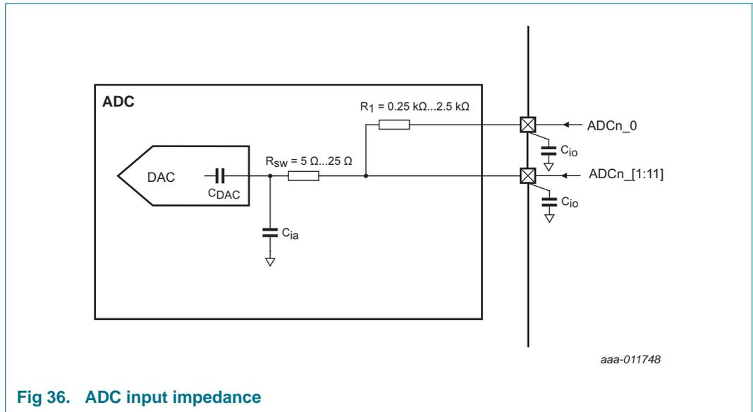
Fig 36. ADC input impedance
