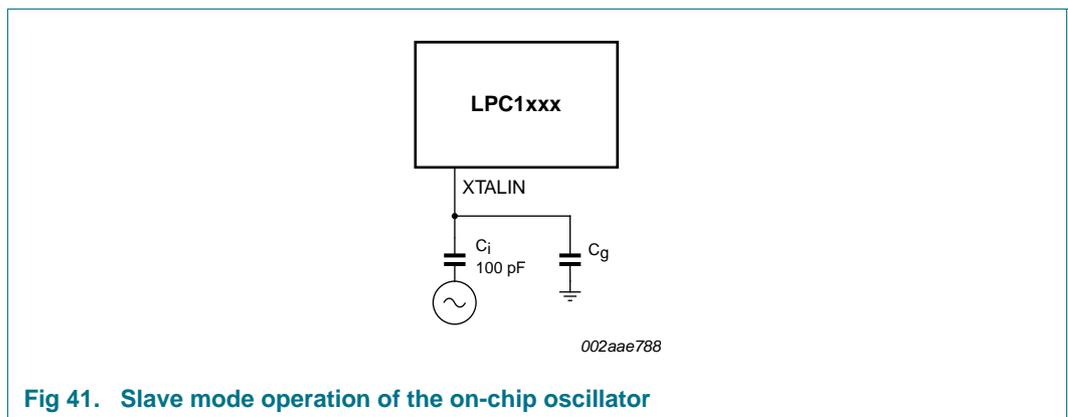
Fig 41. Slave mode operation of the on-chip oscillator
