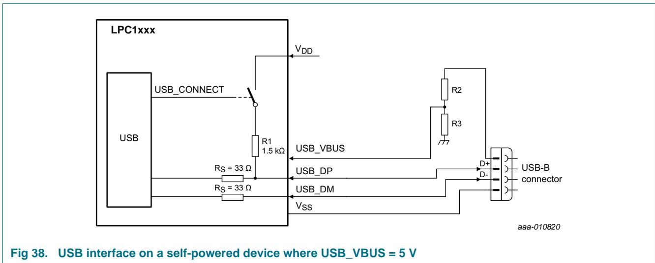
**Fig 38. USB interface on a self-powered device where USB\_VBUS = 5 V**
