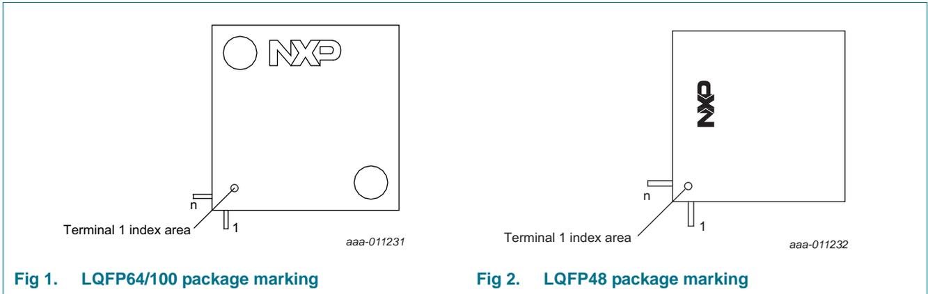
Fig 1. LQFP64/100 package marking
