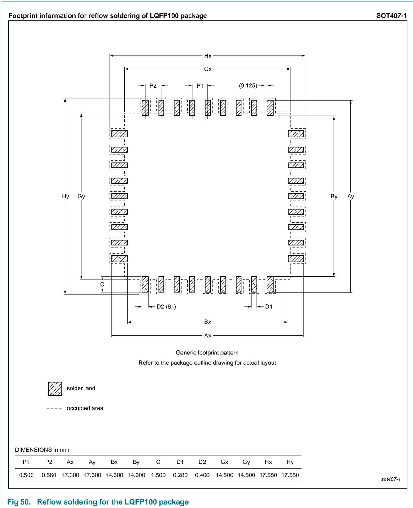
**Fig 50. Reflow soldering for the LQFP100 package**
