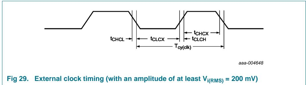
Fig 29. External clock timing (with an amplitude of at least  $V_{i(RMS)} = 200\text{ mV}$ )
