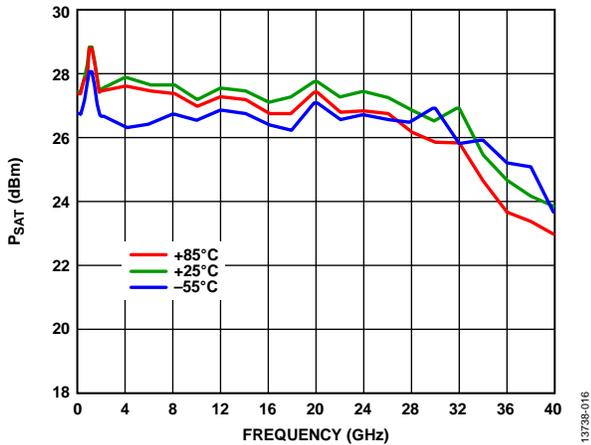
Figure 16. PSAT vs. Frequency for Various Temperatures
