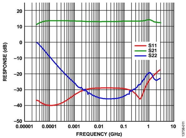
Figure 11. Low Frequency Gain and Return Loss
