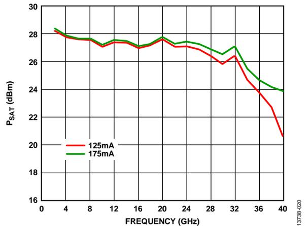
Figure 20. PSAT vs. Frequency and Supply Current
