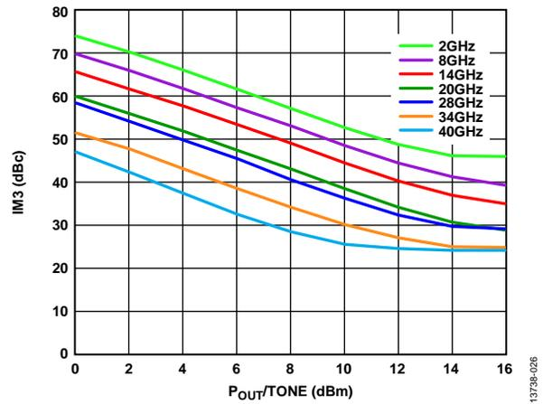
Figure 26. Output IM3 at  $V_{DD} = 11$  V
