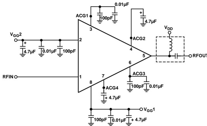
Figure 37. Application Circuit
