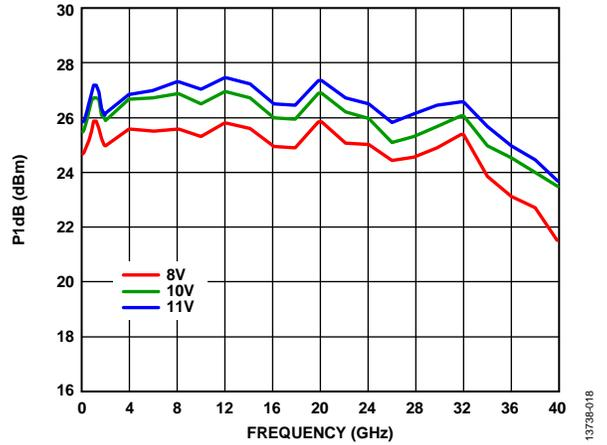
Figure 18. P1dB vs. Frequency for Various Supply Voltages
