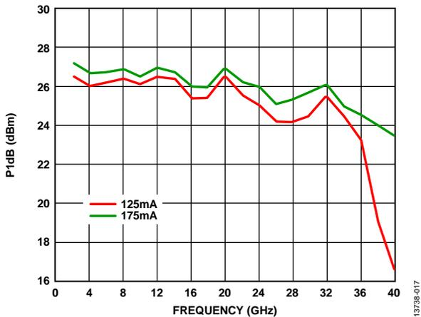
Figure 17. P1dB vs. Frequency and Supply Current
