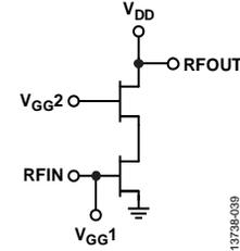
Figure 35. Fundamental Cell Schematic
