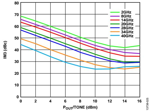
Figure 25. Output IM3 at  $V_{DD} = 8$  V
