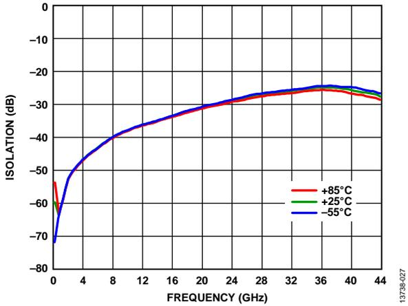
Figure 27. Reverse Isolation vs. Frequency for Various Temperatures
