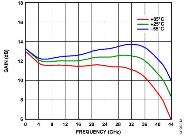
Figure 12. Gain vs. Frequency for Various Temperatures
