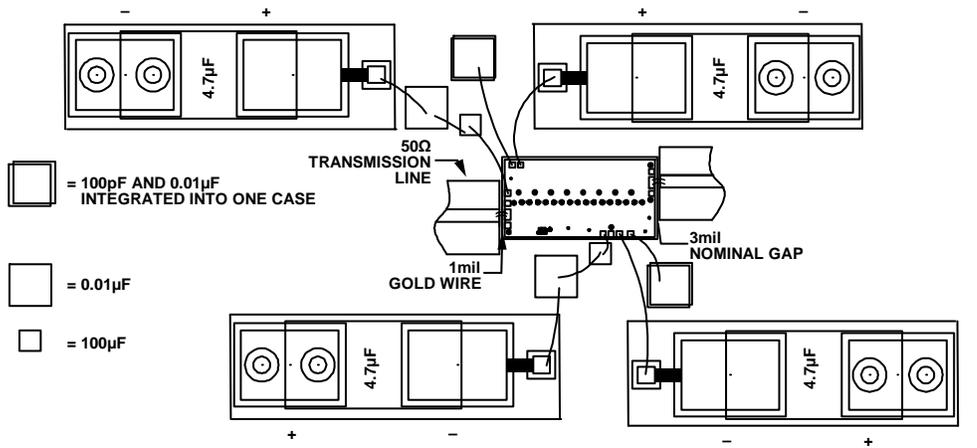
Figure 36. Assembly Diagram
