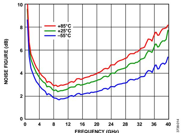
Figure 14. Noise Figure vs. Frequency for Various Temperatures
