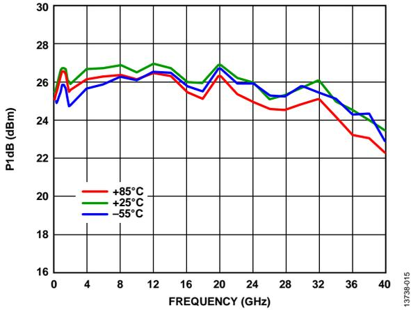
Figure 15. P1dB vs. Frequency for Various Temperatures
