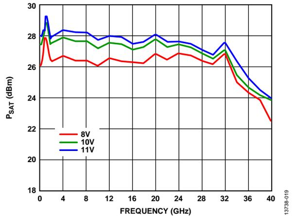
Figure 19. PSAT vs. Frequency for Various Supply Voltages
