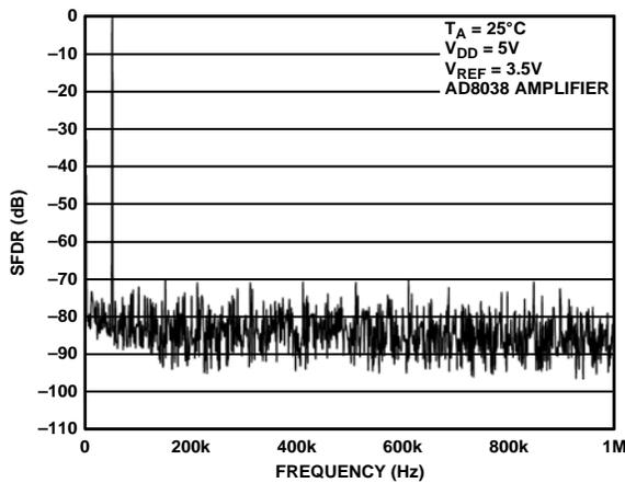
Figure 24. Wideband SFDR, Clock = 2 MHz,  $f_{OUT} = 50$  kHz
