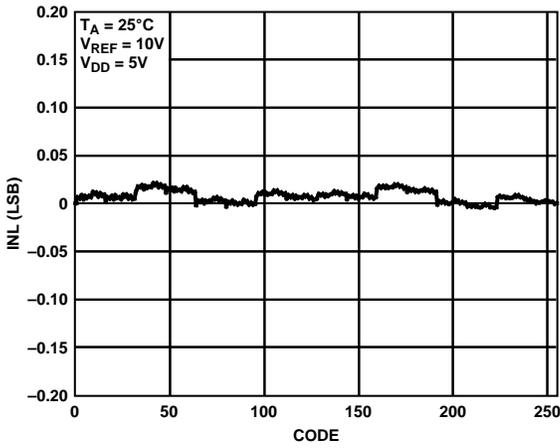
Figure 4. Integral Nonlinearity (INL) vs. Code (8-Bit DAC)
