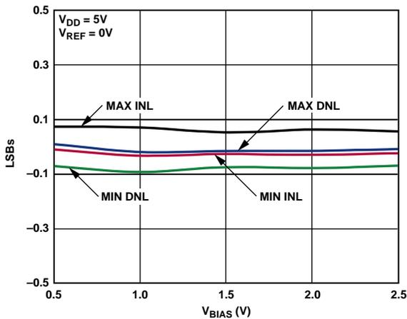
Figure 12. Linearity vs.  $V_{BIAS}$  Voltage Applied to  $I_{OUT2}$
