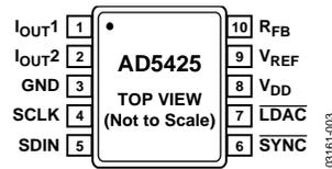
Figure 3. Pin Configuration
