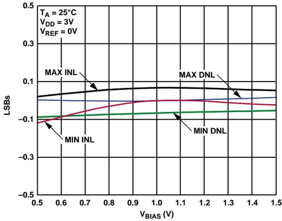
Figure 10. Linearity vs.  $V_{BIAS}$  Voltage Applied to  $I_{OUT2}$
