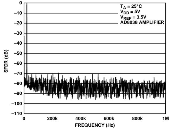
Figure 25. Wideband SFDR, Clock = 2 MHz,  $f_{OUT} = 20$  kHz
