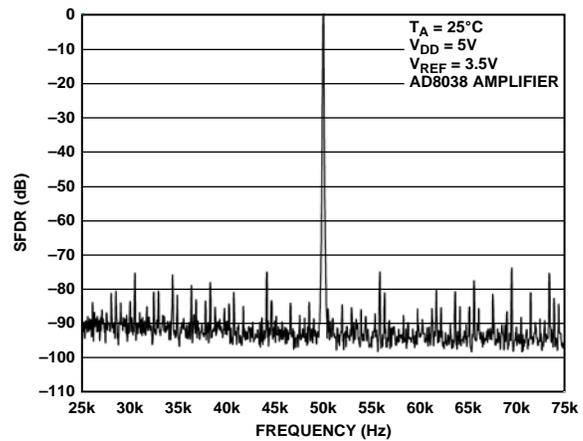
Figure 27. Narrow-Band SFDR, Clock = 2 MHz,  $f_{OUT} = 50$  kHz
