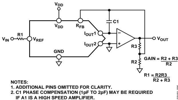
Figure 34. Increasing the Gain of Current Output DAC
