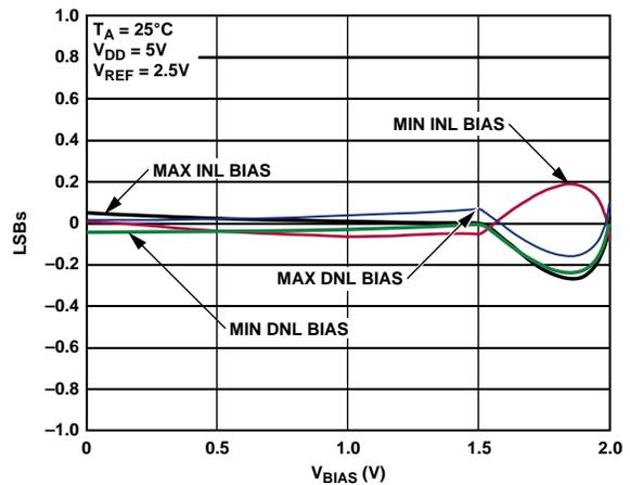
Figure 15. Linearity vs.  $V_{BIAS}$  Voltage Applied to  $I_{OUT2}$
