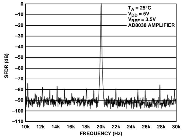
Figure 26. Narrow-Band SFDR, Clock = 2 MHz,  $f_{OUT} = 20$  kHz
