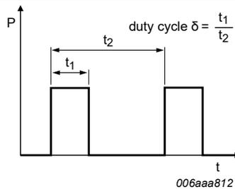
Fig. 17. Duty cycle definition
