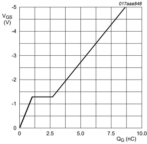
$I_D = -2.8 \text{ A}; V_{DS} = -6 \text{ V}; T_{amb} = 25 \text{ }^\circ\text{C}$
