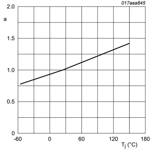
$$a = \frac{R_{DSon}}{R_{DSon(25^\circ C)}}$$
