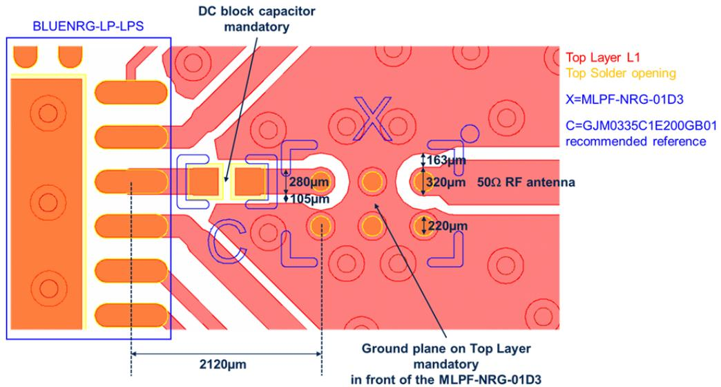
Transmission line between MLPF and antenna is dimensioned to 50 ohms characteristic impedance.
