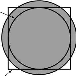
**Figure 16. Footprint - 3 mils stencil - solder mask defined**
