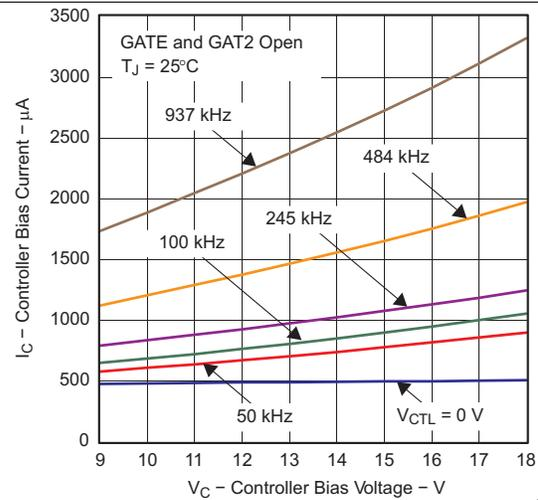
**Figure 9. '754 Controller Bias Current vs Voltage**
