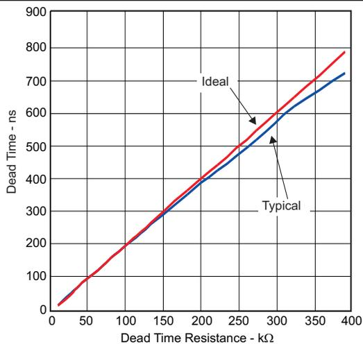
Figure 18. Dead Time vs Dead Time Resistance ( $R_{DT}$ )
