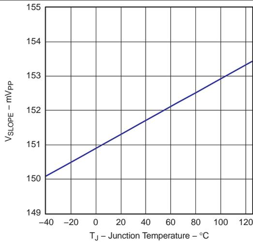
Figure 14. Current Slope Compensation Voltage vs Temperature
