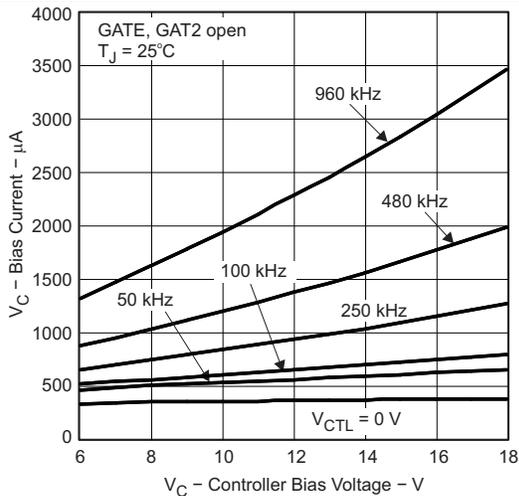
**Figure 10. '756 Controller Bias Current vs Voltage**
