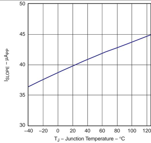
Figure 15. Current Slope Compensation Current vs Temperature
