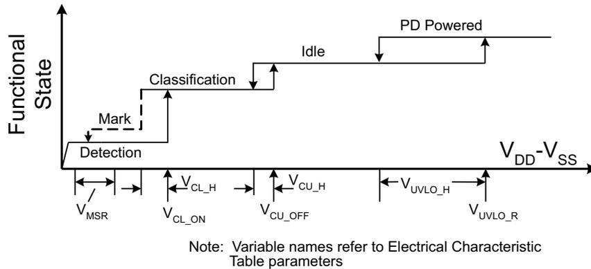
Figure 21. Threshold Voltages
