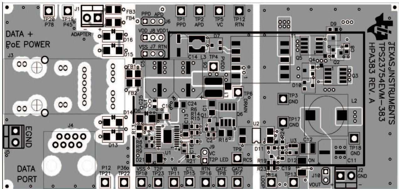
Figure 39. TPS23754EVM-383 EVM Parts Placement and Example Layout
