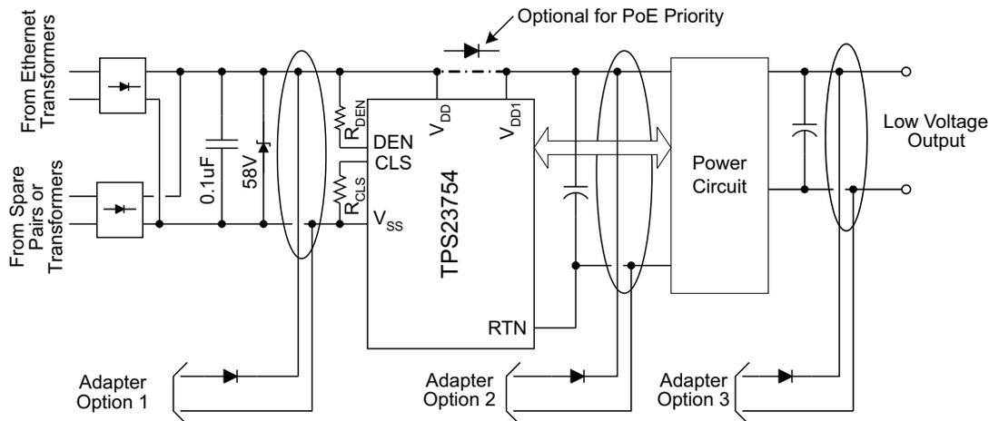
**Figure 26. ORing Configurations**
