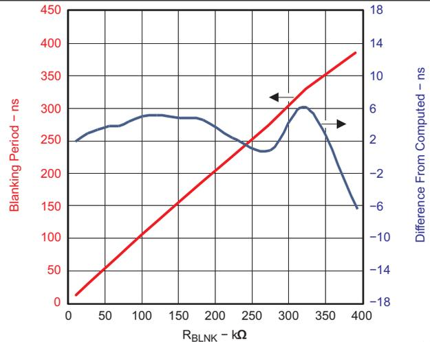
Figure 17. Blanking Period vs Blanking Resistance ( $R_{BLNK}$ )
