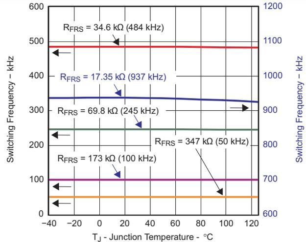
**Figure 11. Switching Frequency vs Temperature**
