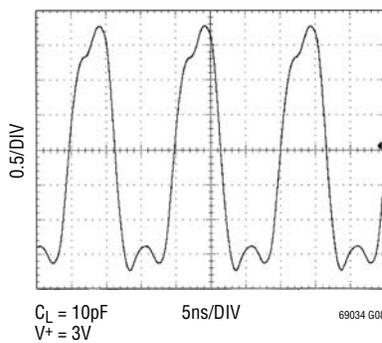
**Output Waveform at 20MHz**
