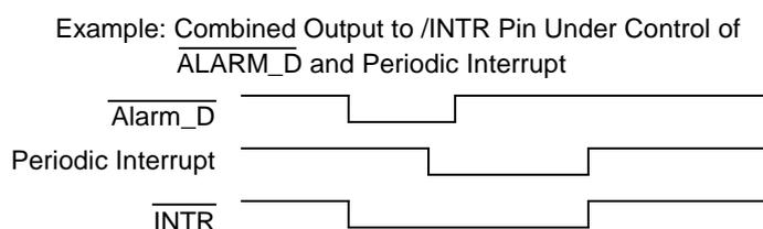
In this event, which type of interrupt signal is output from the  $\overline{\text{INTR}}$  pin can be confirmed by reading the DAFG, and CTFG bit settings in the Control Register 2.
