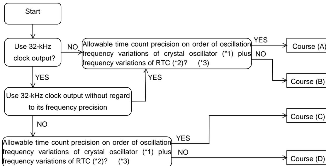
\* 1) Generally, quartz crystal units for commercial use are classified in terms of their center frequency depending on their load capacitance (CL) and further divided into ranks on the order of  $\pm 10$ ,  $\pm 20$ , and  $\pm 50$ ppm depending on the degree of their oscillation frequency variations.
