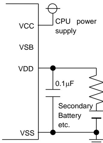
The case of back-up by capacitor or secondary battery (Charging voltage is not equal to CPU power supply voltage)
