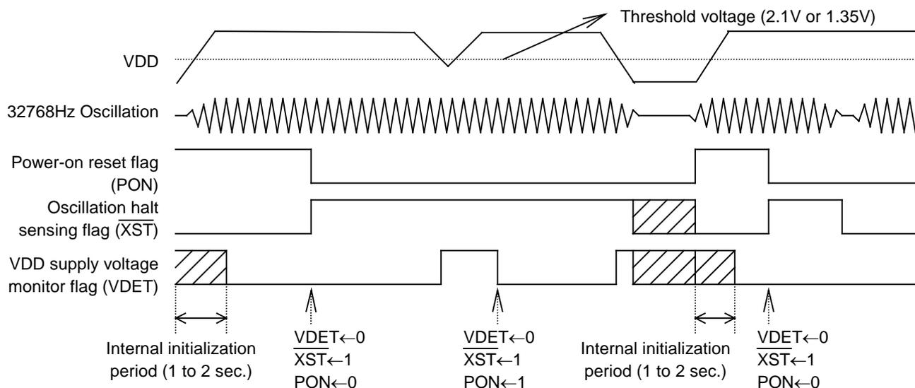
When the PON bit is set to 1 in the control register 2, the DEV, F6 to F0, WALE, DALE,  $\overline{12}/24$ , SCRATCH2, TEST, CT2, CT1, CT0, VDSL, VDET, SCRATCH1, CTFG, WAFG, and DAFG bits are reset to 0 in the oscillation adjustment register, the control register 1, and the control register 2. The PON bit is also set to 1 at power-on from 0 volts.
