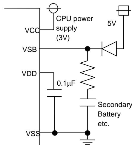
VDD pin cannot be connected to any additional heavy load components such as SRAM. And VDD pin must be connected C2, and C2 should be over 0.1µF.
