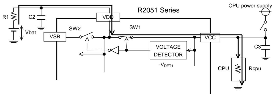
When secondary battery or double layer capacitor connects to VDD pin, after CPU power supply turning off, secondary battery discharges through the root above figure. If R1 is much smaller than CPU impedance (Rcpu), VCC voltage keeps higher than -VDET1, and SW1 keeps on. Therefore R1 must be specified by following formula.
