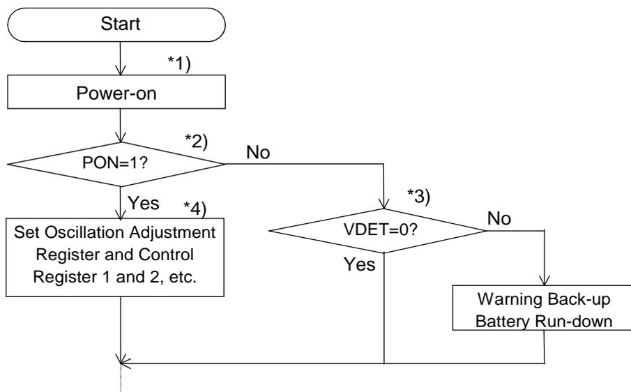
\*1) After power-on from 0 volt, the process of internal initialization require a time span on 1sec, so that access should be done after  $\overline{\text{VDCC}}$  turning to OFF(H).
