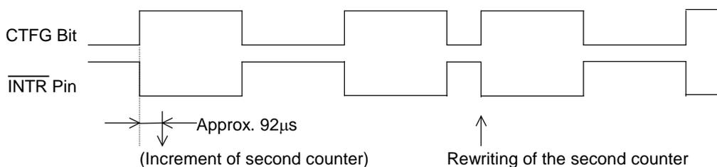
In the pulse mode, the increment of the second counter is delayed by approximately 92  $\mu\text{s}$  from the falling edge of clock pulses. Consequently, time readings immediately after the falling edge of clock pulses may appear to lag behind the time counts of the real-time clocks by approximately 1 second. Rewriting the second counter will reset the other time counters of less than 1 second, driving the  $\overline{\text{INTR}}$  pin low.
