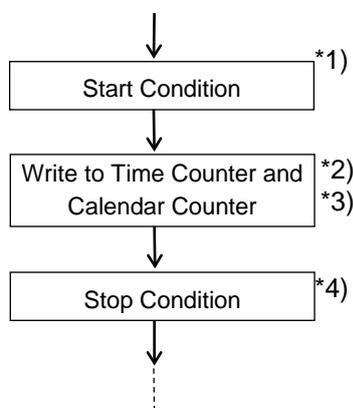
\*1) When writing to clock and calendar counters, do not insert Stop Condition until all times from second to year have been written to prevent error in writing time. (Detailed in "P.37 Data Transmission under Special Condition".
