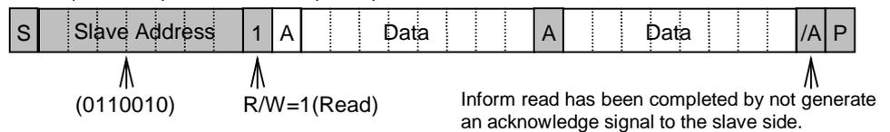
When the transmission direction is to be changed during transmission.
