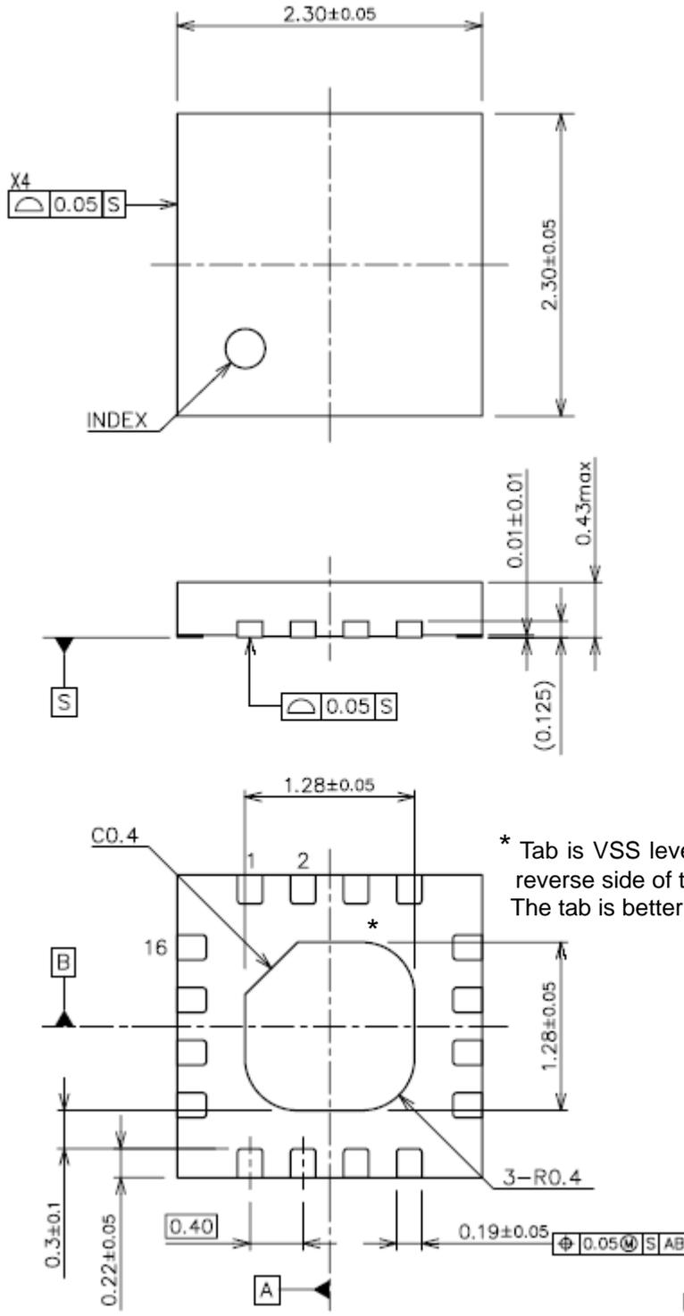
\* Tab is VSS level. (They are connected to the reverse side of this IC.)
