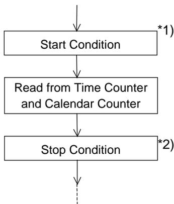
\*1) When reading to clock and calendar counters, do not insert Stop Condition until all times from second to year have been written to prevent error in writing time. (Detailed in "P.37 Data Transmission under Special Condition".
