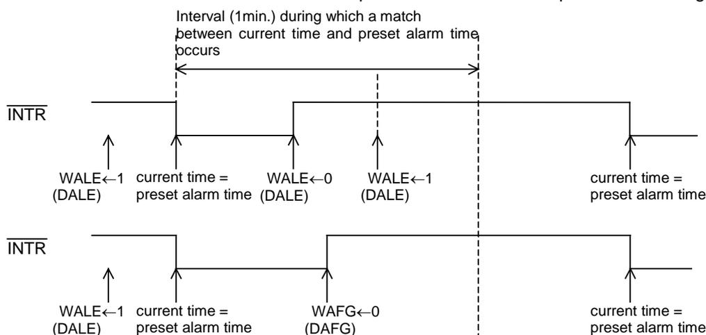
After setting WALE(DALE) to 0, Alarm registers is set to current time, and WALE(DALE) is set to 1,  $\overline{\text{INTR}}$  will be not driven to "L" immediately,  $\overline{\text{INTR}}$  will be driven to "L" at next alarm setting time.
