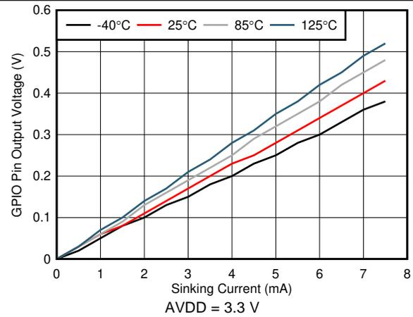
Figure 32. GPIO Pin Output Voltage vs Sinking Current
