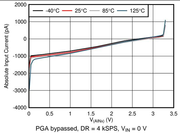
Figure 8. Absolute Input Current vs Absolute Input Voltage
