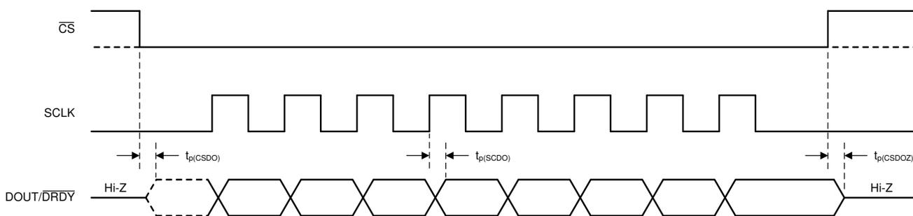
NOTE: Single-byte communication is shown. Actual communication can be multiple bytes.
