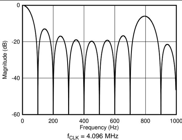
**Figure 55. Digital Filter Frequency Response, Data Rate = 100 SPS**
