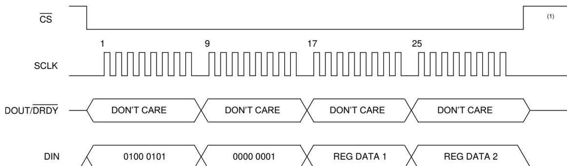
(1)  $\overline{\text{CS}}$  can be set high or kept low between commands. If kept low, the command must be completed.
