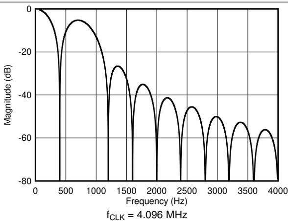
**Figure 57. Digital Filter Frequency Response, Data Rate = 400 SPS**
