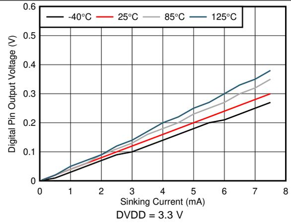
Figure 34. Digital Pin Output Voltage vs Sinking Current
