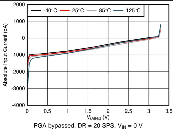
Figure 7. Absolute Input Current vs Absolute Input Voltage
