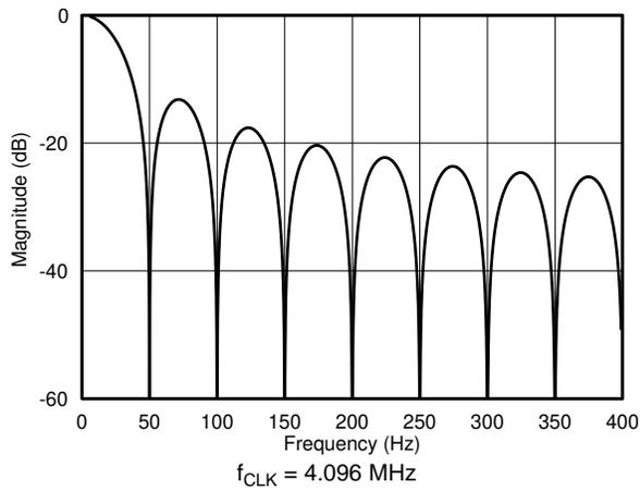
**Figure 53. Digital Filter Frequency Response, Data Rate = 50 SPS**
