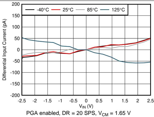
**Figure 13. Differential Input Current vs Differential Input Voltage**
