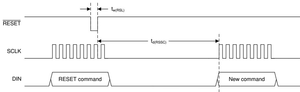
Figure 3.  $\overline{RESET}$  Pin and RESET Command Timing Requirements
