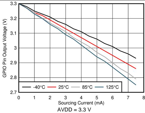
Figure 31. GPIO Pin Output Voltage vs Sourcing Current
