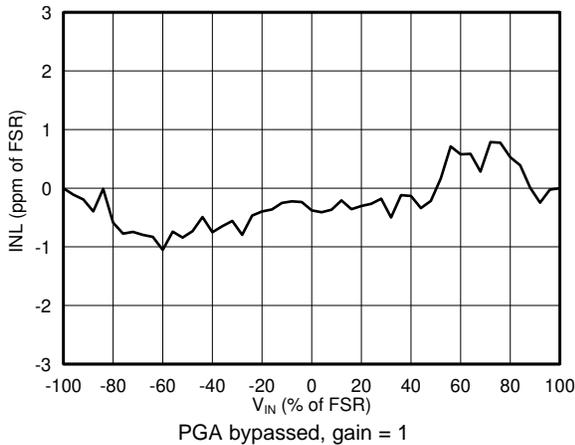
**Figure 15. INL vs Differential Input Voltage**
