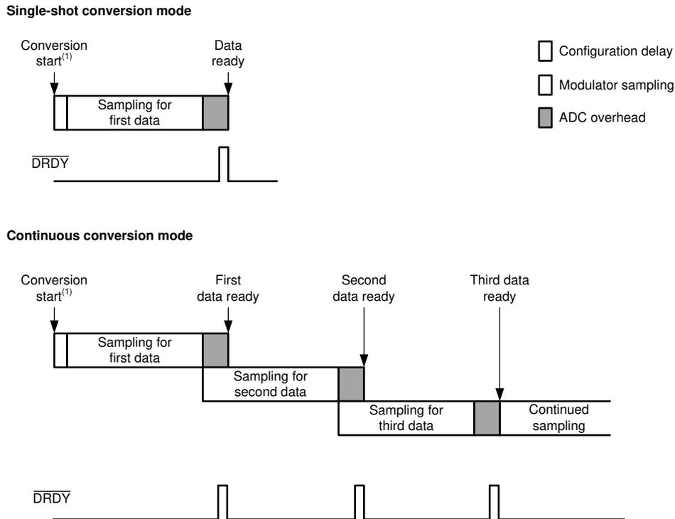
(1) Conversions start at the rising edge of the START/SYNC pin or on the seventh SCLK falling edge for a START command.
