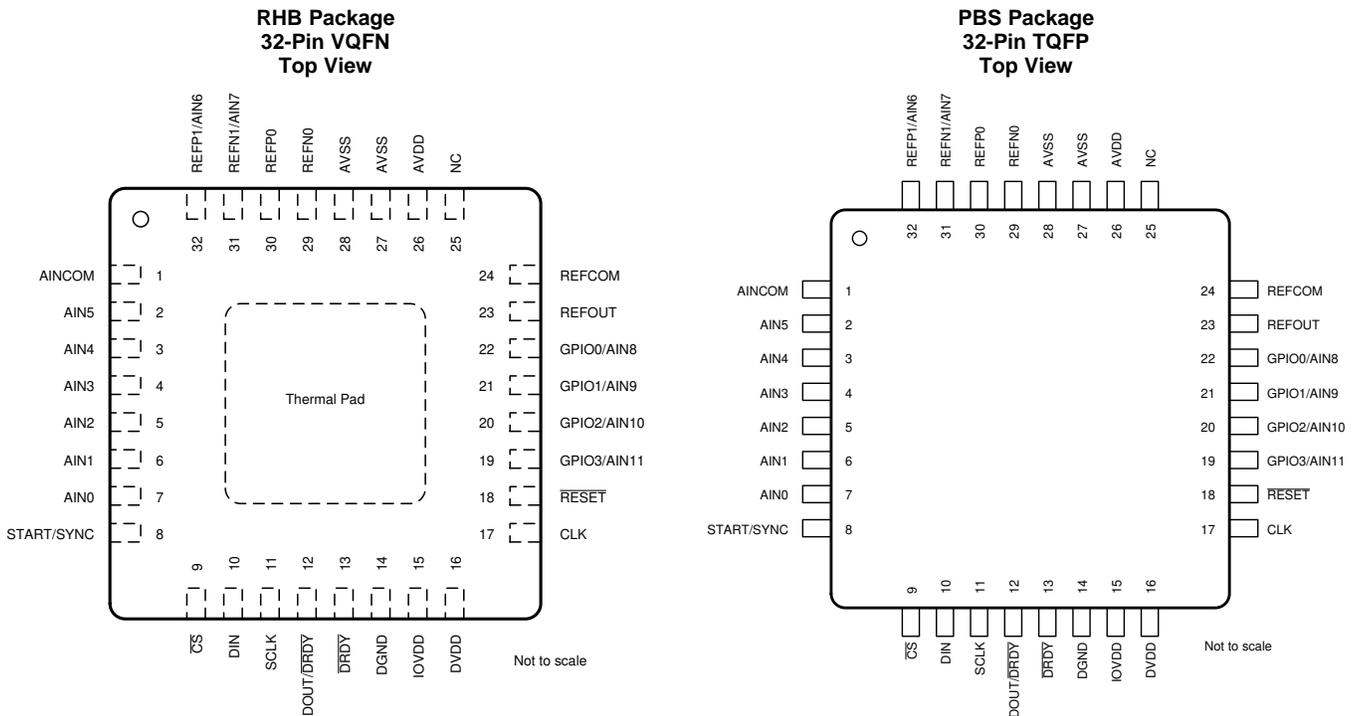
NOTE: The analog input functions (AIN6–AIN11) are not available on pins 19 to 22, 31, and 32 for the ADS114S06B.
