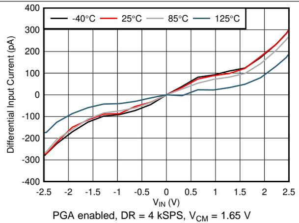
**Figure 14. Differential Input Current vs Differential Input Voltage**
