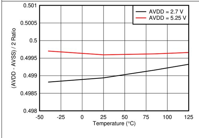
Figure 29. VBIAS Voltage  $[(AVDD - AVSS) / 2]$  vs Temperature
