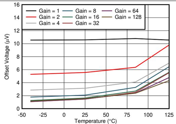
**Figure 18. Offset Voltage vs Temperature**
