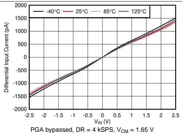
Figure 12. Differential Input Current vs Differential Input Voltage
