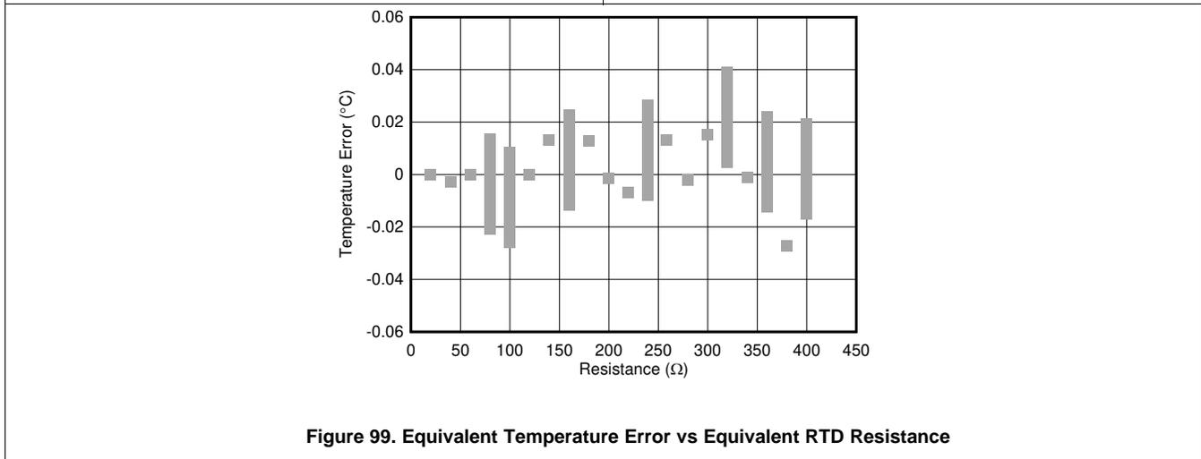
Figure 99. Equivalent Temperature Error vs Equivalent RTD Resistance
