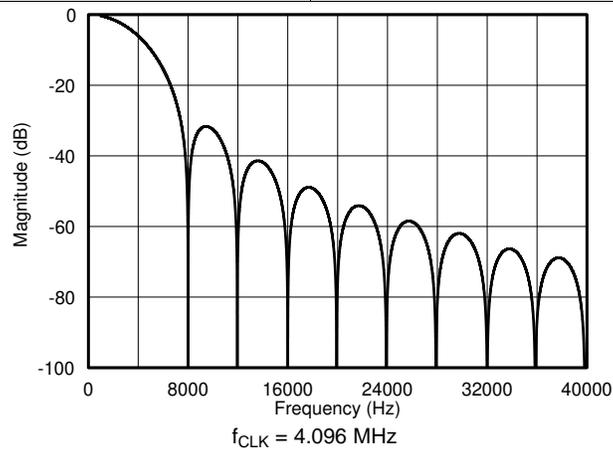
Figure 61. Digital Filter Frequency Response, Data Rate = 4 kSPS
