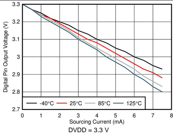
Figure 33. Digital Pin Output Voltage vs Sourcing Current
