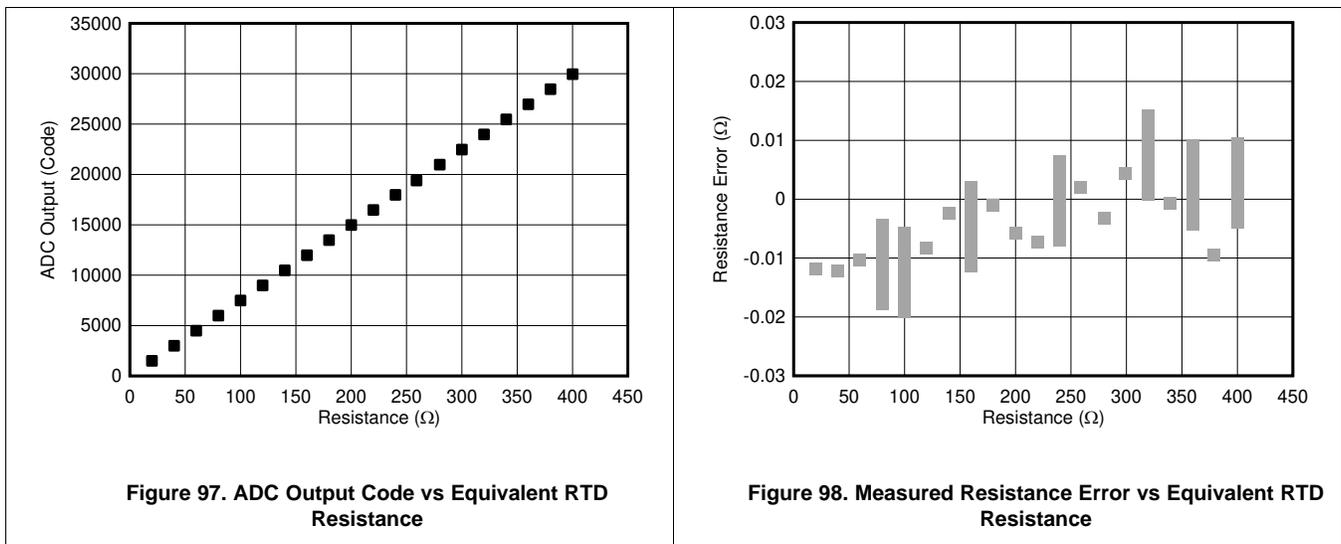
Figure 97. ADC Output Code vs Equivalent RTD Resistance
