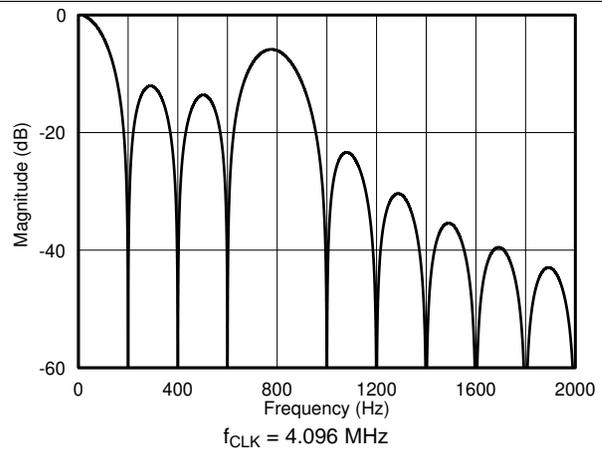
**Figure 56. Digital Filter Frequency Response, Data Rate = 200 SPS**
