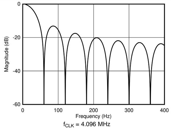
**Figure 54. Digital Filter Frequency Response, Data Rate = 60 SPS**
