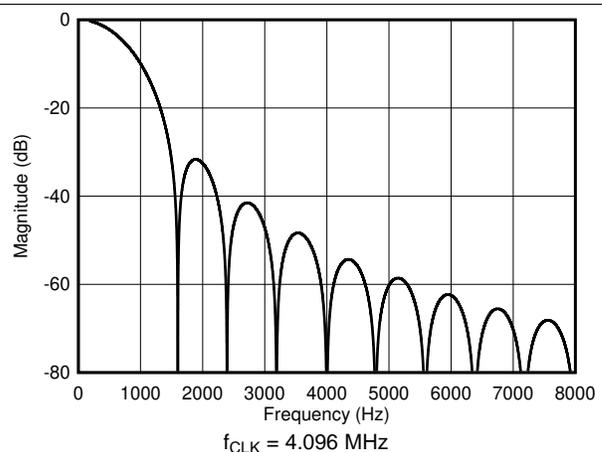
**Figure 58. Digital Filter Frequency Response, Data Rate = 800 SPS**
