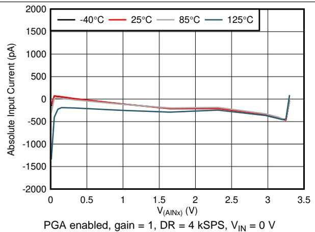
Figure 10. Absolute Input Current vs Absolute Input Voltage
