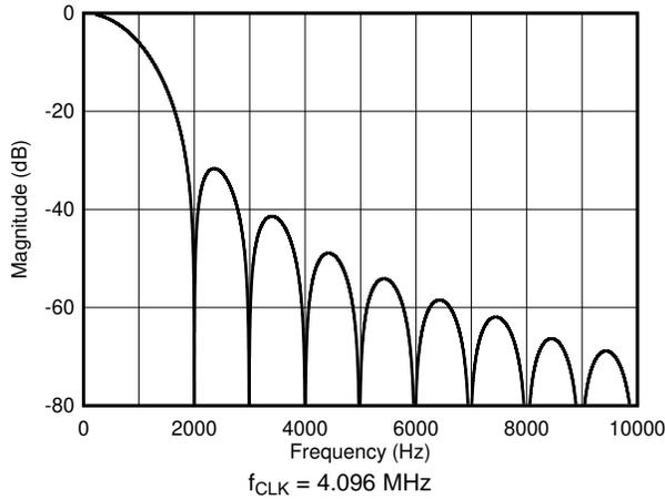
Figure 59. Digital Filter Frequency Response, Data Rate = 1 kSPS
