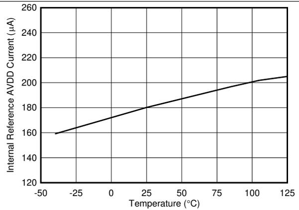
Figure 38. Internal Reference AVDD Current vs Temperature
