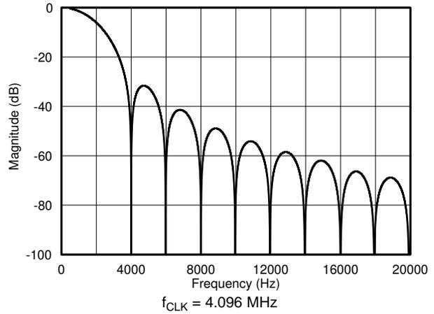
Figure 60. Digital Filter Frequency Response, Data Rate = 2 kSPS
