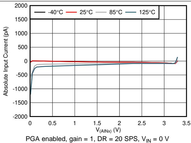
Figure 9. Absolute Input Current vs Absolute Input Voltage
