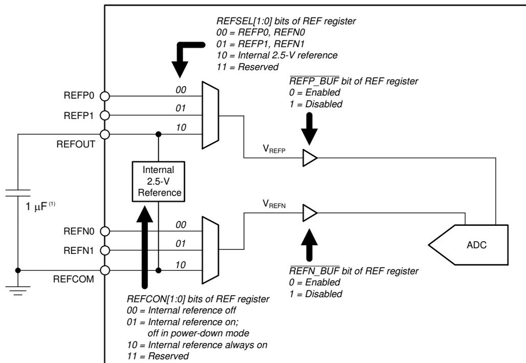
(1) The internal reference requires a minimum 1-μF capacitor connected from REFOUT to REFCOM.
