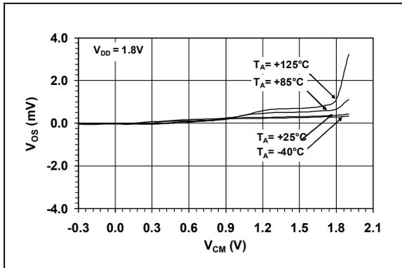
**FIGURE 2-8:** Input Offset Voltage vs. Common-mode Input Voltage.
