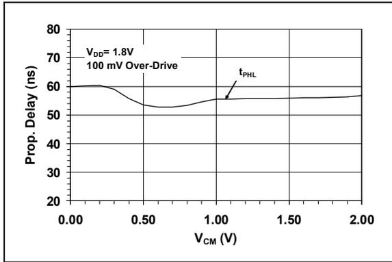
**FIGURE 2-31:** Propagation Delay vs. Common-mode Input Voltage.
