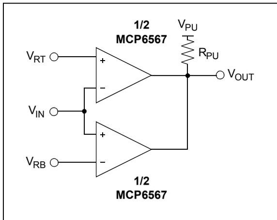
**FIGURE 4-13:** *Windowed Comparator.*
