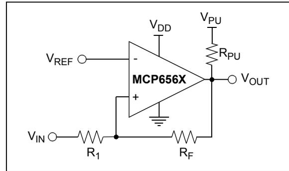
**FIGURE 4-4:** Non-Inverting Circuit with Hysteresis for Single-Supply.
