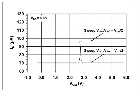
**FIGURE 2-18:** Quiescent Current vs. Common-mode Input Voltage.
