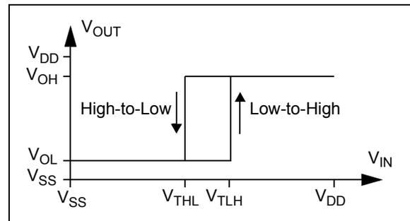
**FIGURE 4-5:** Hysteresis Diagram for the Non-Inverting Circuit.
