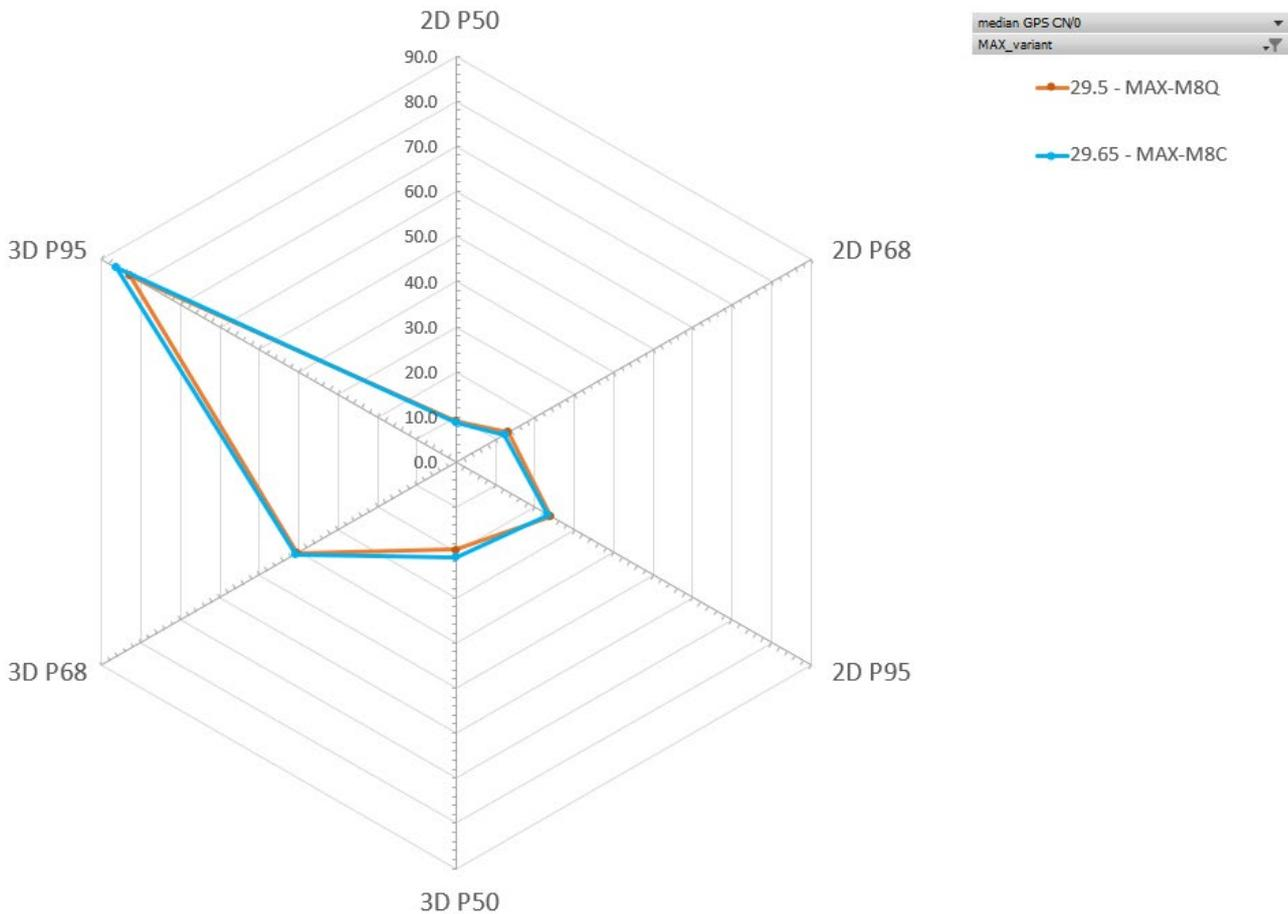
**Figure 6: Position error in meters for MAX-M8C and MAX-M8Q in percentiles at 29.5 dBHz in urban canyon (default mode: GPS and GLONASS including QZSS, SBAS)**
