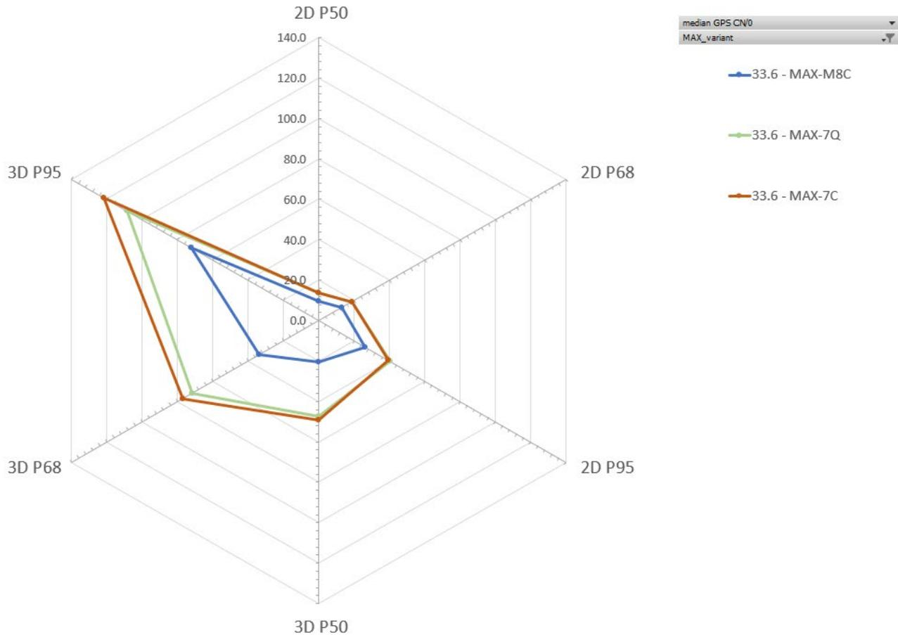
**Figure 16: Position error in meters for MAX-M8C, MAX-7Q and MAX-7C in percentiles at 33.6 dBHz in an urban canyon**
