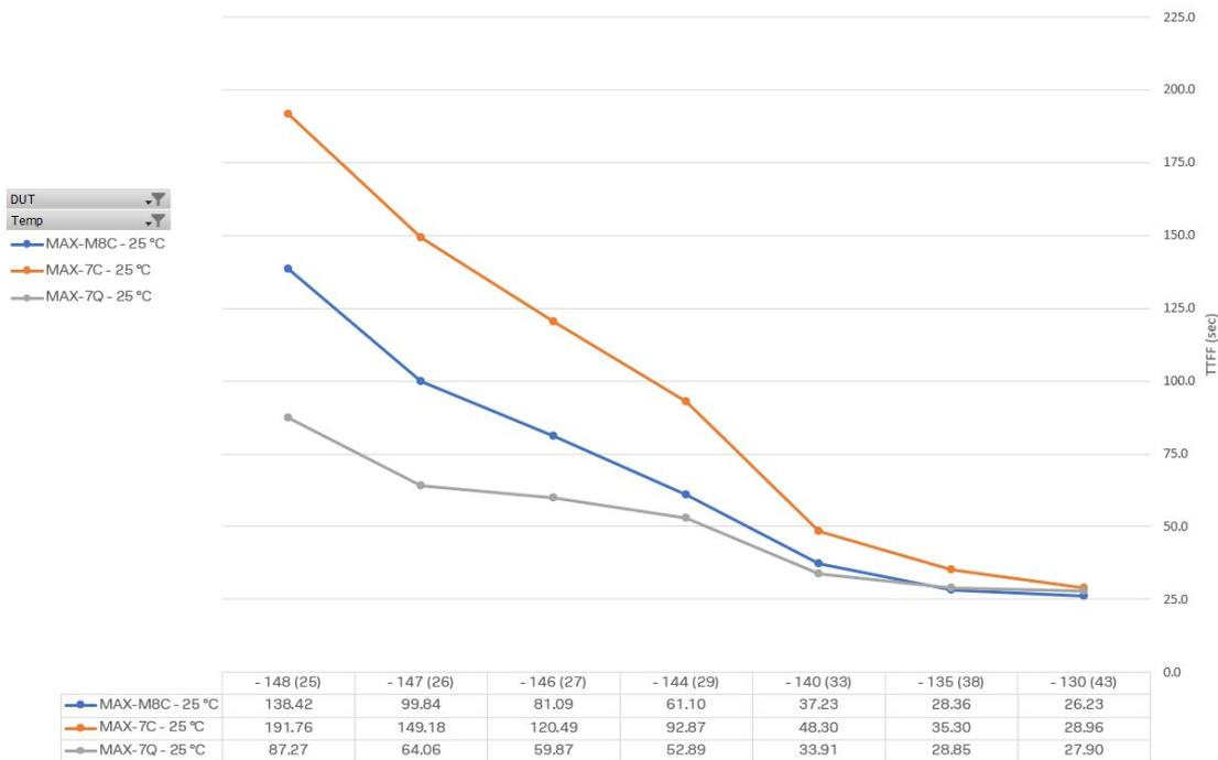
**Figure 11: TTFF vs. signal power in dBm and equivalent C/N0 inside parenthesis for MAX-M8C, MAX-7Q and MAX-7C during cold starts<sup>24</sup> (default configuration)**
