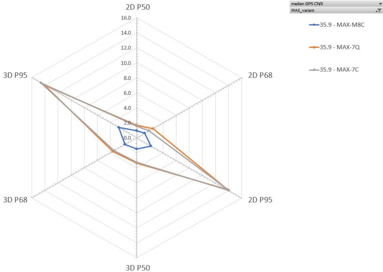
**Figure 17: Position error in meters for MAX-M8C, MAX-7Q and MAX-7C in percentiles at 35.9 dBHz in a highway**
