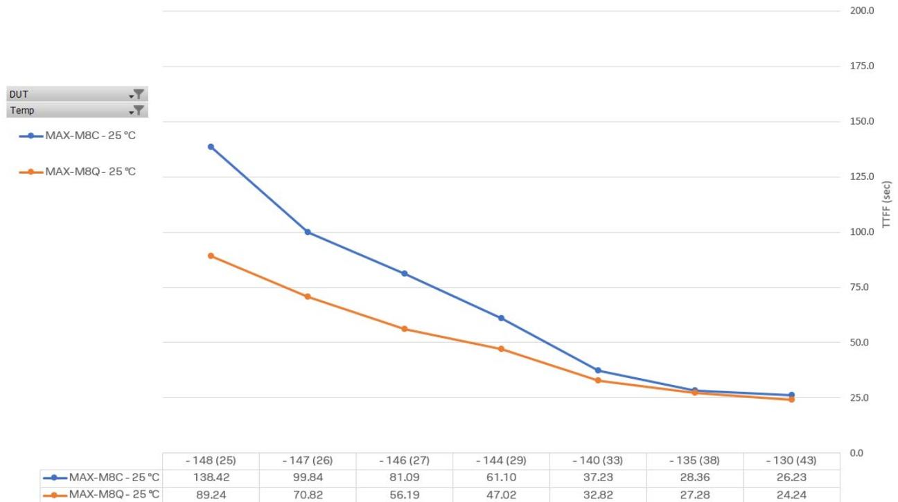
**Figure 2: TTFF vs. signal power in dBm and equivalent C/N0 inside parenthesis for MAX-M8Q and MAX-M8C during cold starts<sup>7</sup> (default mode: GPS & GLONASS including QZSS, SBAS)**
