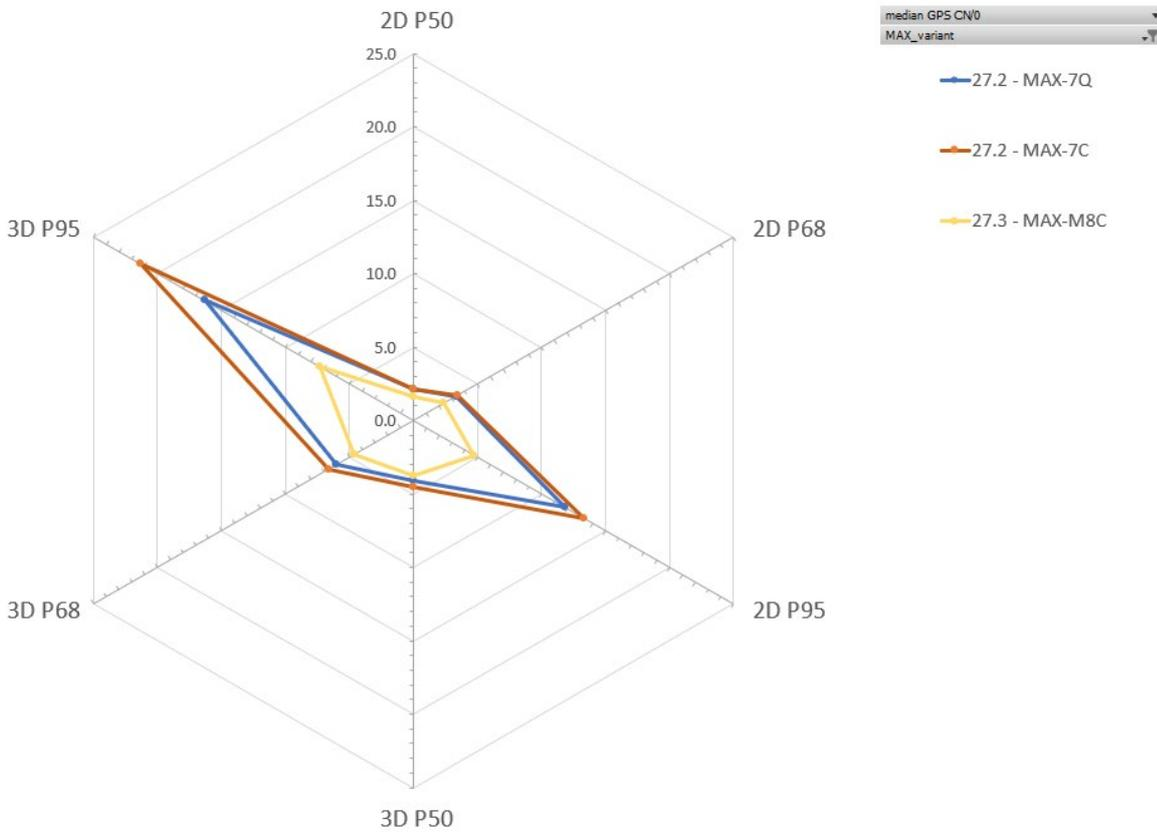
Figure 13: Position error in meters for MAX-M8C, MAX-7Q and MAX-7C in percentiles at 27.2 dBHz in a rural area
