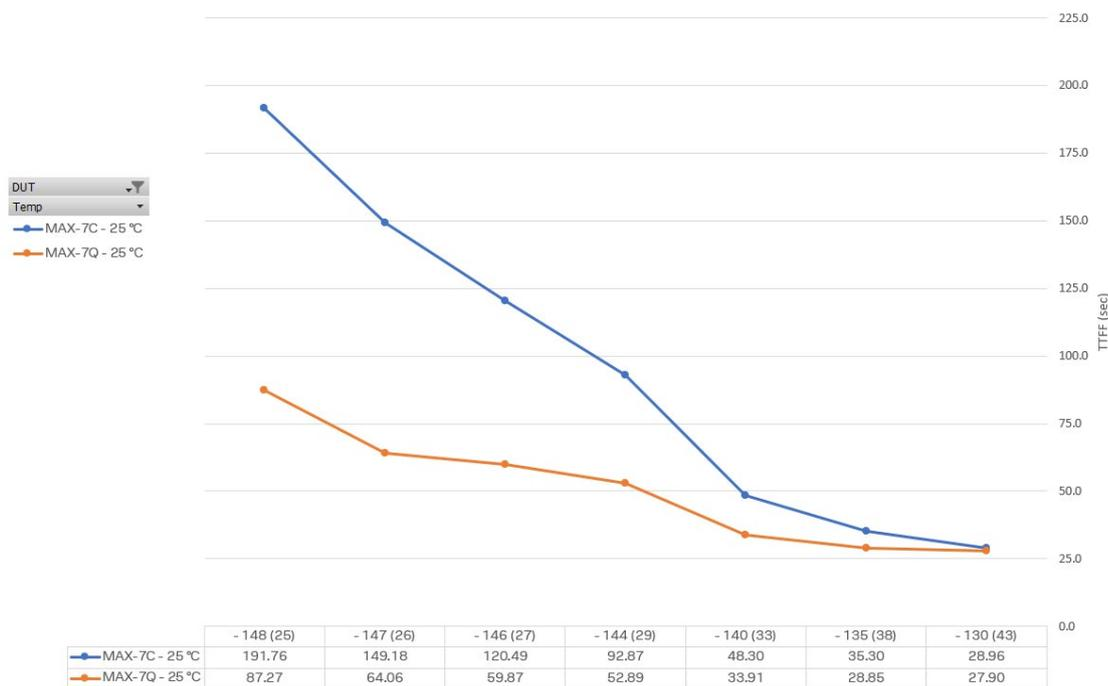
Figure 10: TTFF vs. signal power in dBm and equivalent C/N0 inside parenthesis for MAX-7Q and MAX-7C during cold starts<sup>18</sup>
