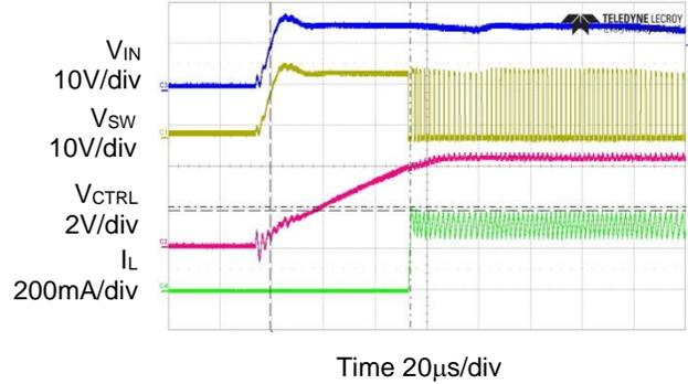
**PWM Dimming (100Hz, Duty=50%)**
