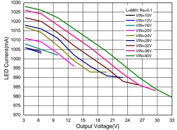
**LED Current vs. Output Voltage**
