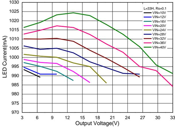
**LED Current vs. Output Voltage**
