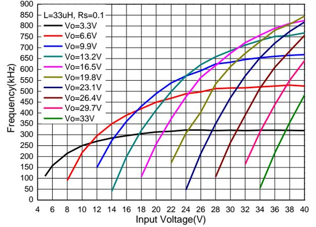
**Operating Frequency vs. Input Voltage**
