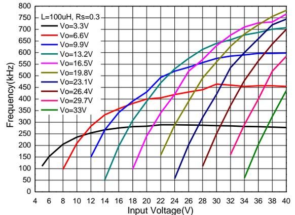
**Typical Performance Characteristics** (continued) (@T<sub>A</sub> = +25°C, V<sub>IN</sub> = 16V, unless otherwise specified.)
