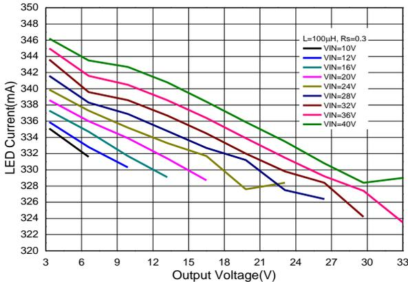
**LED Current vs. Output Voltage**
