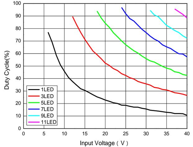
**Performance Characteristics** (@ $V_{IN} = 16V$ , 3LEDs,  $R_S = 0.3\Omega$ ,  $L = 47\mu H$ ,  $T_A = +25^\circ C$ , unless otherwise specified.)
