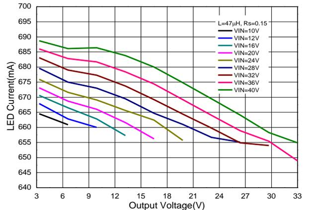
**Typical Performance Characteristics** (continued) (@T<sub>A</sub> = +25°C, V<sub>IN</sub> = 16V, unless otherwise specified.)
