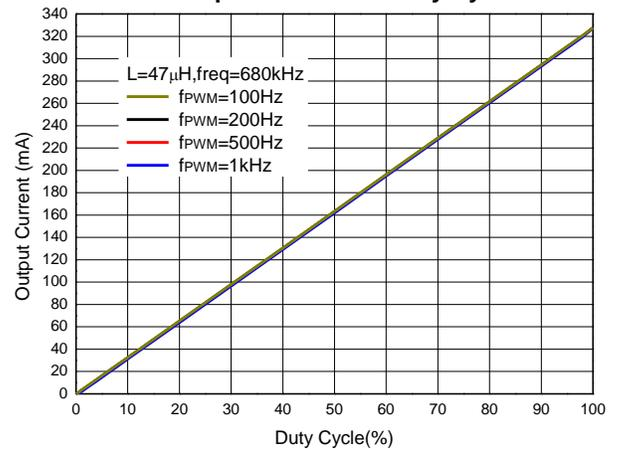
**Typical Performance Characteristics** (continued) (@ $T_A = +25^\circ\text{C}$ ,  $V_{IN} = 16\text{V}$ , unless otherwise specified.)
