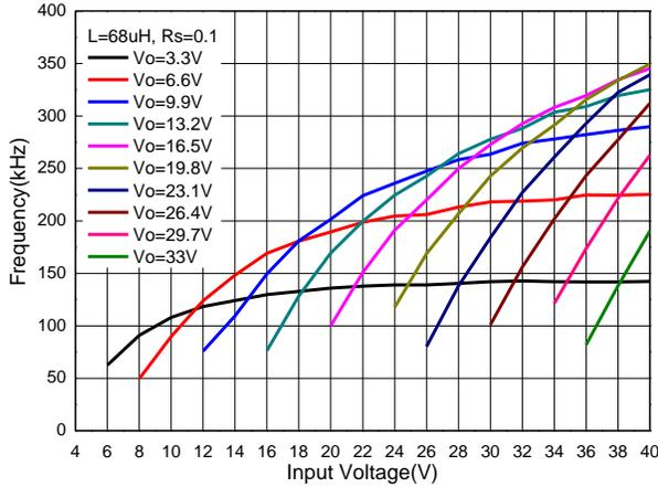
**Operating Frequency vs. Input Voltage**
