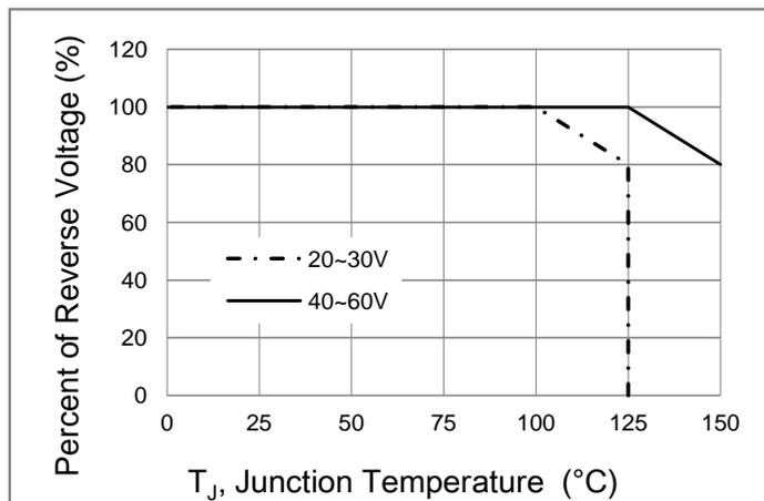
**Fig.5 Operating Temperature Derating Curve**
