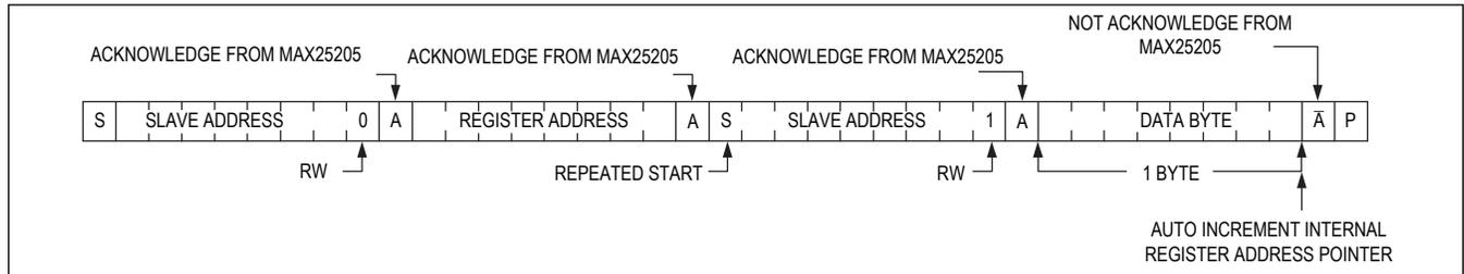
Figure 8. Reading 1 Byte of Indexed Data
