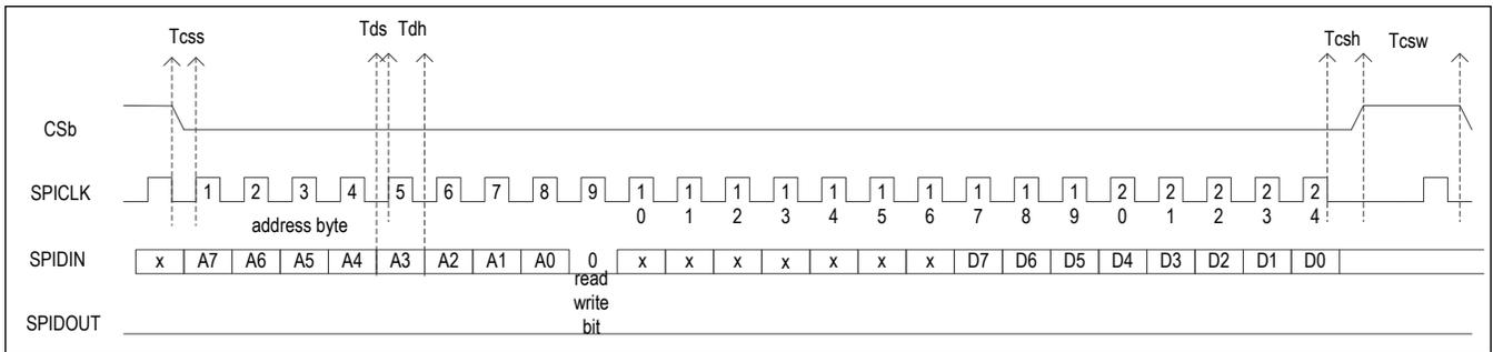
Figure 10. SPI Write
