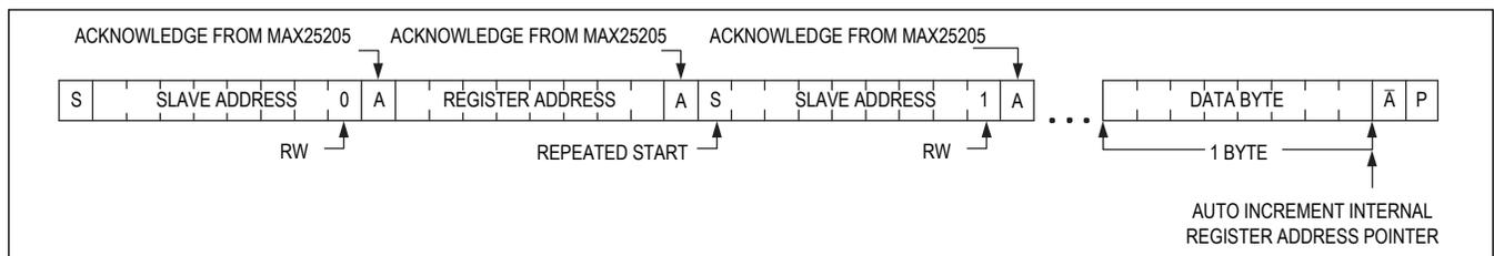
Figure 9. Reading n Bytes of Indexed Data
