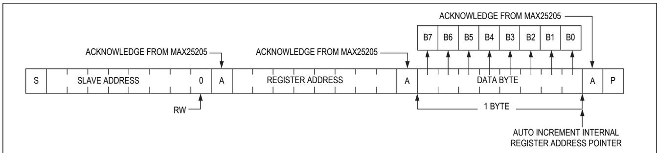
Figure 6. Write 1 Byte
