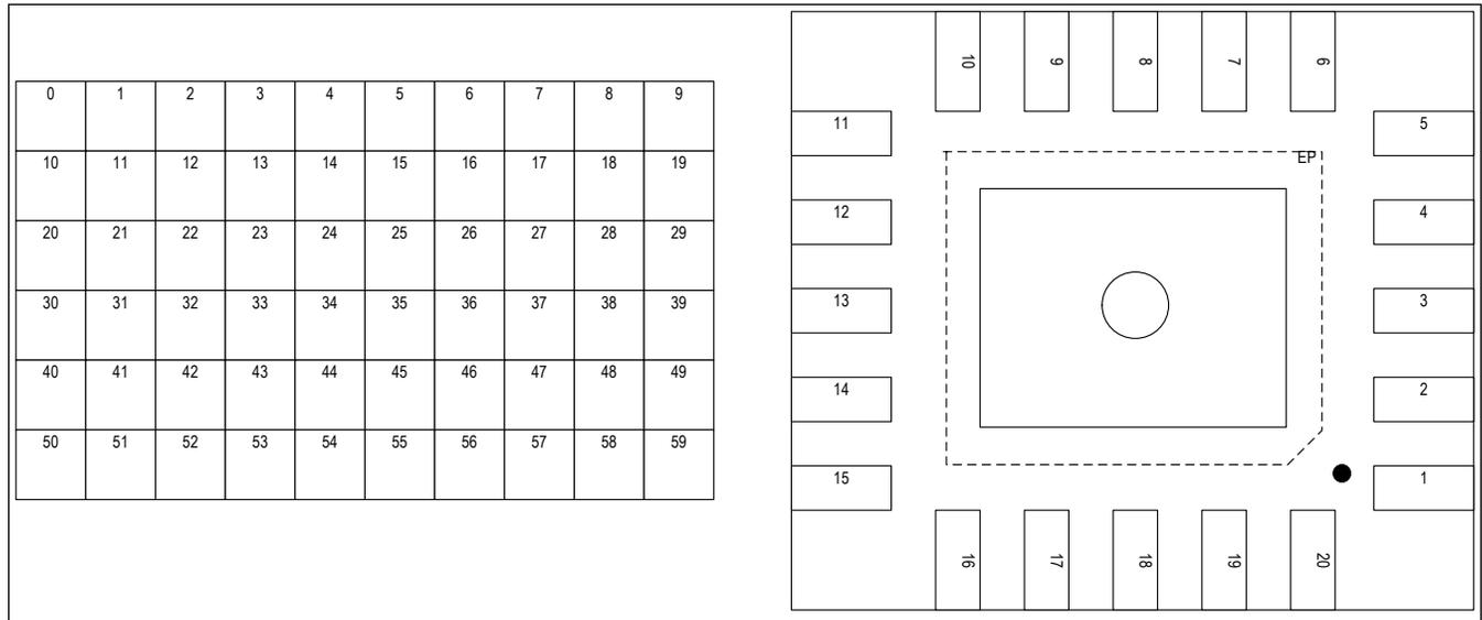
Figure 3. Array Orientation Relative to Pin 1
