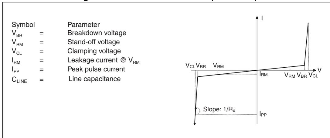
**Table 2. Electrical characteristics (values,  $T_{amb} = 25\text{ }^{\circ}\text{C}$ )**
