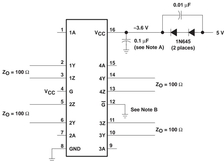
NOTE A: Place a 0.1  $\mu\text{F}$  Z5U ceramic, mica or polystyrene dielectric, 0805 size, chip capacitor between  $V_{CC}$  and the ground plane. The capacitor should be located as close as possible to the device terminals.
